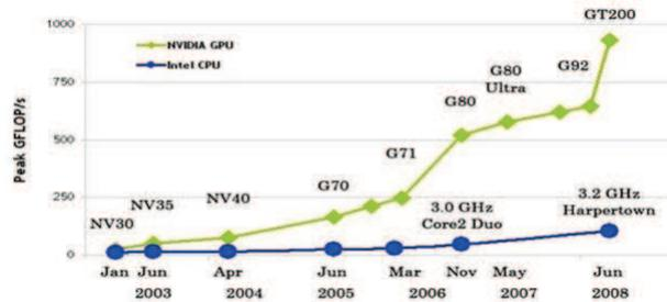
Figure 1: Performance growth of NVIDIA's GPUs vs Intels CPUs [5]
