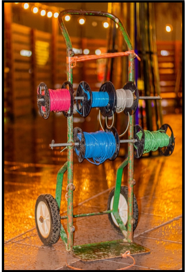
Photograph 43: For as long as I can remember my dad has had this dolly, or diablito in Valley slang. It is a mexicanada because the 10 nuts welded to its frame allow it to act as a wire rack, used when wiring a house/building.
