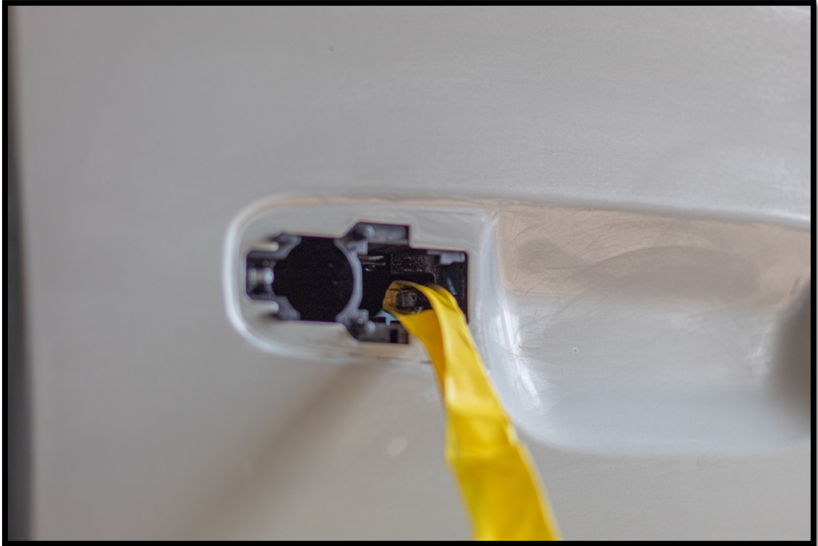
Photograph 25: Painter's tape is folded and then used to hook the trigger in car door, you then pull on the tape to open it when the handle is taken off
