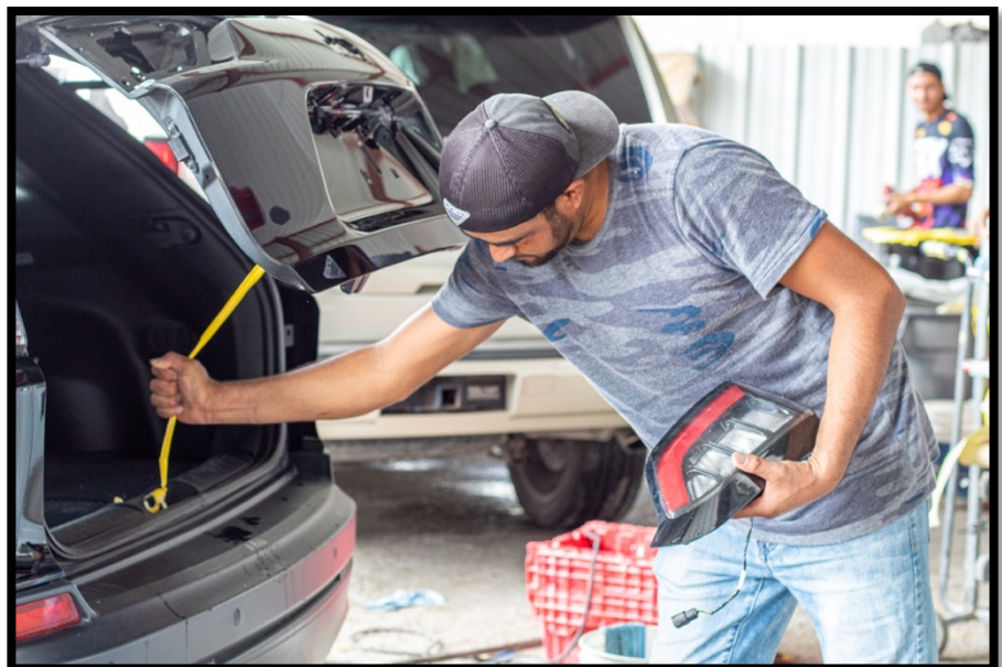
Photograph 20: Hugo shows me how the tape holds the trunk open at an angle so he can work on it comfortably
