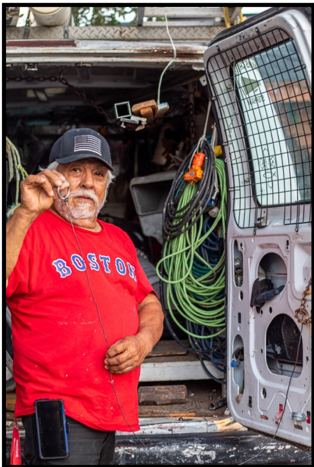
Photograph 37: To open the back door he has to pull the ring from the door on the side, the ring is attached to a chain on the back door that engages the trigger.
