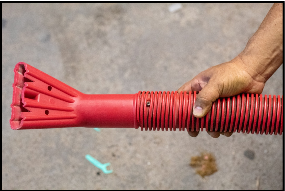
Photograph 93: In his carwash people would often steal the vacuum head, to prevent this he screwed it on.
