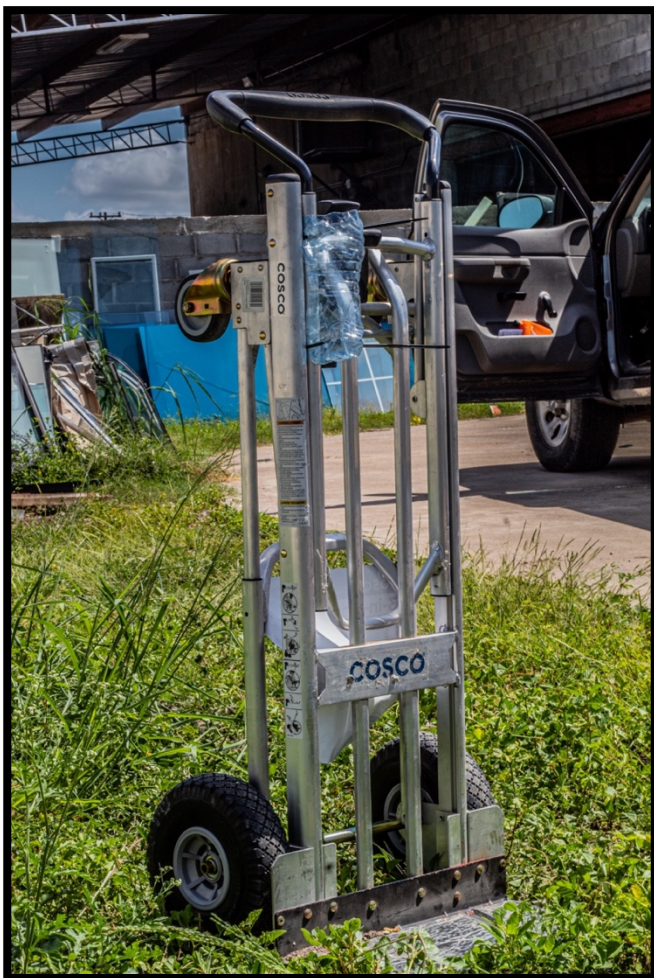
Photograph 56: Dolly has plastic water bottle cut in half zip tied to it, this is used to hold welding rods or other miscellaneous tools.
