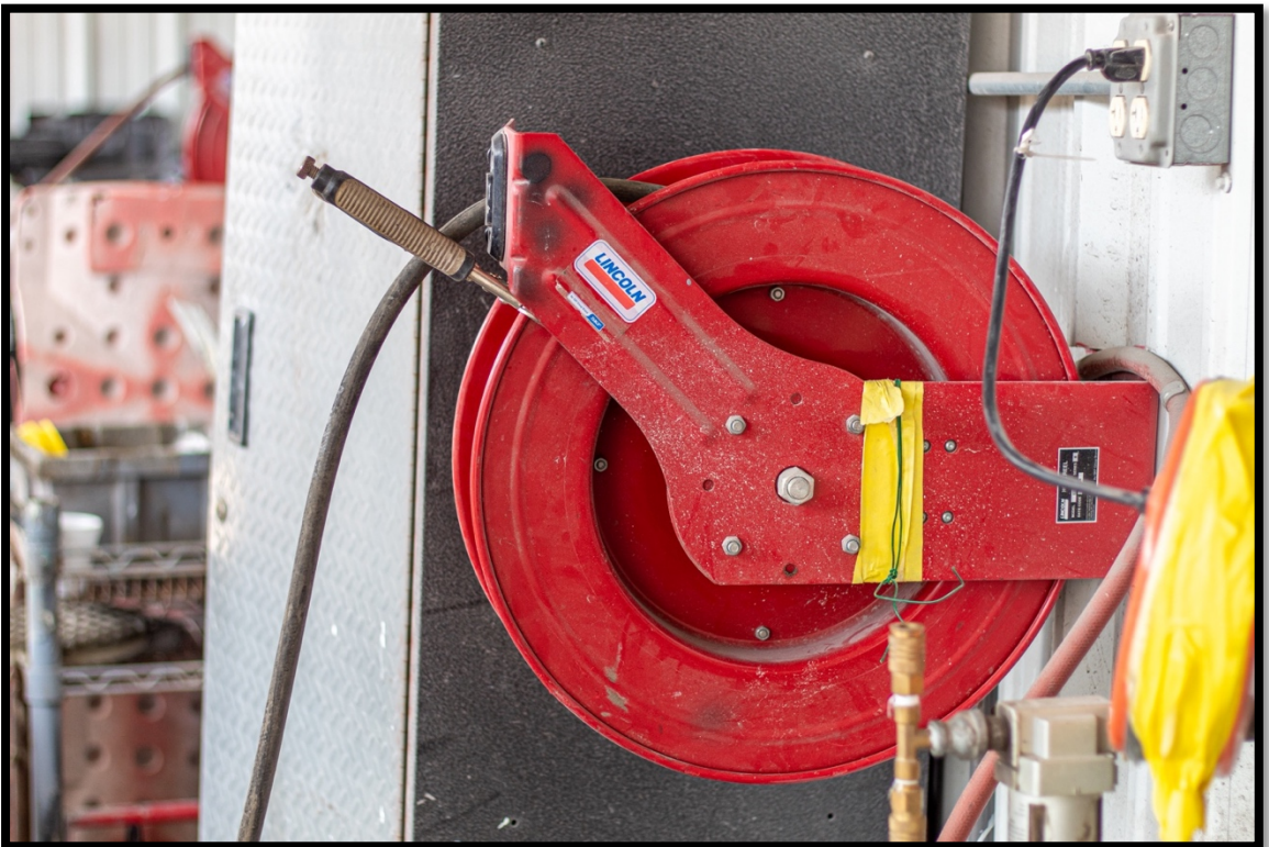
Photograph 24: The spring-loaded hose reel in the wall stopped locking when it was fully extended, the hose would go right back in, to solve this the workers in the autobody shop tighten an adjustable wrench that keeps it from going back in
