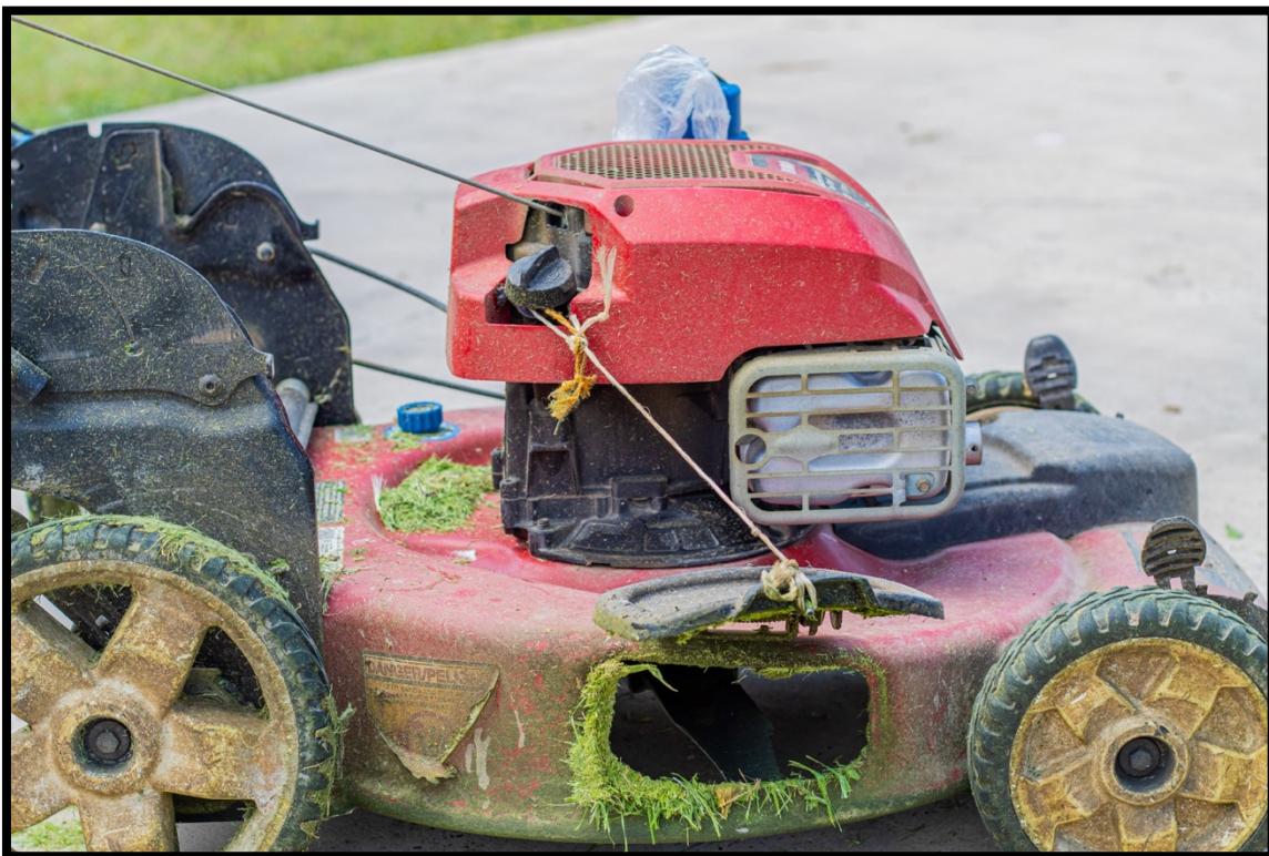
Photograph 75: To let the grass fall out and not get stuck on the blades he permanently opens the side flap with a string. This mexicanada allows him to push with ease and get the job done much faster but it comes with a risk as it can send rocks flying.
