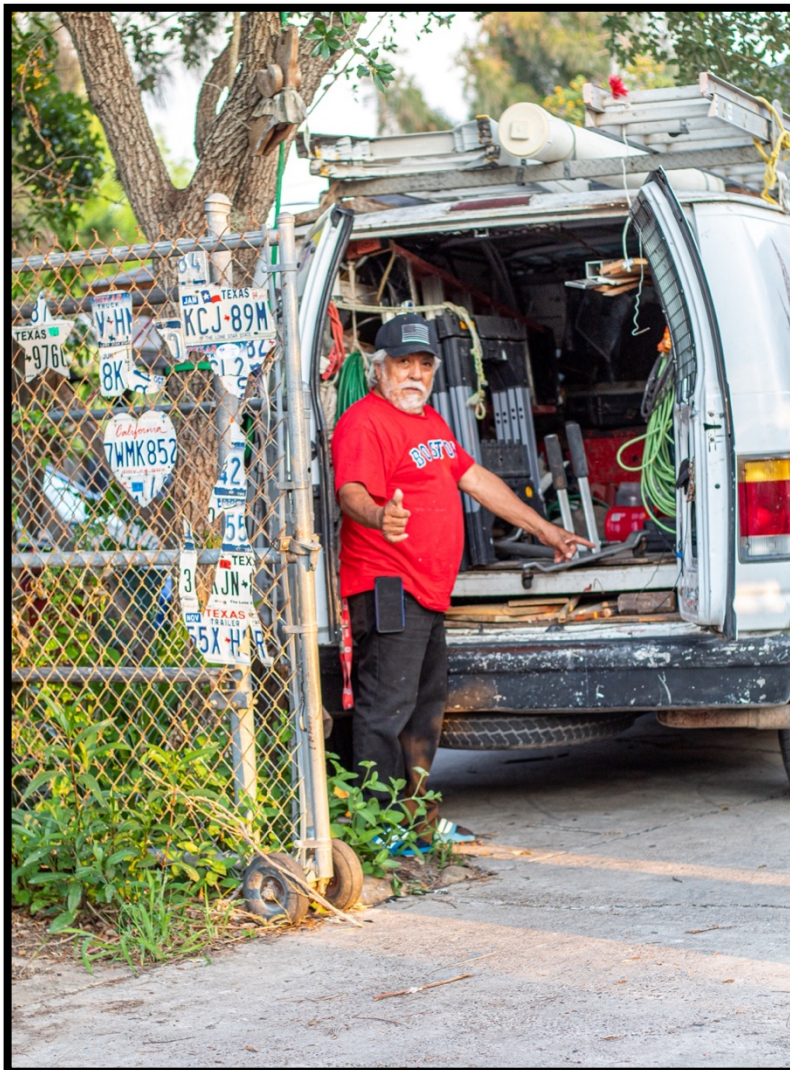
Photograph 36: Tio Lolo shows me his mexicanada, a second level in his work van. That he uses to store sensitive material like sheetrock wall. Allows him to protect it and carry even more things above it.
