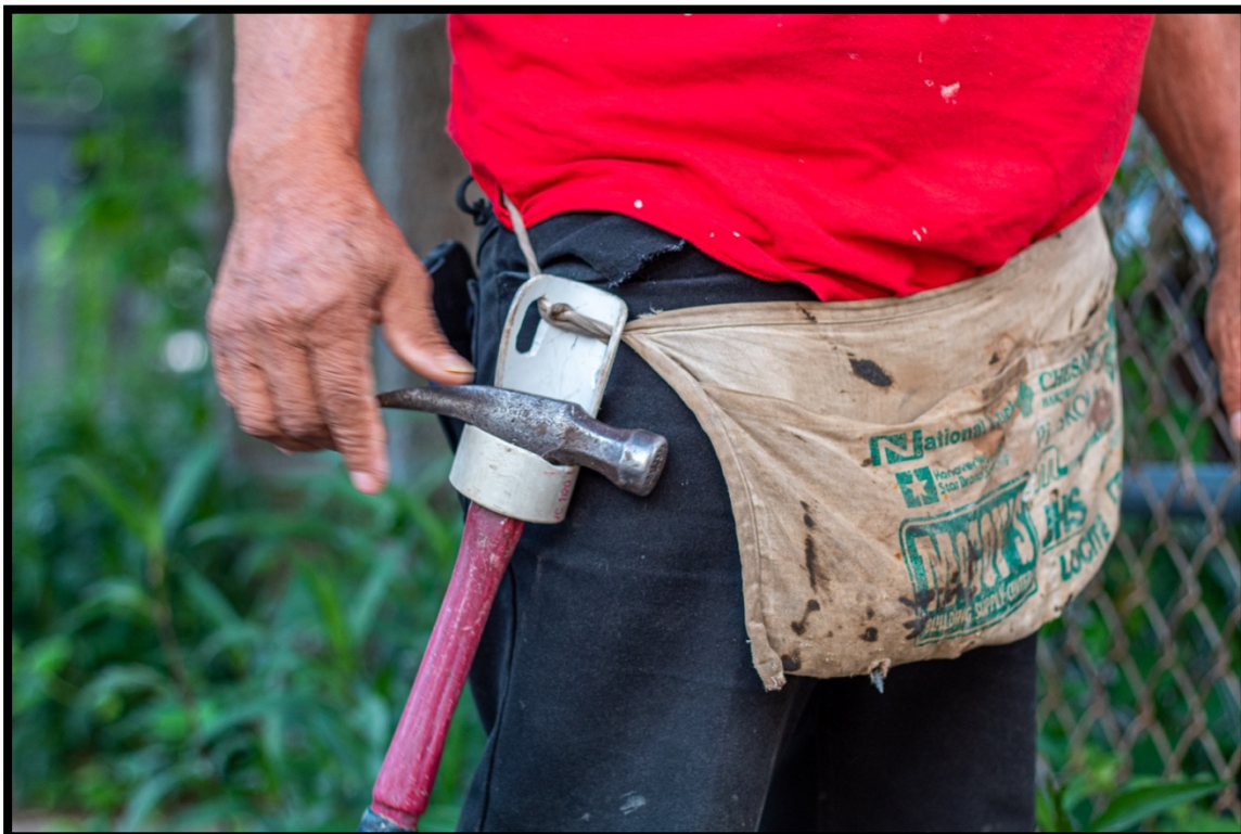
Photograph 38: When he started carpentry work, he wanted a leather pouch, but they were expensive. He made his own hammer holster from a piece of PVC pipe and used it with the apron that he got for free at hardware stores when you bought a box o nails.
