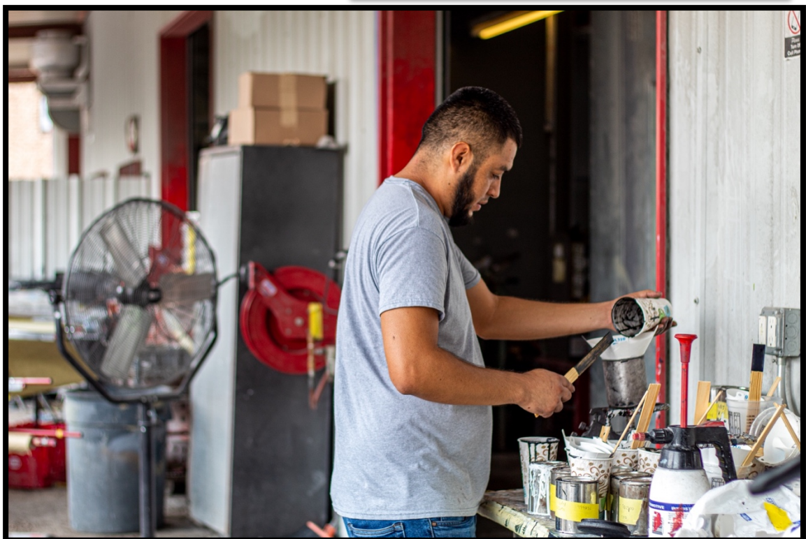
Photograph 22: Mixing and pouring paint into spray gun using coffee cups
