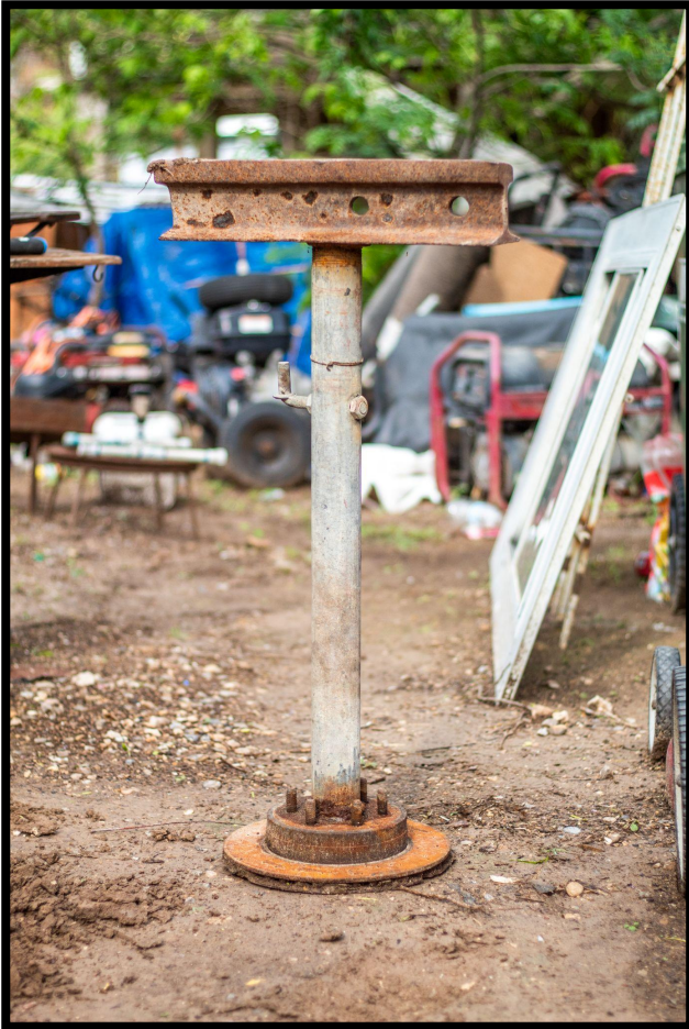
Photograph 17: Luis's Mexicanada is a blacksmith's anvil, used to bend metals over it. This one is made from an old train track, fence post, and an old wheel hub.
