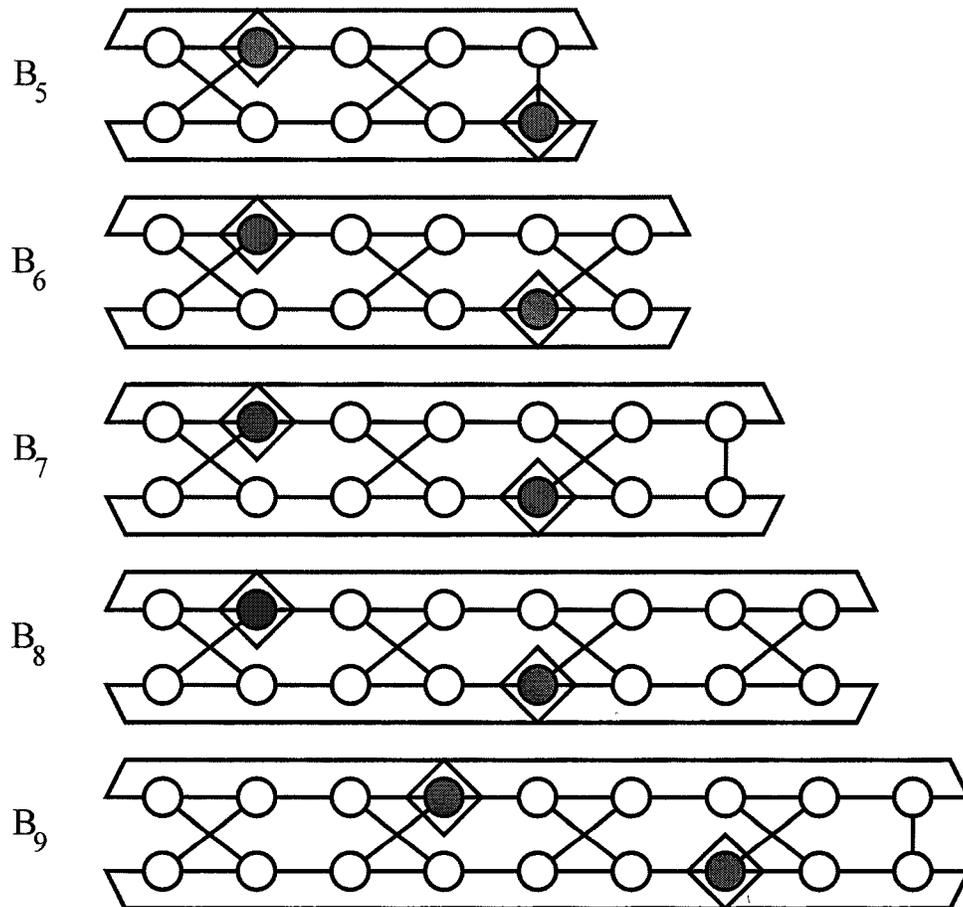
Figure 12: Worst-case graphs and minimal power dominating sets thereon
