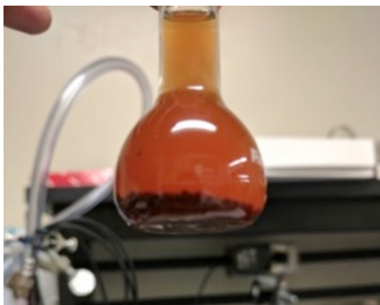
Figure 33. A partially suspended 0.005 M PyVEDOT solution in 0.1 M TBAP in \text{CH}_3\text{CN} electrolyte solution
