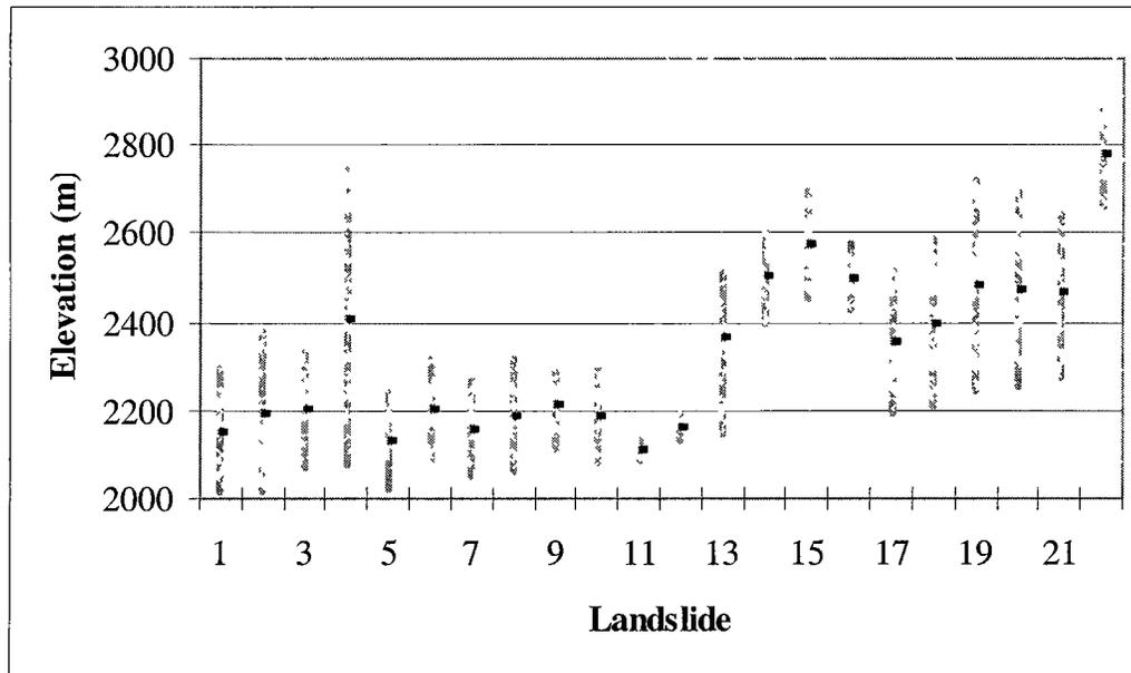
Figure 8. Elevation of the landslides. The top of each line marks the elevation at the head of the landslide, and bottom of the line is the landslide toe. The black dot marks the mean elevation.
