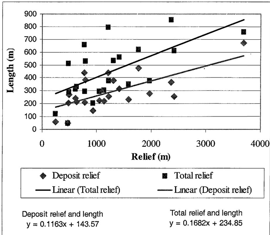
Figure 7. Scatterplot diagram of relief (deposit and total) versus length. The coefficient of determination ( $r^2$ ) for the deposit relief and length was 0.45. The coefficient of determination ( $r^2$ ) for the total relief and length was 0.40.
