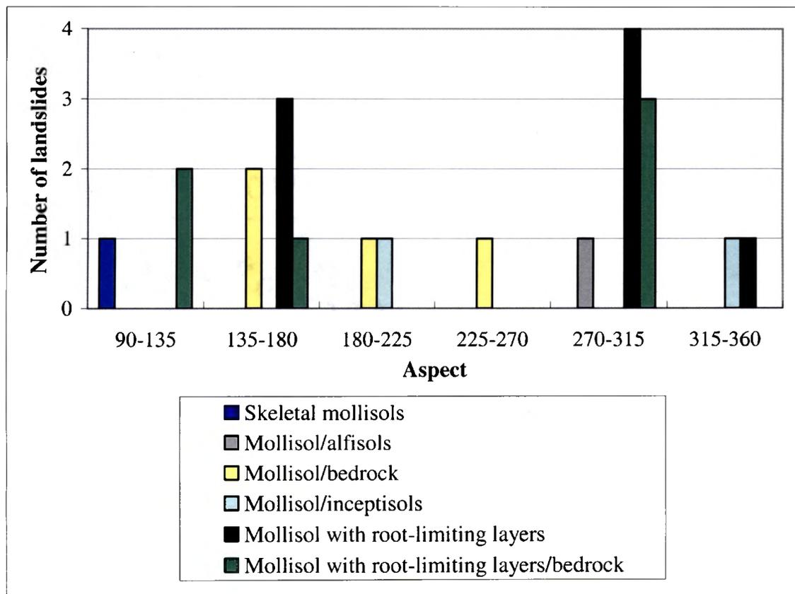
Figure 14. Histogram of the soil types, divided by aspect. Landslides did not occur from 0° - 90°.
