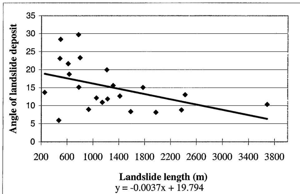
Figure 11. Scatterplot diagram of landslide length versus the angle of landslide deposit. The correlation of determination ( $r^2$ ) was 0.40.
