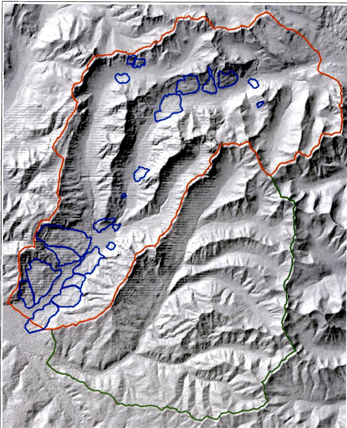
Figure 3. Landslide map of study area overlain on a 30-meter DEM.
