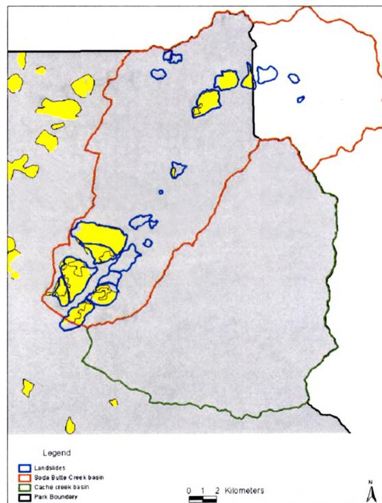
Figure 6. Comparison of landslide maps. Landslides mapped in this study (in blue) and landslides identified on the soil map (in yellow). The soil map was only for YNP and ended at the Park boundary (in black).
