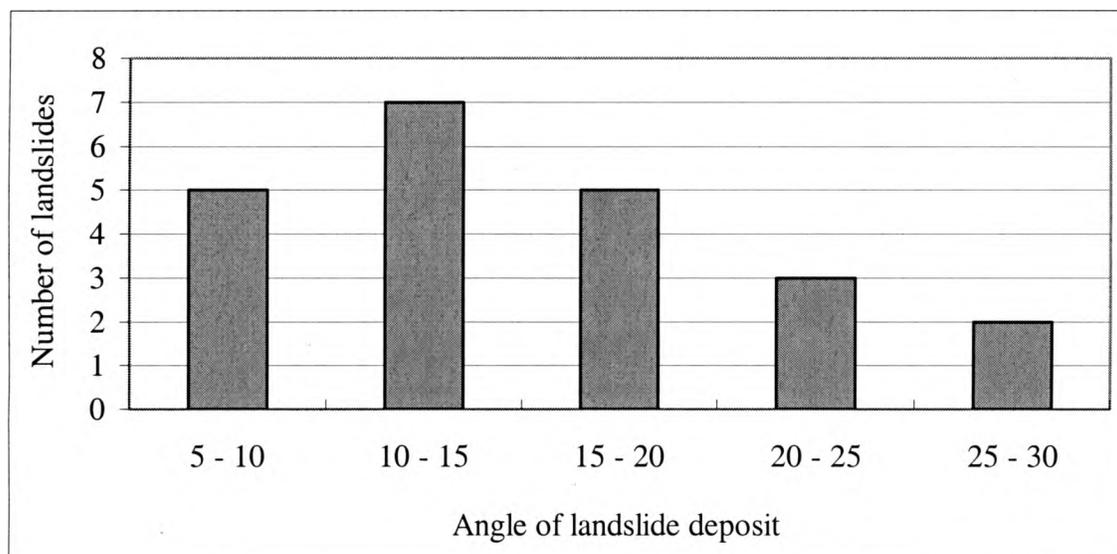
Figure 9. Histogram of the angle of landslide deposits.
