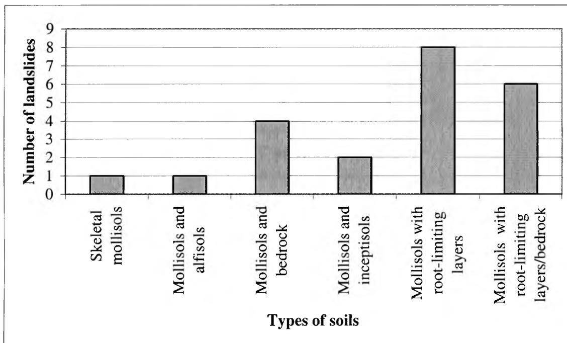
Figure 13. Histogram of the soil types found on the landslides.
