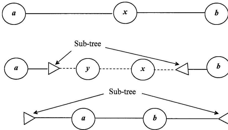
**Figure 5.3: Two non adjacent nodes can not reach TERMINAL state in STGCFA.**
