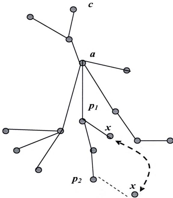
*In the adjacent sub tree,  $x$  leaving  $p_1$  and joining  $p_2$  or vice versa, can potentially displace the center.  $p_1$  or  $p_2$  should update node  $x$ 's displacement to its parent only if the last known largest HOP\_COUNT in its routing table is changed due to node  $x$ 's movement.*
