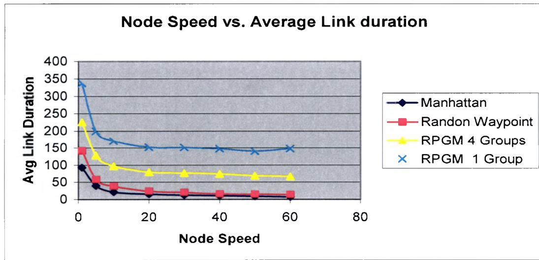
Figure 5.11: Average Link Duration vs. Node Speed, while transmission range = 100m.
