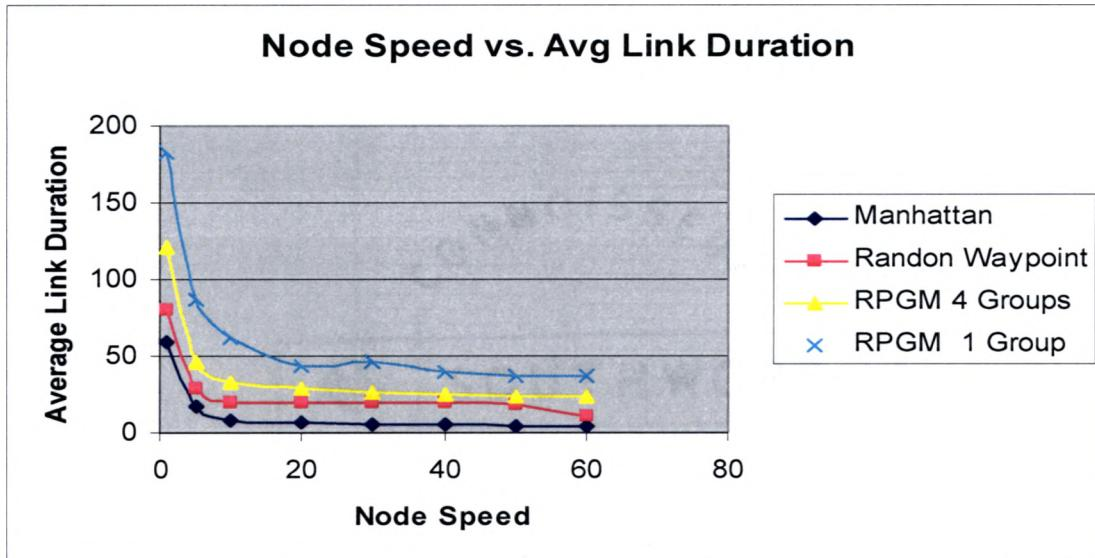
Figure 5.10: Average Link Duration vs. Node Speed, while transmission range = 50m.
