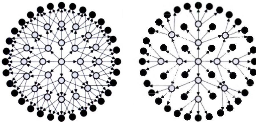
*Image on the left is flooding, where every node forwards messages, while in MPR only multi point relays (Grey nodes) can forward the messages*
