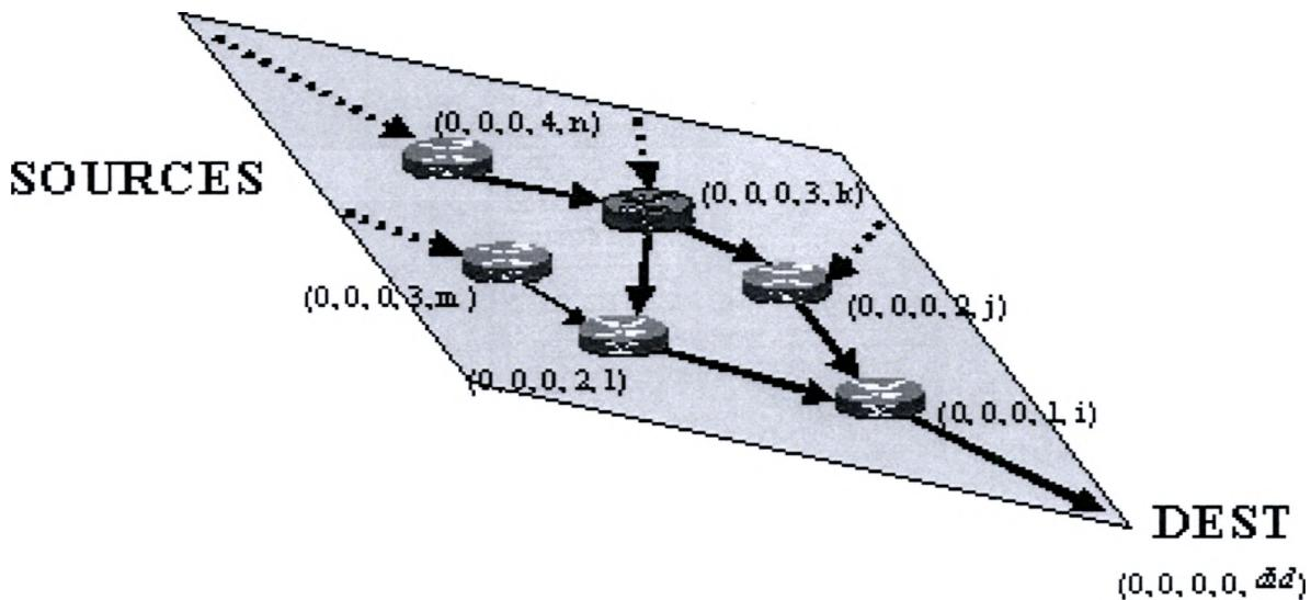
**Figure 2.1: Temporarily Ordered Routing.**
