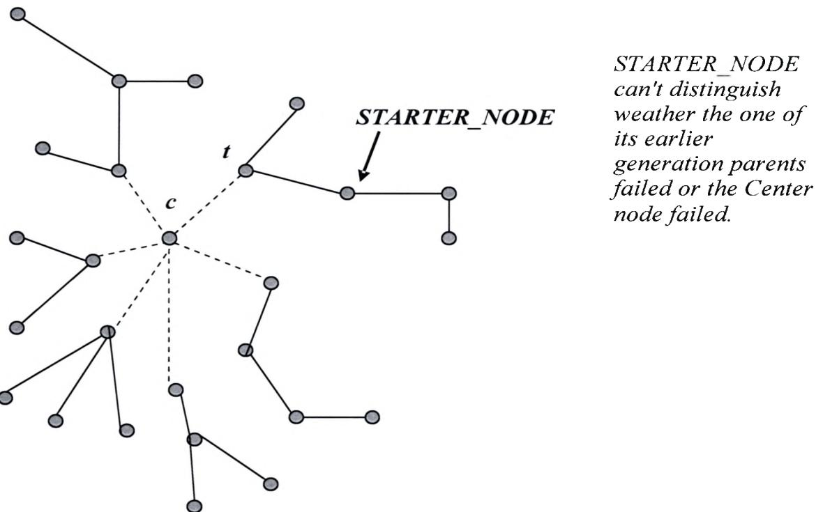
**Figure 4.9: Support for node failure.**
