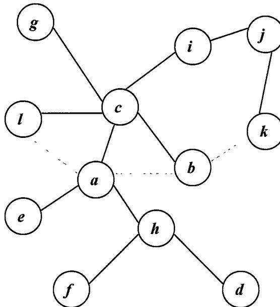
Figure 4.3: Spanning tree Generated by STGCFA.
