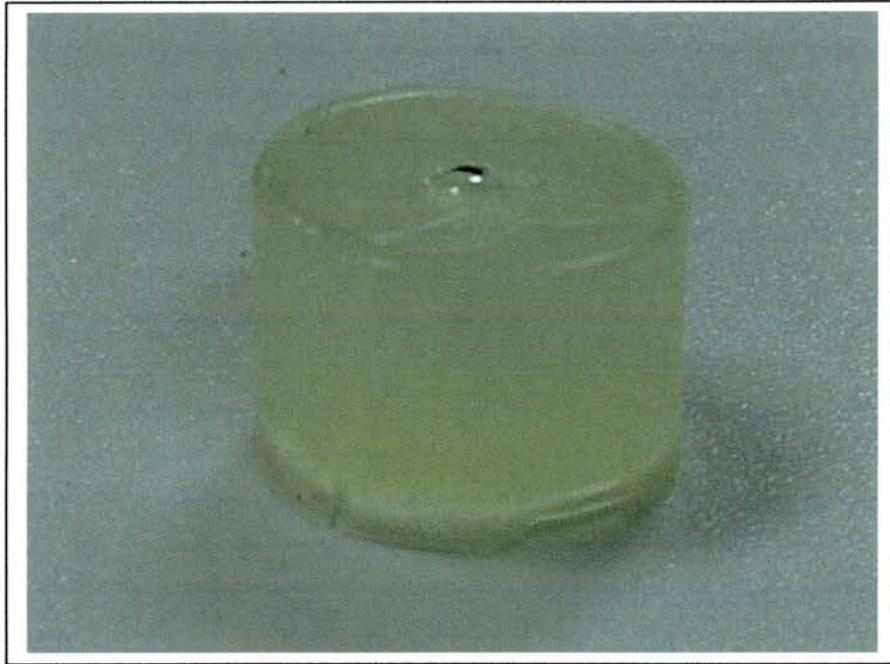
**Figure 3.7 Epoxy Mount (~1 inch dia.) with Sapphire Sphere**
