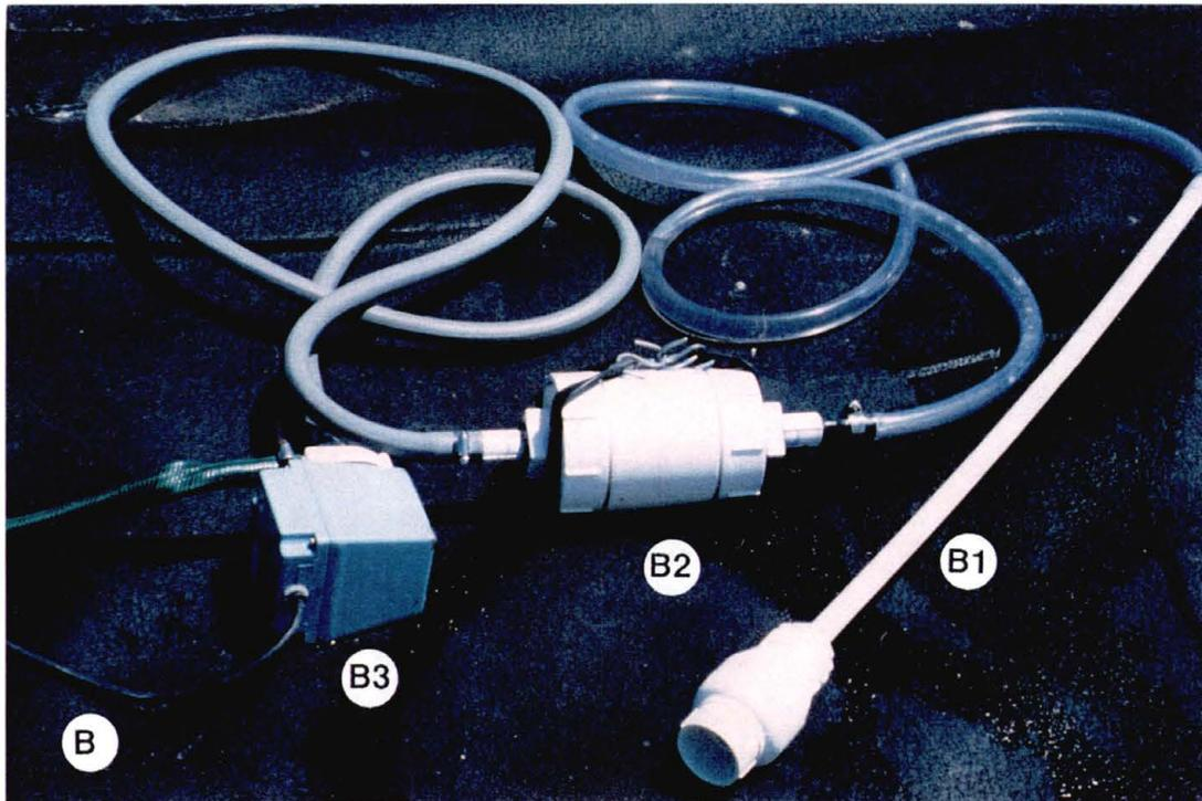
Figure 1. A modified Wellnitz (1991) continuous suction device, for sampling predaceous aquatic macroinvertebrates. A) frame and B) vacuum sampler. The vacuum sampler consisted of B1) sampling wand, B2) canister containing the filter, and B3) water pump.
