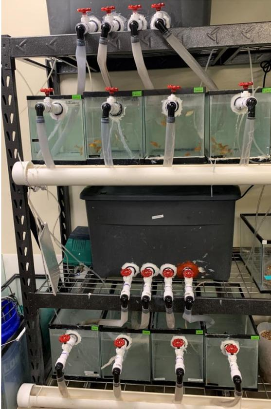
**Figure 2.** Continuous flow water setup. Depicted is the setup for two of the nitrite treatments. Water was added into the tote every 2 days and flowed down into the aquariums using gravity at a rate of 10-15 mL/ second. The water then flowed out of the aquariums and into a drainage system. This setup was designed to prevent the accumulation of nitrate and ammonia and keep the nitrite concentration at the desired level.
