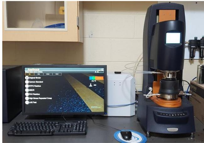
Figure 5. Dynamic Shear Rheometer
