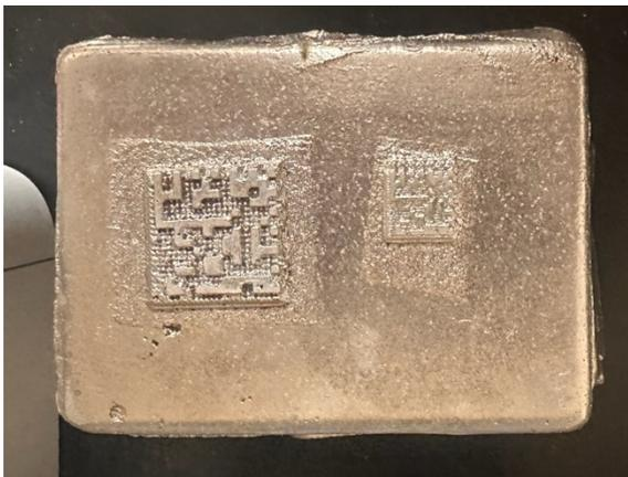
**Figure 3.13** Ground block with a negative pattern and dots on the base portion of the matrix code.
