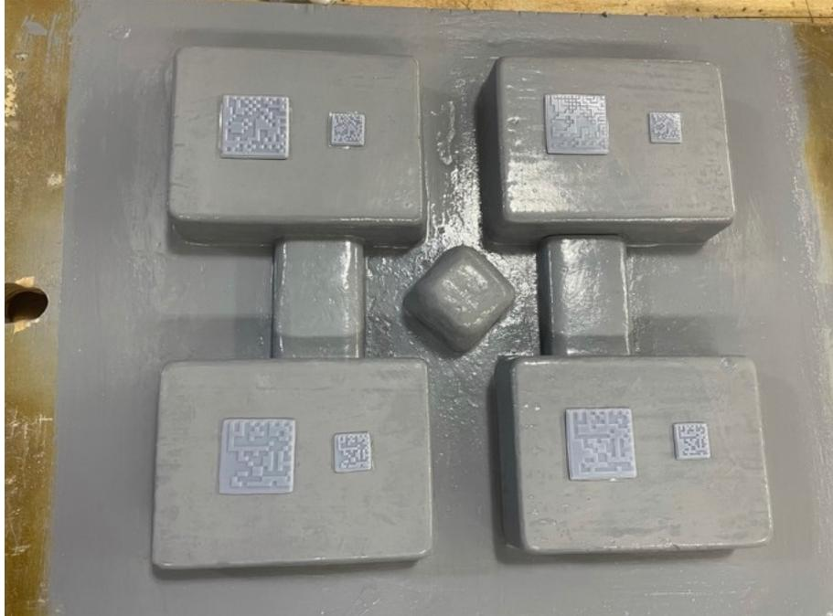
**Figure 2.3** The pattern that was used to create the mold in Figure 2.2. The printed tags are attached using double sided tape.
