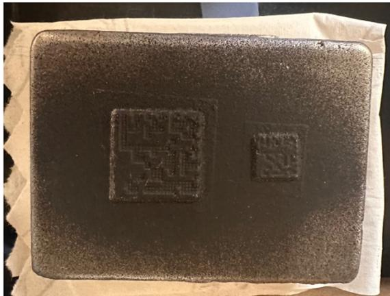
**Figure 3.16** Painted block with a positive pattern and dots on the filler portion of the matrix code.
