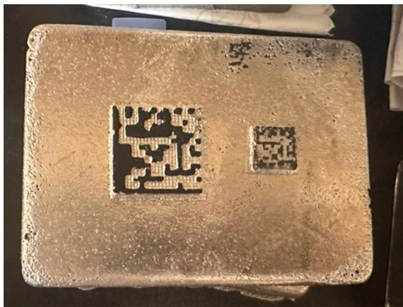
**Figure 3.8** Inked block with a positive pattern and dots on the filler portion of the matrix
