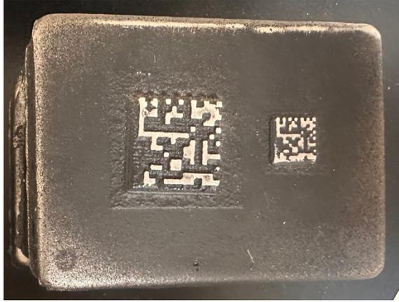
**Figure 3.21** Ground and painted block with a negative pattern and dots on the base portion of the matrix code.
