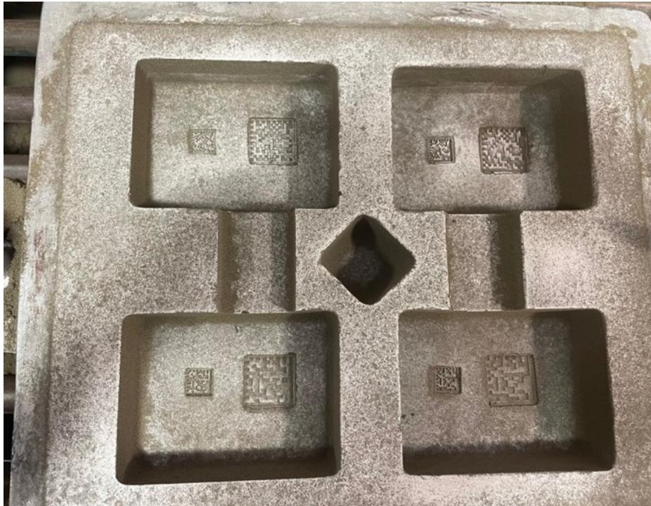
**Figure 2.2** An example of the how the mold looks after removing the pattern. Each block contains both a 1 inch x 1 inch tag and a 0.5 inch x 0.5 inch tag.
