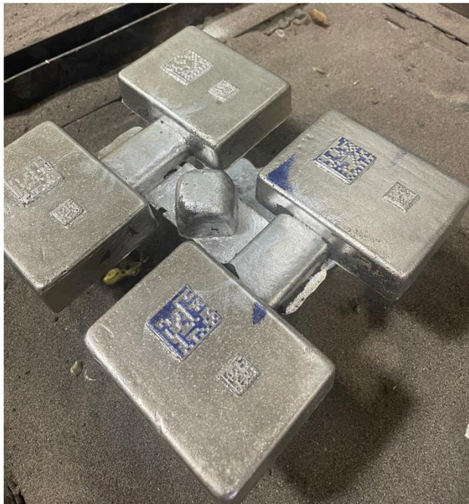
**Figure 3.1** Blocks removed from mold. These blocks are still attached to each other as well as the runner and gating system. Right hand blocks were inked using a standard ink pad to test effect.
