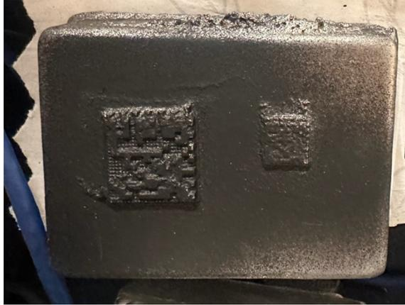
**Figure 3.17** Painted block with a negative pattern and dots on the base portion of the matrix code.
