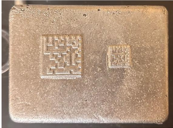
**Figure 3.3** As-Cast block with a negative pattern.
