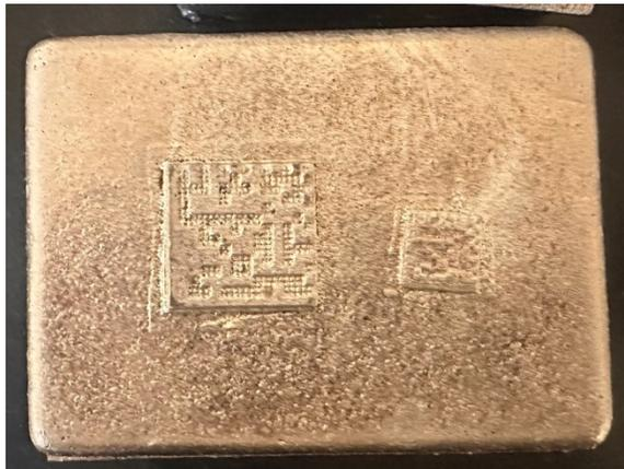
**Figure 3.4** As-Cast block with a positive pattern and dots on the filler portion of the matrix code.
