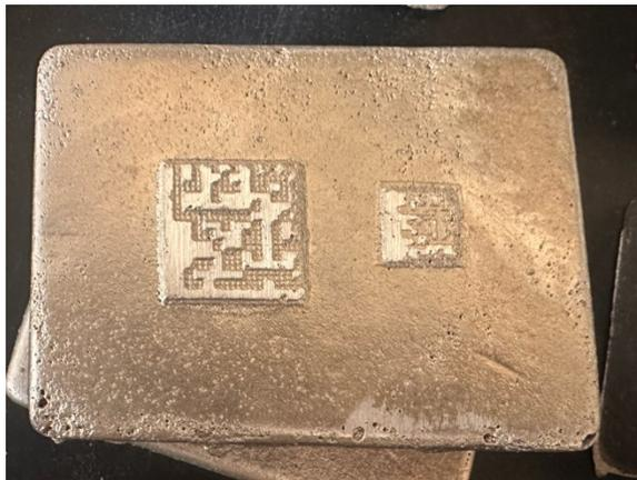
**Figure 3.12** Ground block with a positive pattern and dots on the filler portion of the matrix code.
