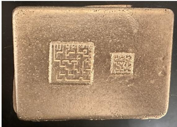
**Figure 3.2** As-Cast block with a positive pattern.
