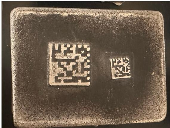
**Figure 3.18** Ground and painted block with a positive pattern.
