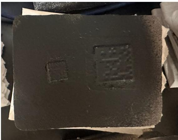
**Figure 3.14** Painted block with a positive pattern.
