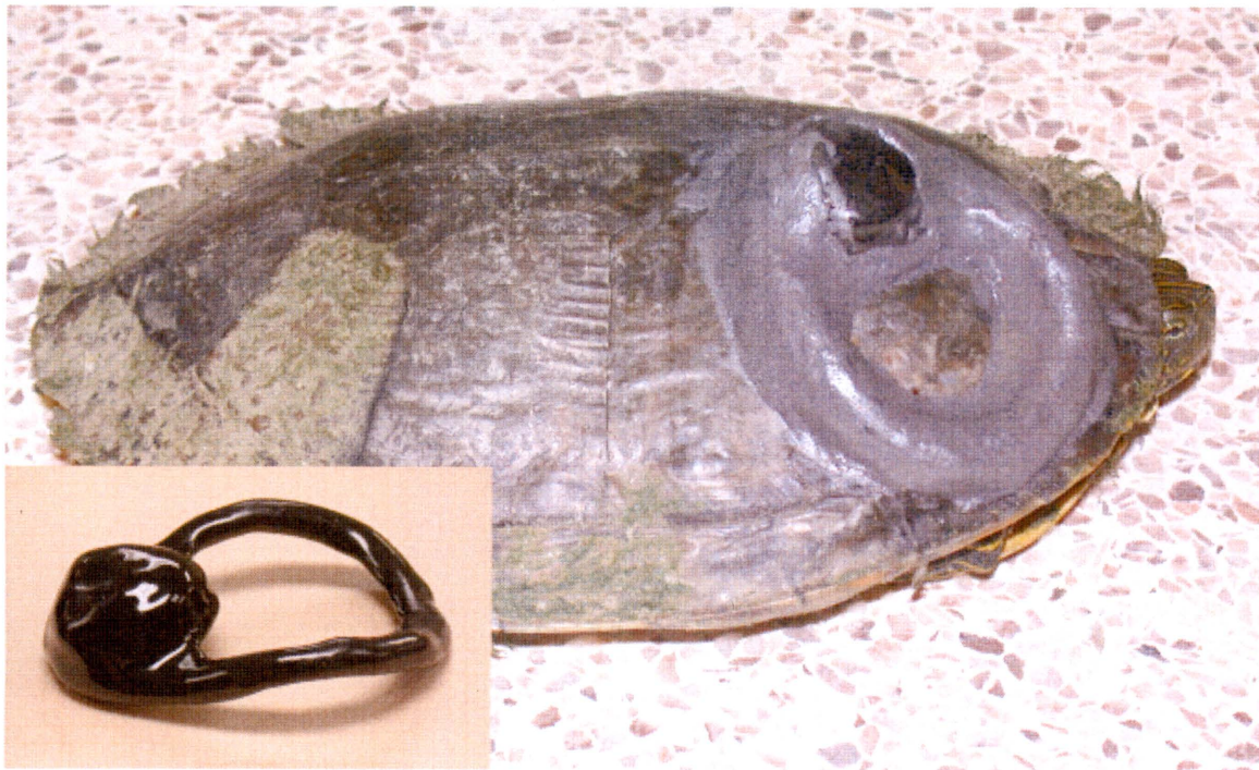
Figure 3. The revised transmitter with a loop antenna.
