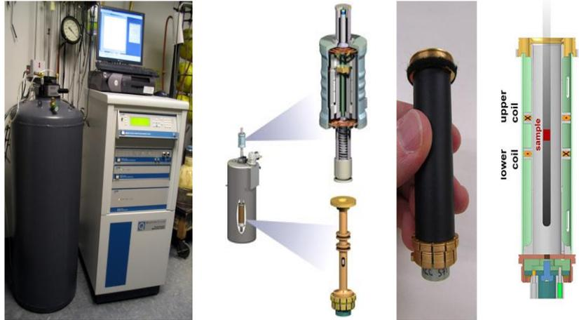
Figure 3. 3. Left to Right: PPMS apparatus (a), VSM attachments for PPMS (b), photograph of the VSM puck (c), a cross-section of VSM puck (d), at Texas State University.
