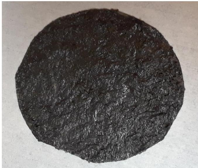
Figure 3. 22. Defocusing correction sample prepared by using superglue: showing nonuniform thickness.
