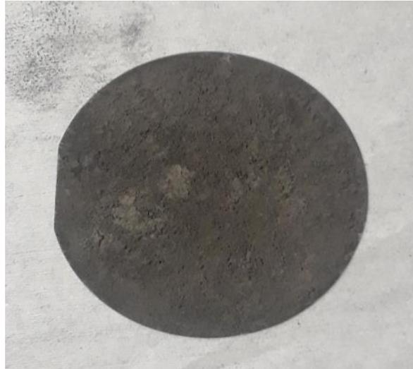
Figure 3. 23. Defocusing correction sample prepared by using hair spray.
