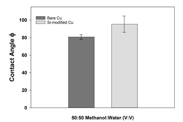
Figure 7. Contact angle measurements using 20 µL of 50:50 methanol:water (V:V) on a bare copper surface and a Si-modified surface, (n=10).
