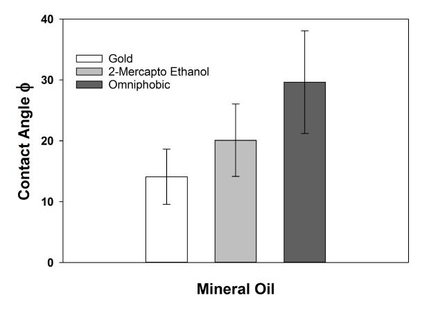
Figure 19. Contact angle measurements were performed on a copper-gold plated surface, 2-mecapto ethanol surface, and the omniphobic surface with an n=11 and their respective 95% confidence intervals using 18 µL of mineral oil.
