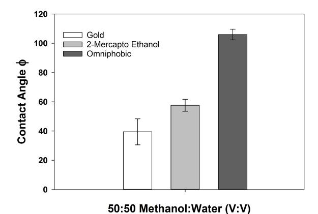
Figure 18. Contact angle measurements were performed on a copper-gold plated surface, 2-mercapto ethanol-gold surface, and the omniphobic surface with an n=11 and their respective 95% confidence intervals using 18  $\mu$ L of 50:50 methanol:water (V:V).
