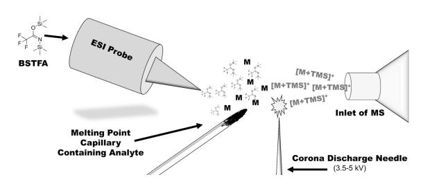
Figure 28. ASAP schematic using direct infusion of BSTFA for online derivatization.
