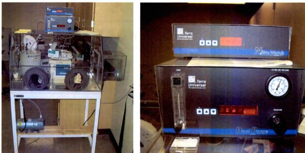
**Figure 17 (left) Glove box with all tools inside and controllers on top. (right) Humidity controller *Nitro watch* and gas supply control *Dual Purge*.**
