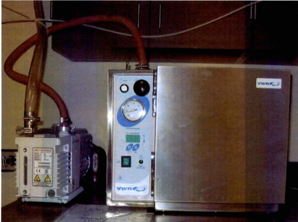
**Figure 48 Vacuum or annealing oven. To the left is the vacuum pump, the oven control panel contains power switch, temperature setting, vacuum gauge, and vent/vacuum valves.**
