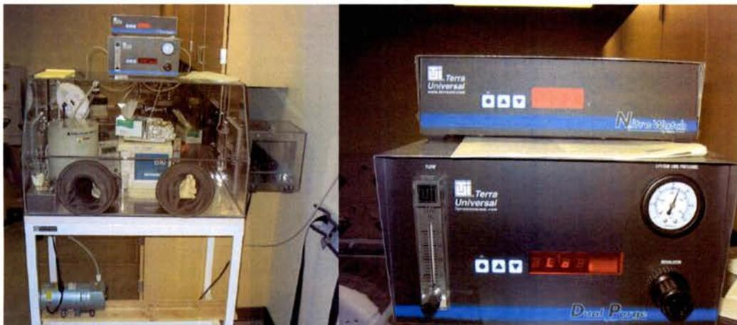
**Figure 46 (left) Glove box with all tools inside and controllers on top. (right) Humidity controller *Nitro watch* and gas supply control *Dual Purge*.**
