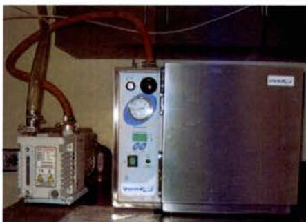
**Figure 20** Vacuum or annealing oven. To the left is the vacuum pump, the oven control panel contains power switch, temperature setting, vacuum gauge, and vent/vacuum valves. RCP was annealed at 140 °C and DBCs were annealed at either 160 °C or 180 °C.
