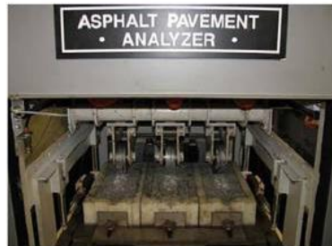
(b) Asphalt Pavement Analyzer used in the Loaded wheel test
