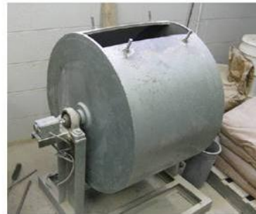
(a) Los Angeles Abrasion Machine used in the Cantabro Loss test
