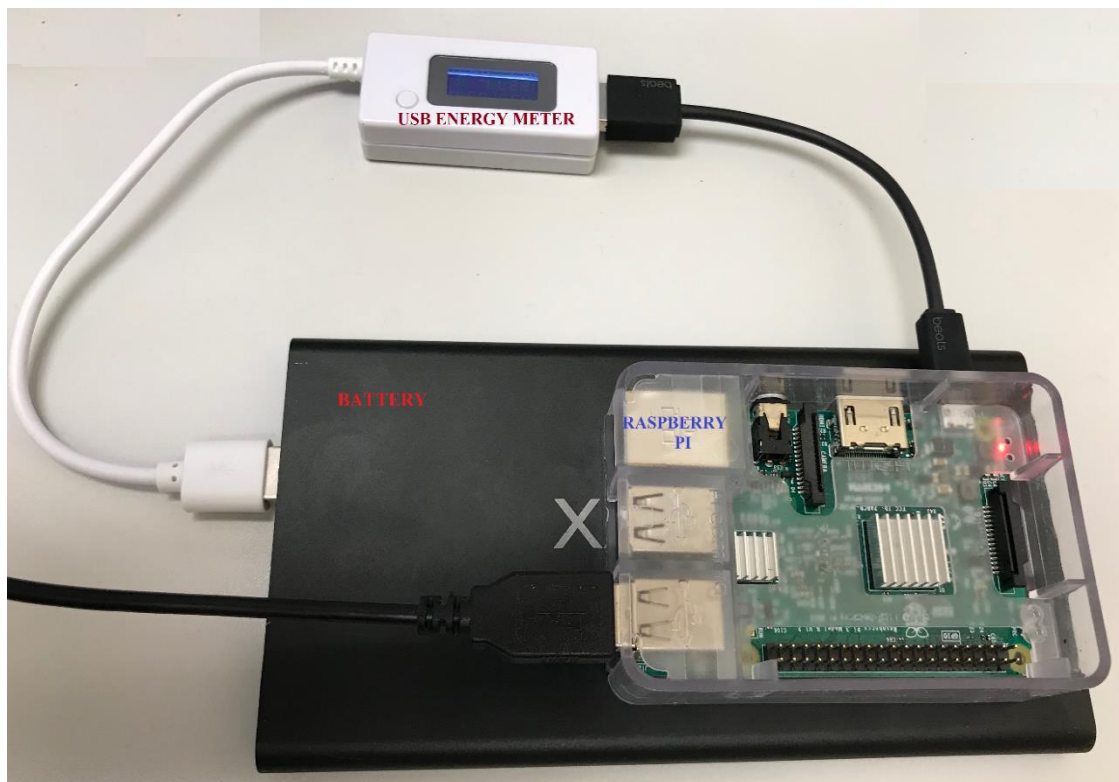
Figure 10: Power usage measurement setup
