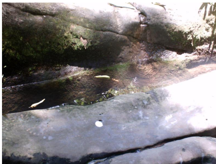
Figure 26. One of several sites testing for E. coli around San José en Rebeldía. All sites tested negative as indicated by the white test pad, the small white disc in the lower left center of the photo.
