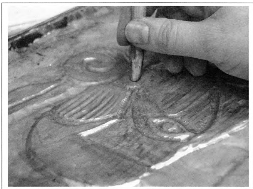
Illustration 8.70 Working Plate in Pitch
