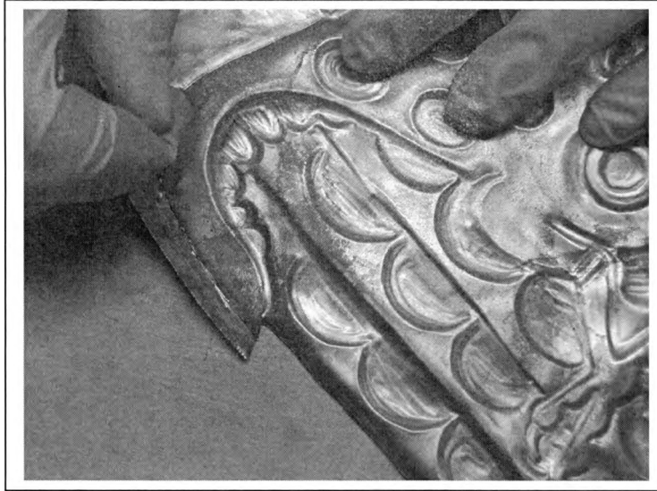
Illustration 8.39 Cutting the Free Hand Plate
