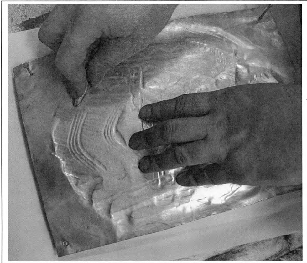
Illustration 8.49 Burnishing the Plate
