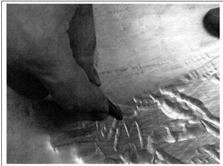
Illustration 8.91 Burnishing the Plate
