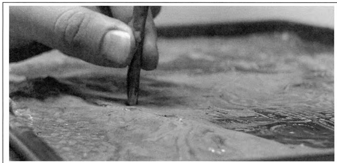
Illustration 8.81 Cutting While Embedded in Pitch
