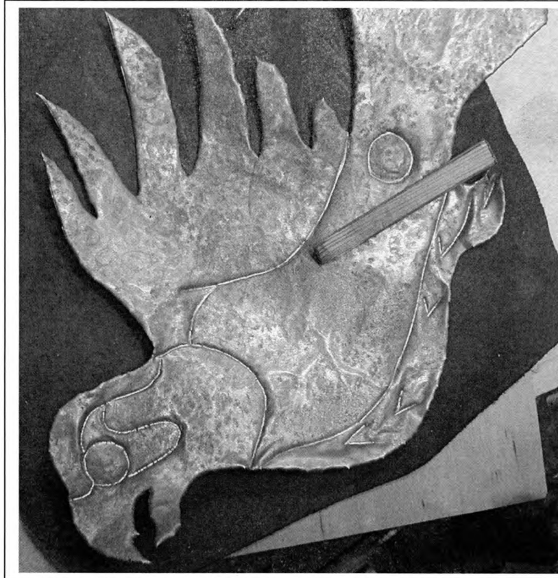
Illustration 7.14 Partially Chased Freehand Plate
