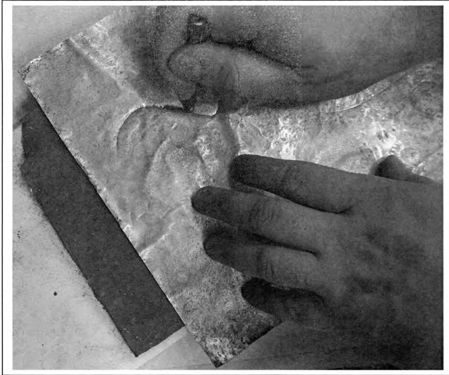
Illustration 7.11 Cutting with Copper Chisel
