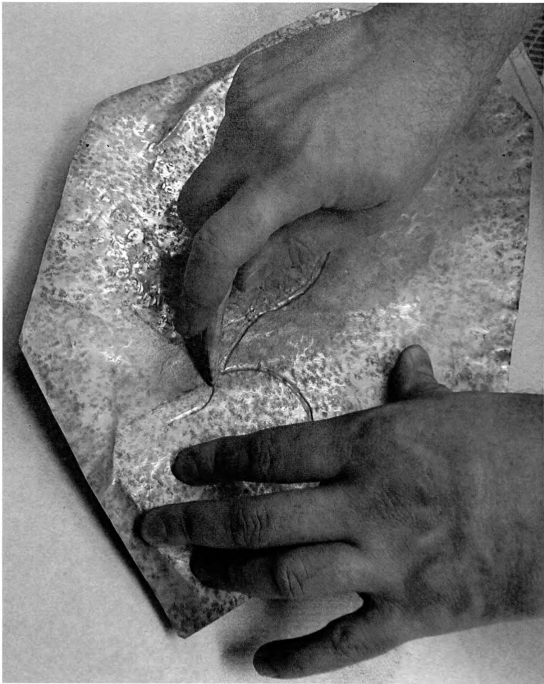
Illustration 7.20 Using the Antler Tine to Define the Raptor Shape
