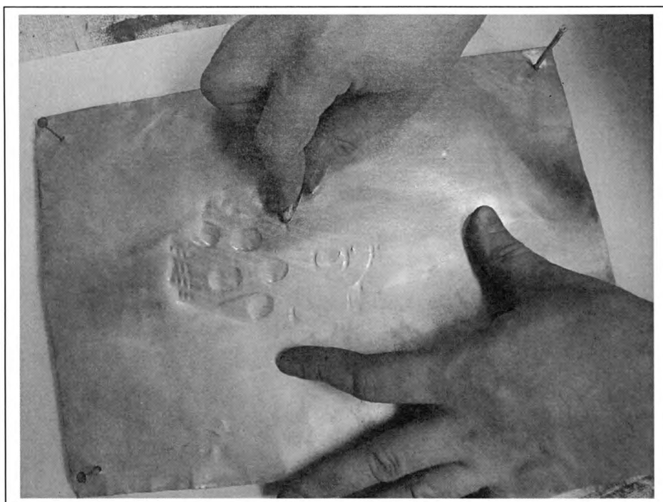
Illustration 8.45 Burnishing the Plate
