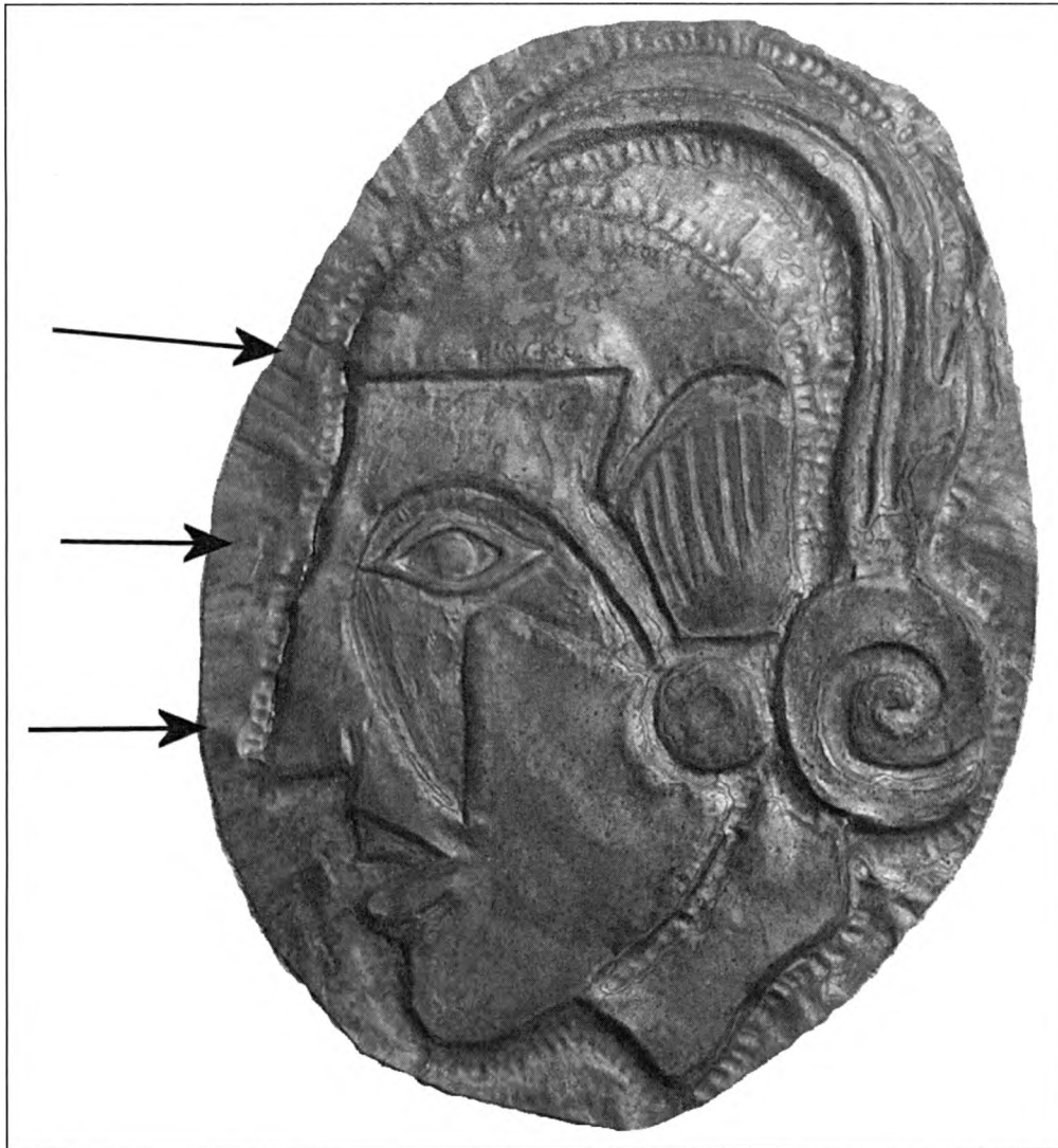
Illustration 8.66 Completed Plate Utilizing Template Only Showing Area of Cutting
