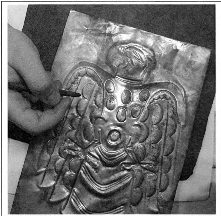
Illustration 8.38 Chasing Repeated on Backside of Plate
