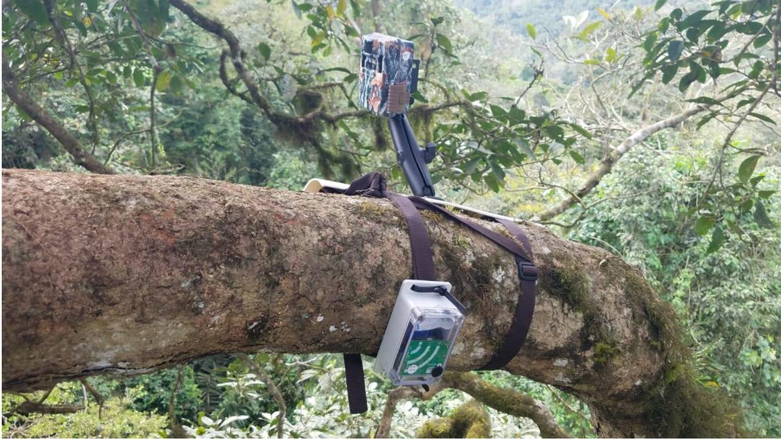
**Figure 2:** Canopy station – the AudioMoth is positioned slightly under the tree to decrease chance of water buildup and in a weatherproof case that has a membrane to allow sound to pass and a silica packet in the event moisture enters. The camera is mounted on an arm and positioned so it will not interfere with wildlife movement and is facing the main branch. Not photographed is the kestrel.
