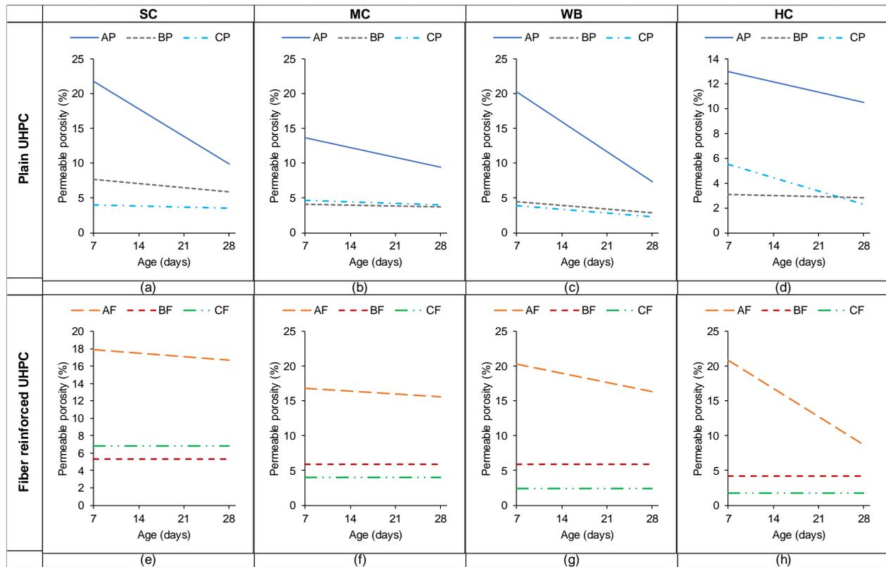
**Figure 4.** Permeable porosity of plain UHPC mixtures cured under (a) SC, (b) MC, (c) WB, and (d) HC regimes and permeable porosity of fiber reinforced mixtures cured under (e) SC, (f) MC, (g) WB, and (h) HC regimes.
