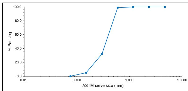
**Figure 1.** Particle size distribution of fine aggregate.
