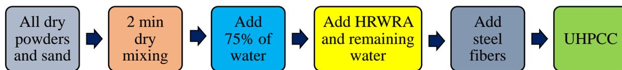
**Figure 2.** Mixing procedure for UHPC.
