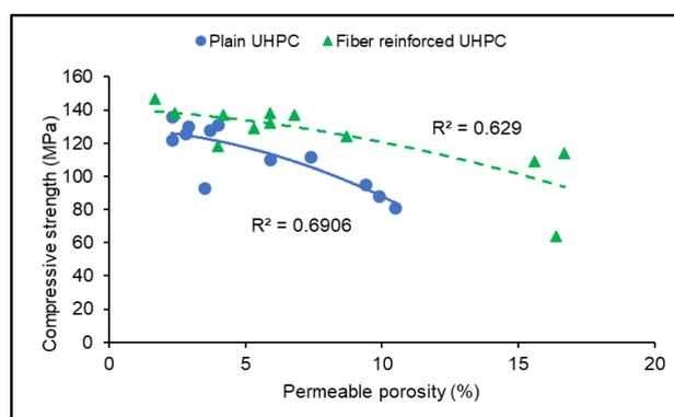
**Figure 13.** Compressive strength vs. permeable porosity for formulated UHPC mixtures after 28 days of curing.
