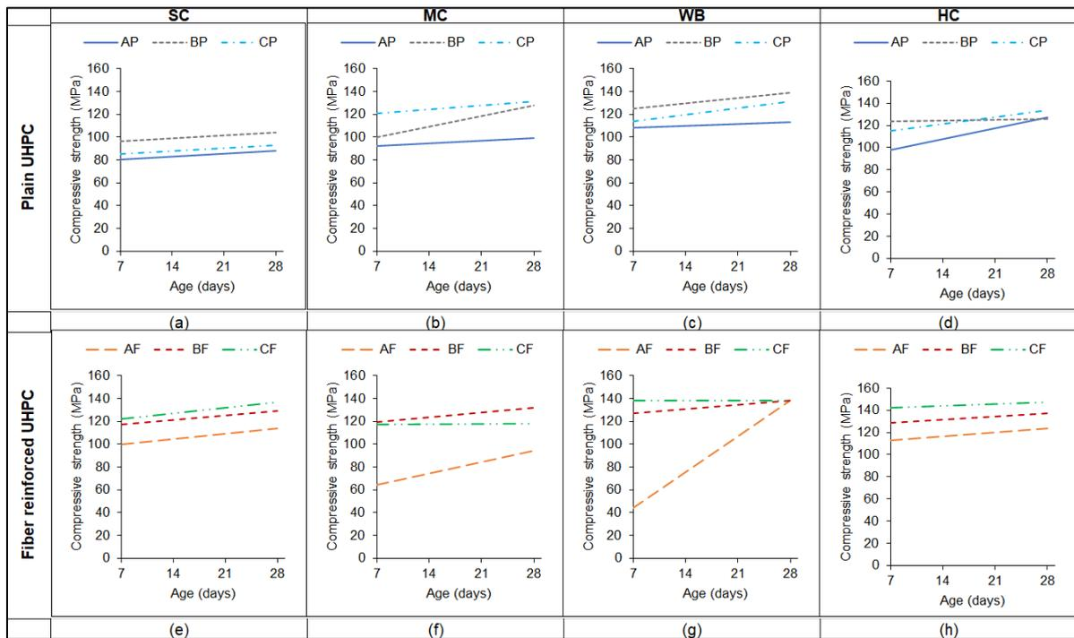
**Figure 8.** Compressive strengths of 50 mm cube specimens of plain UHPC mixtures when cured under (a) SC, (b) MC, (c) WB, and (d) HC regimens and compressive strengths of 50 mm cube specimens of fiber reinforced UHPC mixtures when cured under (e) SC, (f) MC, (g) WB, and (h) HC regimens.
