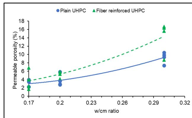
**Figure 6.** Permeable porosity vs. w/cm ratio for formulated UHPCs.
