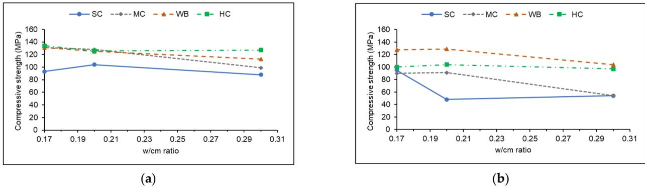
**Figure 10.** Effect of different curing regimens on compressive strength of plain UHPC mixtures (a) 50 mm cube specimen and (b) 100 mm cube specimens.
