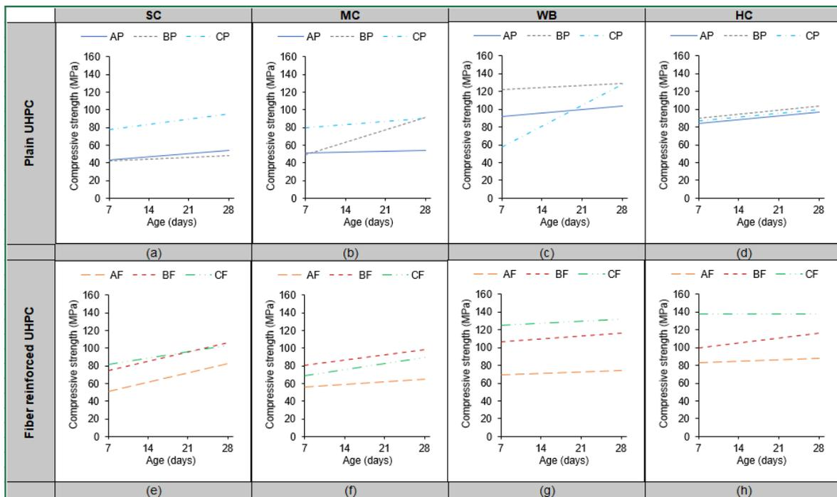
**Figure 9.** Compressive strengths of 100 mm cube specimens of plain UHPC mixtures when cured under (a) SC, (b) MC, (c) WB, and (d) HC regimens and compressive strengths of 100 mm cube specimens of fiber reinforced UHPC mixtures when cured under (e) SC, (f) MC, (g) WB, and (h) HC regimens.
