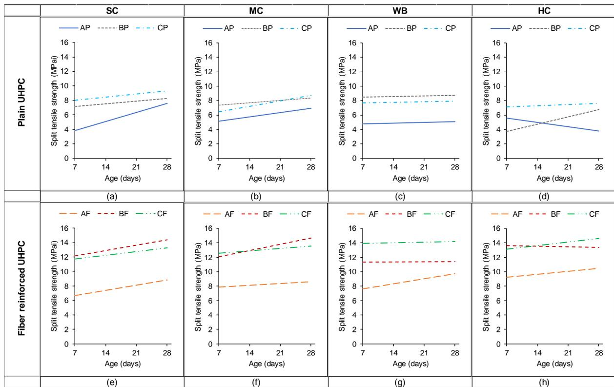
**Figure 14.** Split tensile strength of plain UHPC mixtures when cured under (a) SC, (b) MC, (c) WB, and (d) HC regimens and split tensile strength of fiber reinforced UHPC mixtures when cured under (e) SC, (f) MC, (g) WB, and (h) HC regimens.
