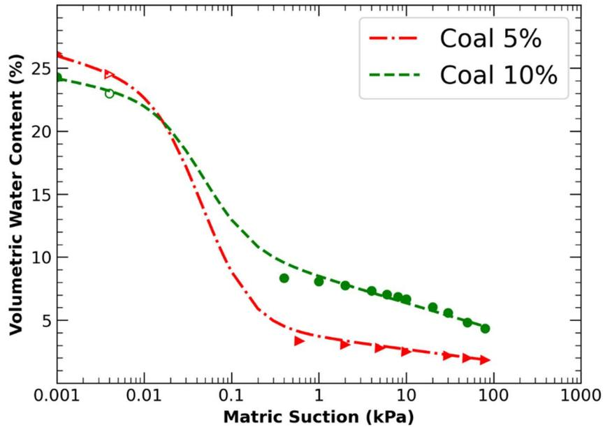
Figure 4-3 SWRC of Coal Fouling
