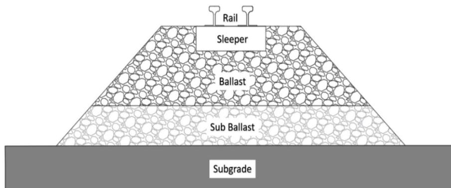
Figure 1-1 Cross Section of Railway
