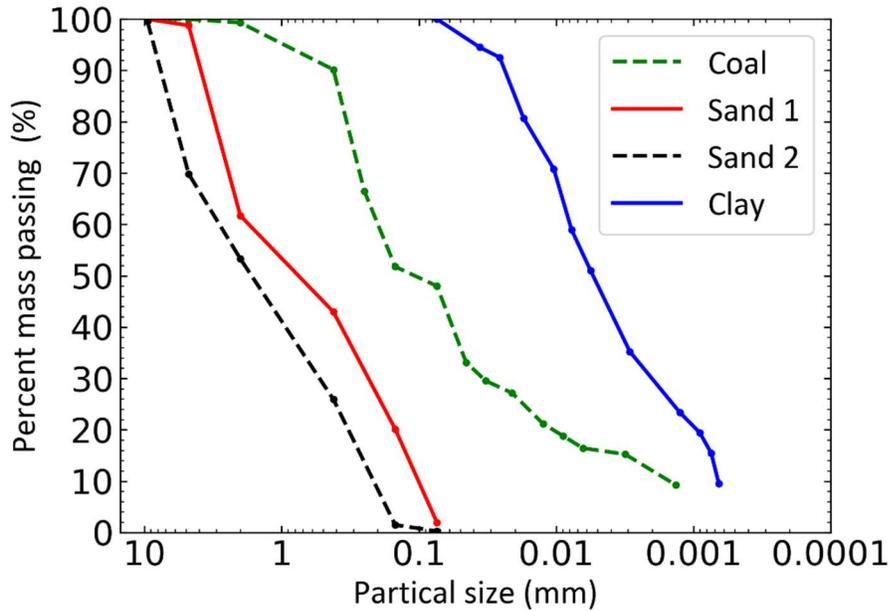
Figure 3-1 Grain Size Distribution of Fouling Material
