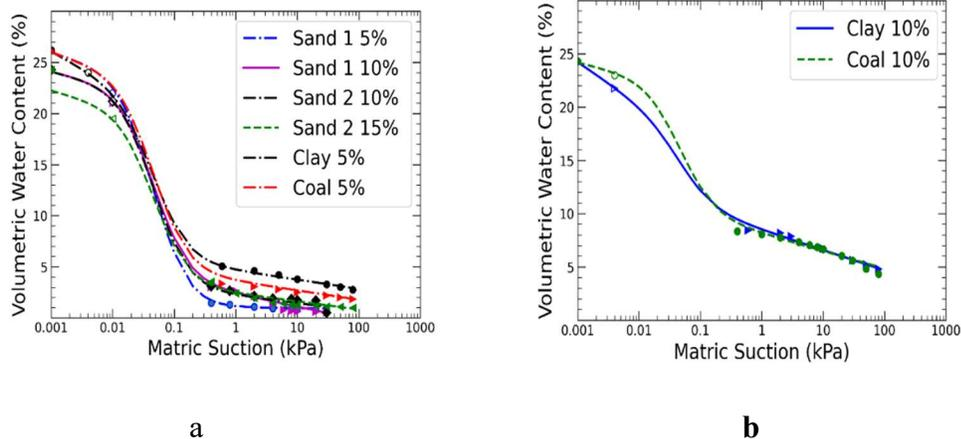
Figure 4-6: SWCR for (a) Moderately Clean FI and (b) Moderately fouled FI
