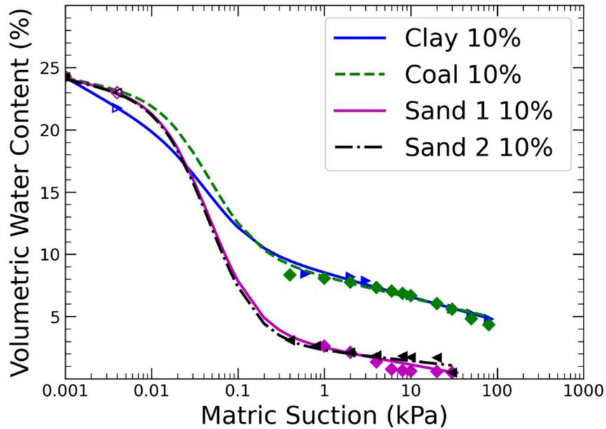
Figure 4-5 Comparison of the 10% Fouled Ballast
