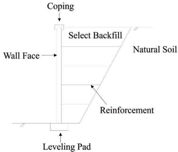
Figure 1-3 Schematic of an MSE wall
