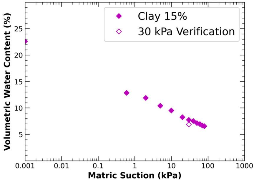
Figure 4-1 First Clay Test with a Verification Test
