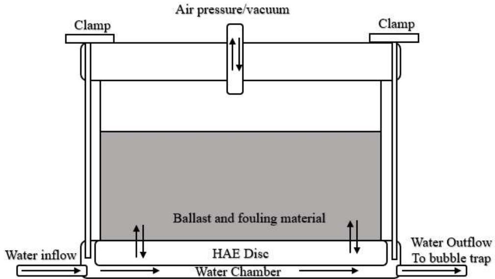
Figure 3-2 Theoretical Test Setup
