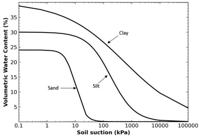
Figure 2-3 Typical SWRC for Different Soils
