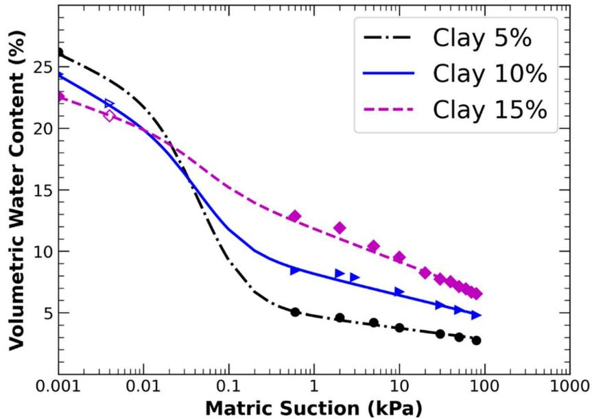
Figure 4-4 SWRC of Clay Fouling
