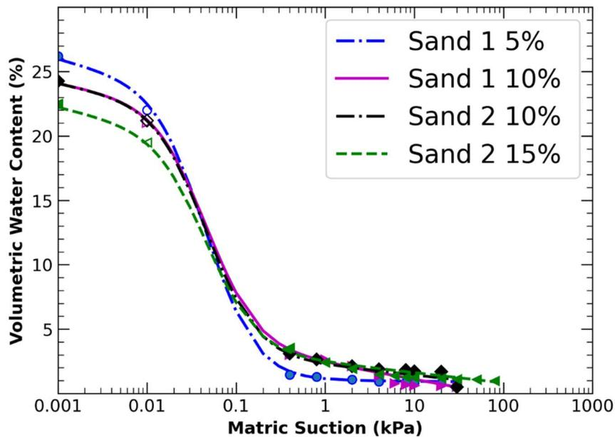
Figure 4-2 SWRC of Sand Fouling
