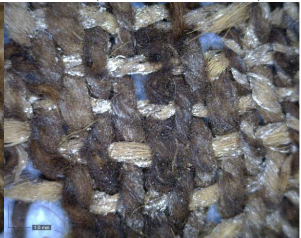
Detail of Repair with Solid Dark Brown Warps
