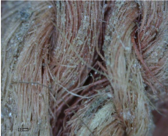
Fiber under 202x Magnification
