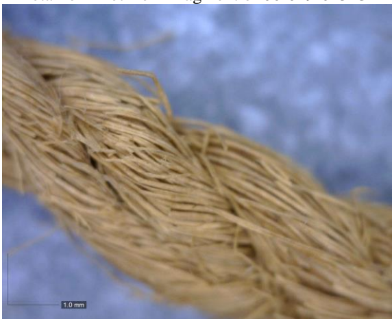
Z(3S) Cord Ply Configuration from 06-019-043-G
