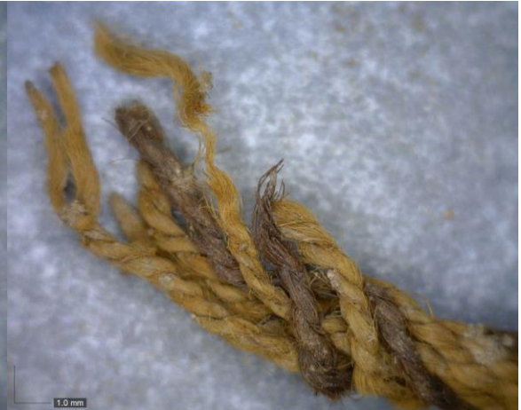
Specimen 06-032-006-F - Detail of Frayed End
