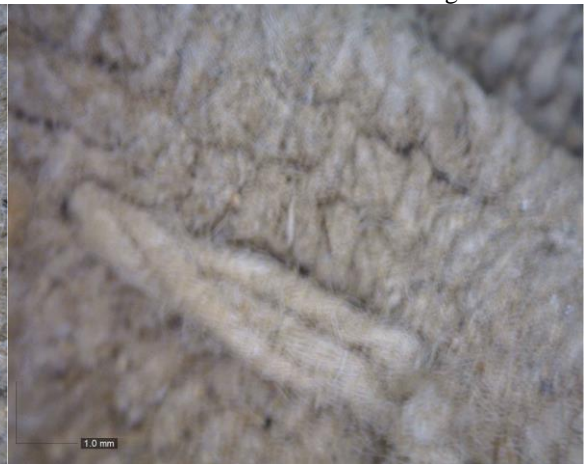
Textile Db End Selvedge and Sewing Stitch Detail
