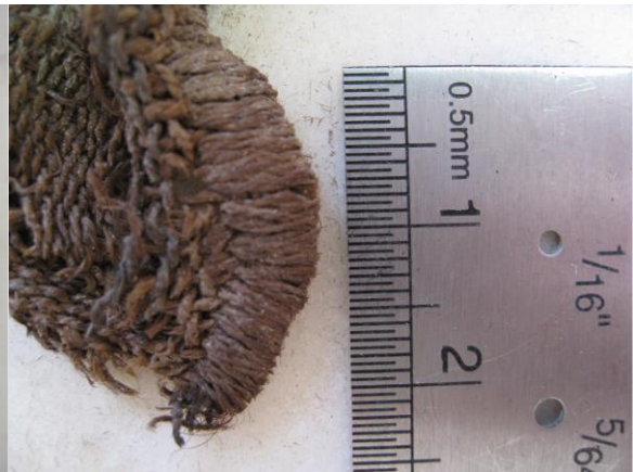
Detail of Border Covering Side Selvedge
