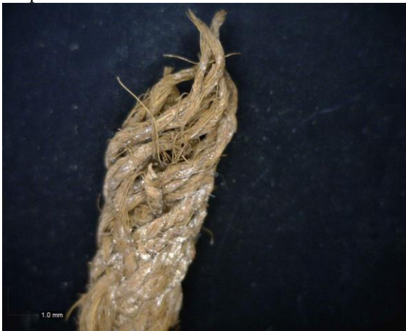
Detail Showing Structure Unraveling
