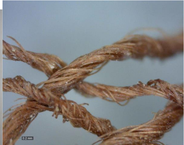
Dyed Red Wool Yarns Magnified 217x
