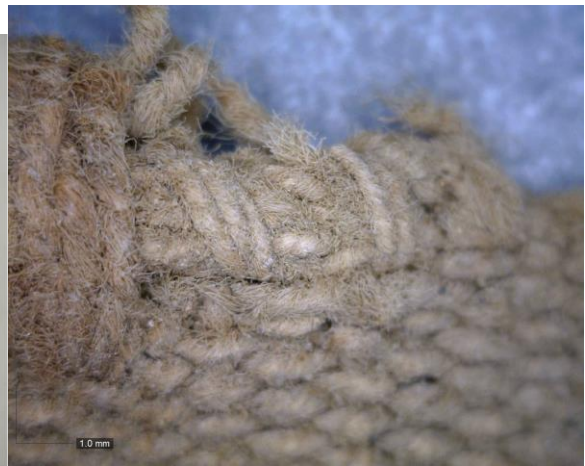
Detail of Rolled Hem/Side Selvedge
