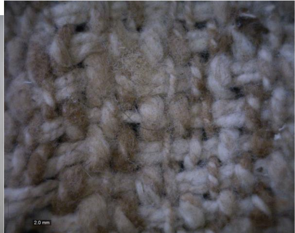
Weave Detail with Barber-Pole/Mottled Elements
