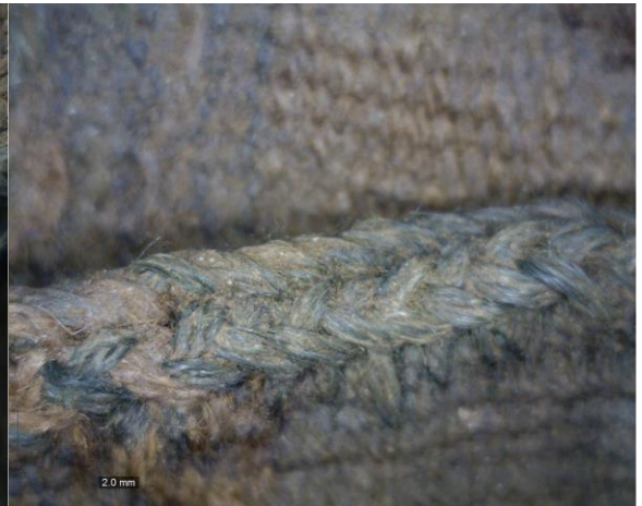
Cross Knit Stitch Side Seam Detail
