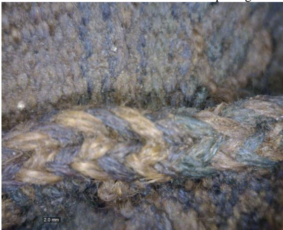
Cross Knit Stitch Side Seam Detail
