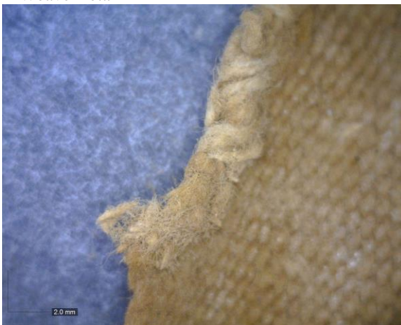
Detail of Outside Side Selvage and Whip Stitch
