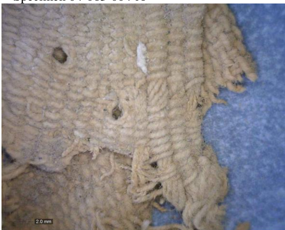
Voids from Stitches down Patch
