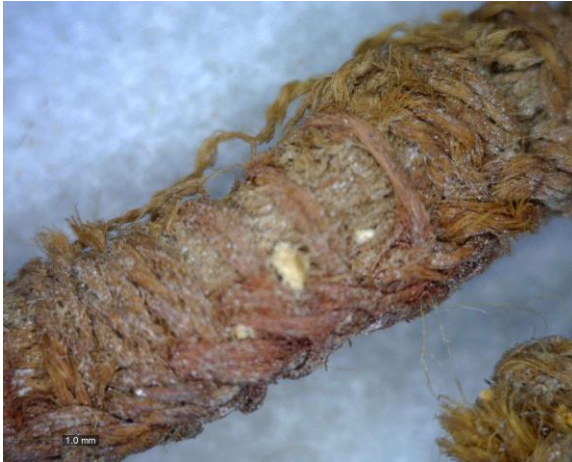
Dyed Red Fiber and Damage Exposing Core
