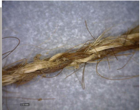
Detail of Ply Configuration
