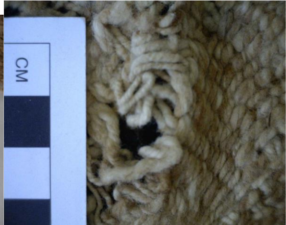
Detail Showing Hole/Void in Fabric
