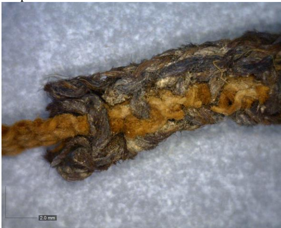
Binding Interwoven through Main Body
