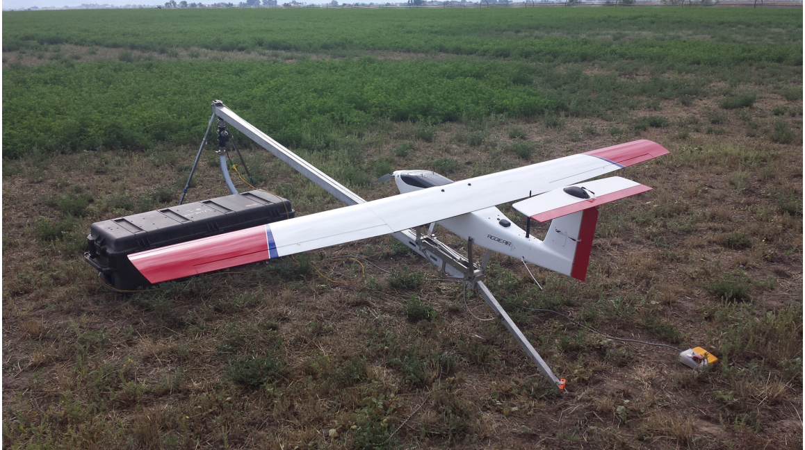
Figure 7. The Minion 2.0 fixed-wing UAS. Platform developed by AggieAir (Utah State University, Logan, UT, USA). Pictured is the launching system (pneumatic rail) as well as the platform itself. Surveys with the Minion were flown at 300 and 200 m.
