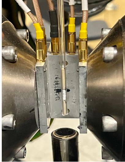
**Fig. 6.15:** The field-annealed  $\text{SrO}(\text{Fe}_2\text{O}_3)_6/\text{PA12}$  cylindrical-shaped filament wrapped with Teflon tape and secured in Pyrex glass tubes with PEEK stoppers and high temperature silicone glue for torque measurement.
