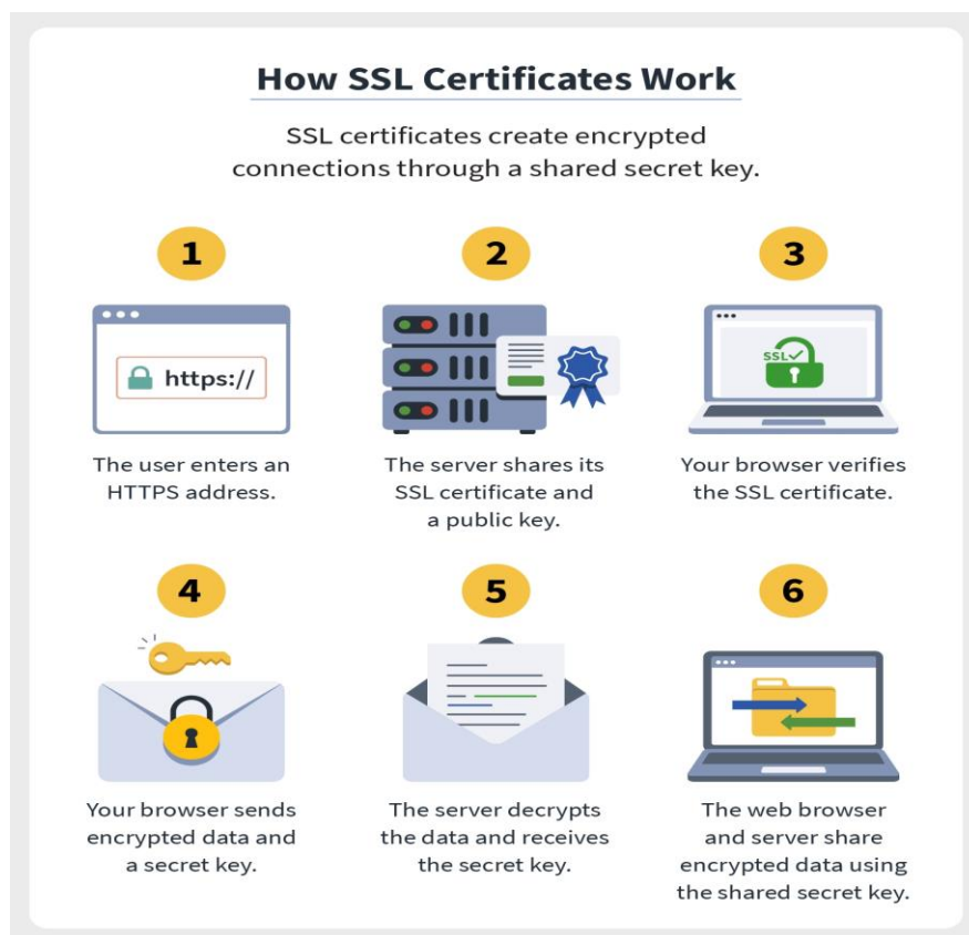
Figure 6 - How SSL Certificates Work
