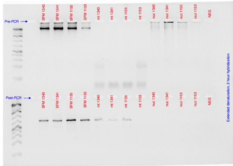
**Figure 8: Gel Electrophoresis of SFM line of products before (top row) and after PCR (bottom row) after an extended denaturation. Denaturation occurred for 30 minutes, while hybridization occurred for 2 hours at 50 °C.**
