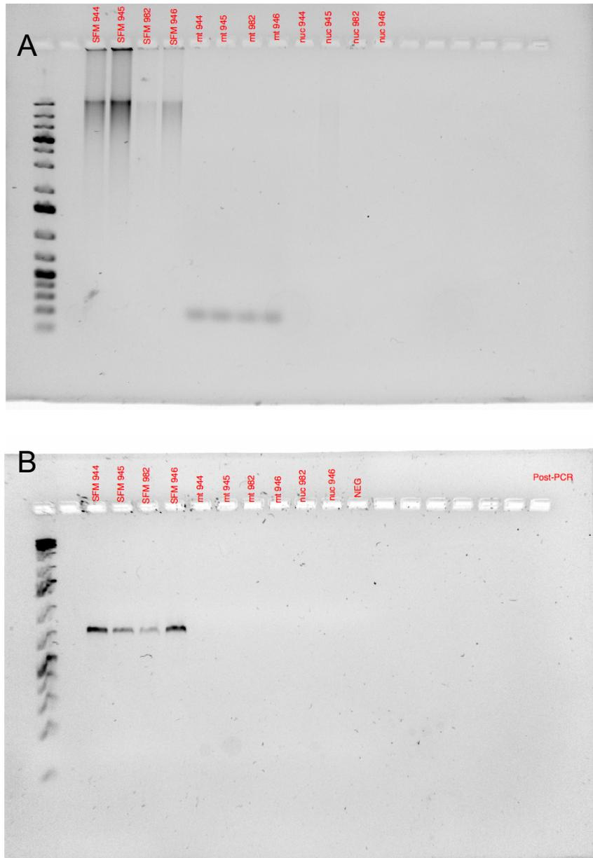
**Figure 3: Gel Electrophoresis of magnetic capture products before (A) and after PCR (B). Dynabeads M-270 Streptavidin were used and hybridization temperature was 45 °C**
