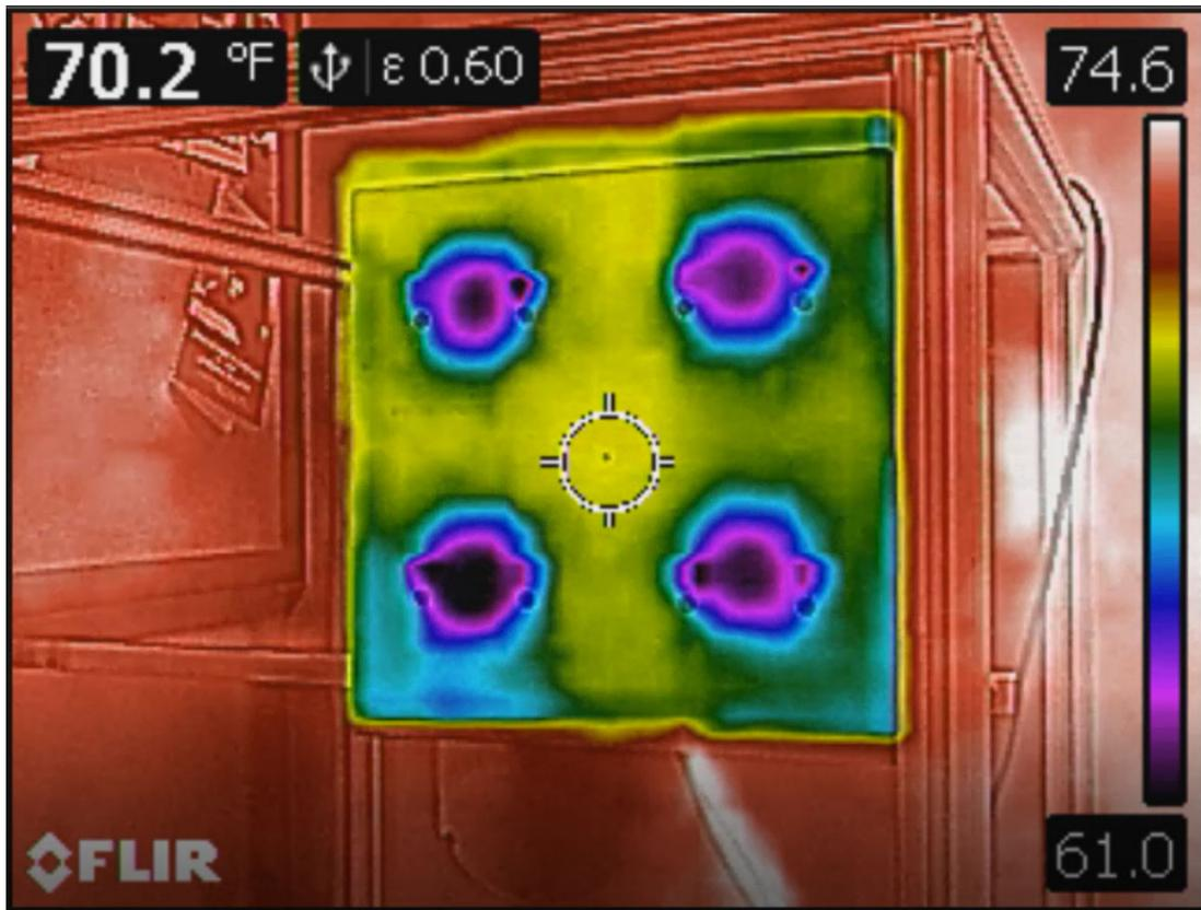
Figure 33 – Condensation Plate Temperature Distribution
