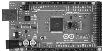
Figure 7 - Arduino Mega Microcontroller
