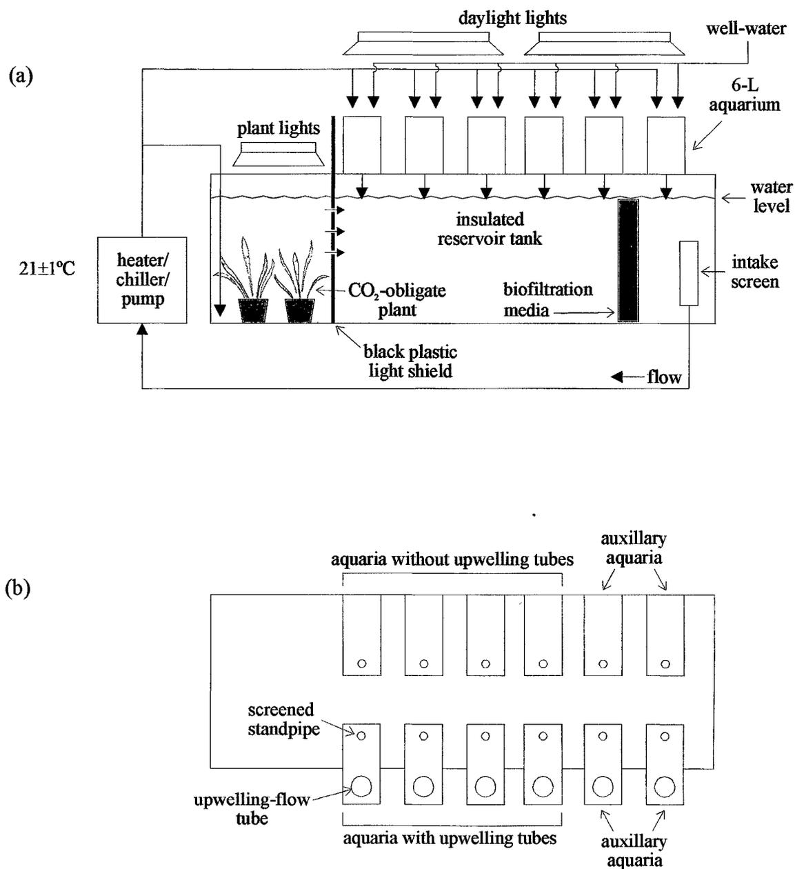
Figure 1. Schematic of one of three water recirculation systems with (a) a side view of the interactions of the different components of a system and (b) a top view of the arrangement of aquaria used in the 9-month experiment to examine the effects of diel water quality fluctuations and upwelling flow in the San Marcos salamander. Overflow pipe not shown. Auxiliary aquaria used for taking water quality measurements and holding replacement salamanders. Not to scale.
