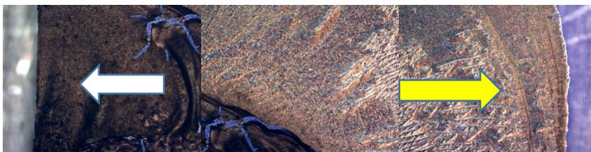
Figure 42: Optical microscope image of a P3HT film templated from 32% DMSO/chlorobenzene. The white arrow indicates where pore formation accumulates at lower DMSO percentages (left film edge), and the yellow arrow shows where pore formation accumulates at the higher DMSO percentages (right film edge)
