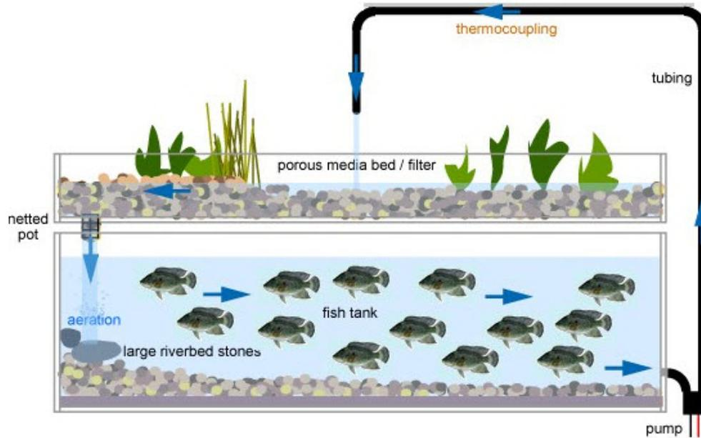
*Figure 3. An overview of an aquaponics system in which the necessary minerals are derived from the fish tank to support plant growth.*
