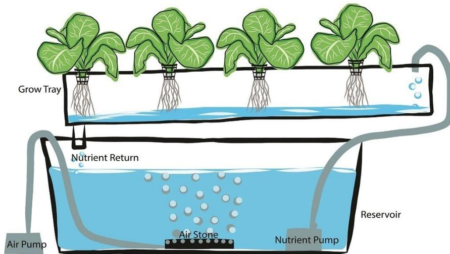
*Figure 2. A general overview of simple hydroponics system in which the water and required minerals are added to a water bed and pumped to medium for crop growth.*
