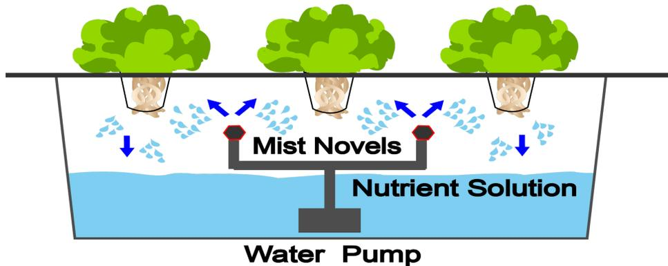
*Figure 4. A general overview of an aeroponics system where minerals and moisture are delivered to plants in a fixed frame.*
