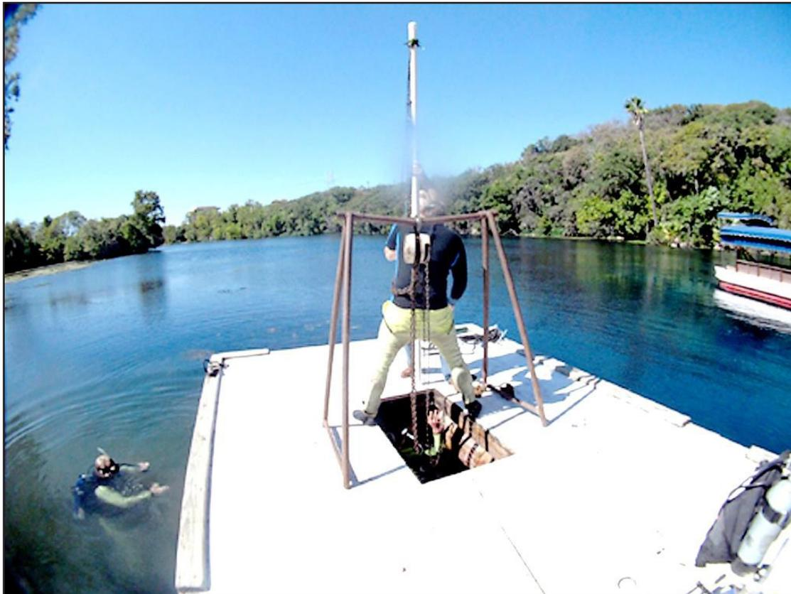
*Figure 13: Core being extracted using chain-hoist on barge.*
