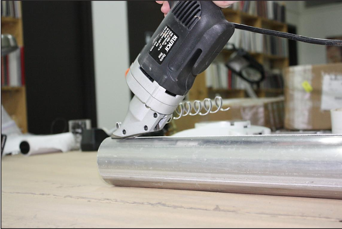
*Figure 15: Electric tin shears cutting aluminum core tube.*
