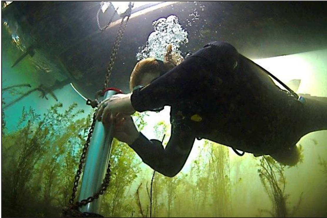
*Figure 14: Chain being secured to the driven core tube.*
