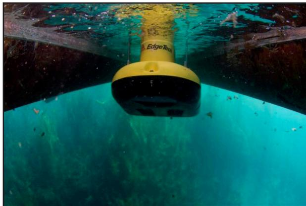
*Figure 8: Towfish deployed.*
