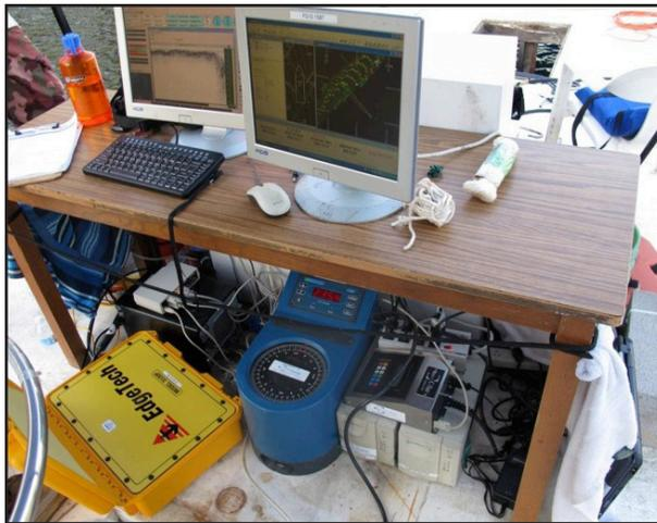
*Figure 6: The EdgeTech SB-424 subbottom profiling system.*
