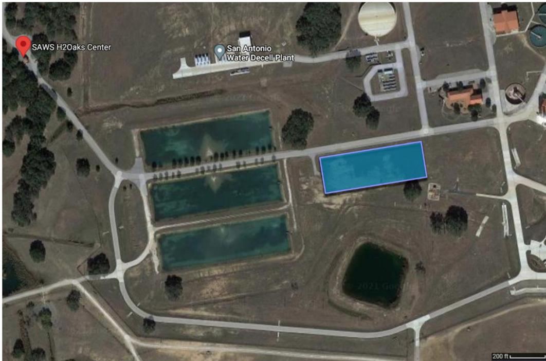
**Figure 5-2.** Estimated footprint (a blue rectangle: 600' × 200' × 2') of a full-scale photobioreactor for the SAWS H2Oaks Center
