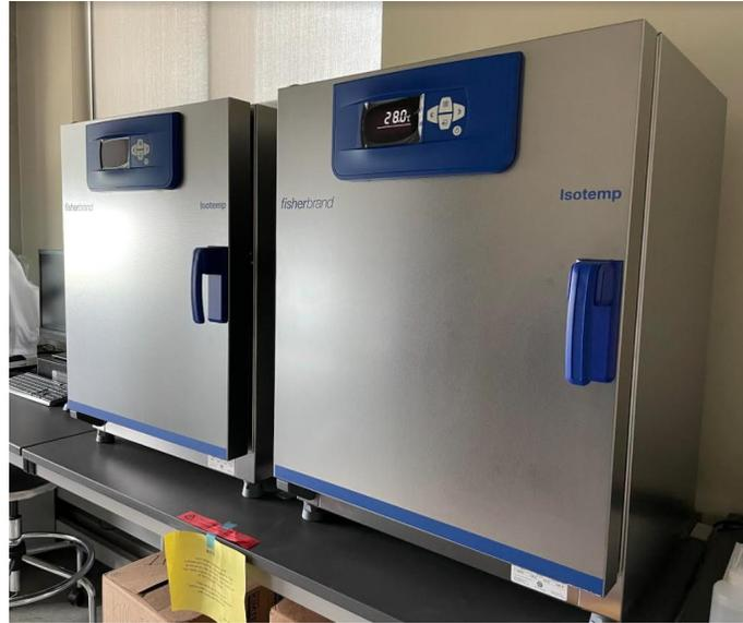
**Figure 3-5.** Non-refrigerated incubators
