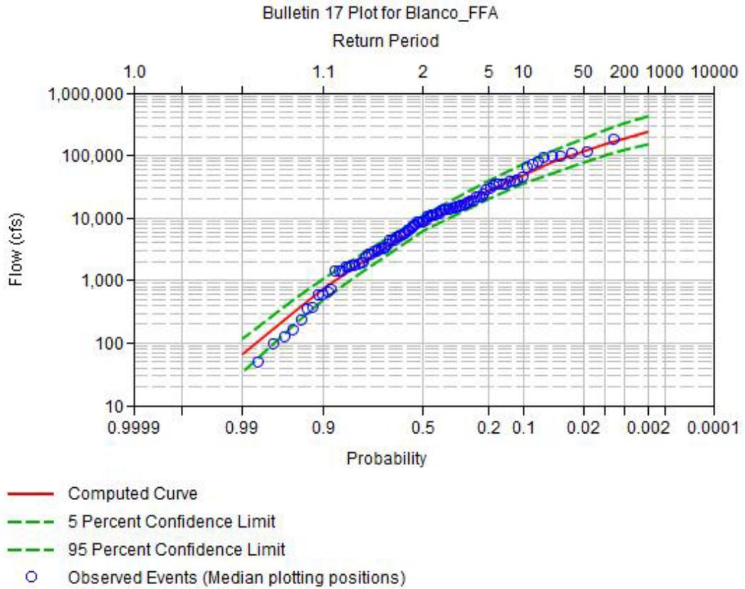
Figure 4: Flood-frequency analysis computed curve from HEC-SSP software
