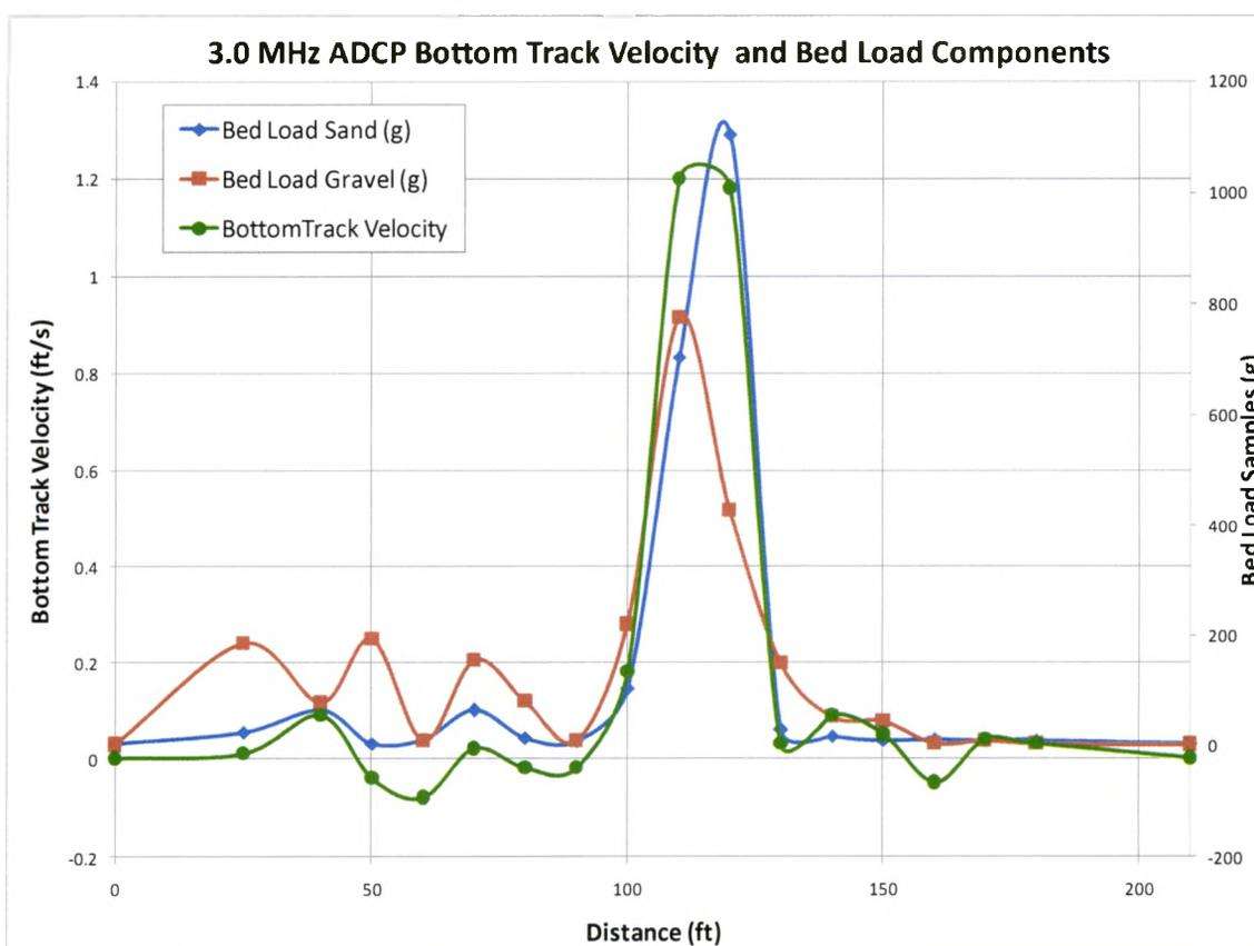
Figure 18. Chart showing how the different bed load components of gravel and sand varied with bottom track velocities throughout the cross-section during the 3.0 MHz ADCP measurement.
