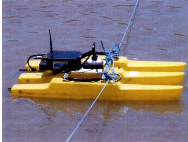
Figure 7 . SonTek ADCP mounted on an unmanned tethered trimaran (SonTek 2007).
