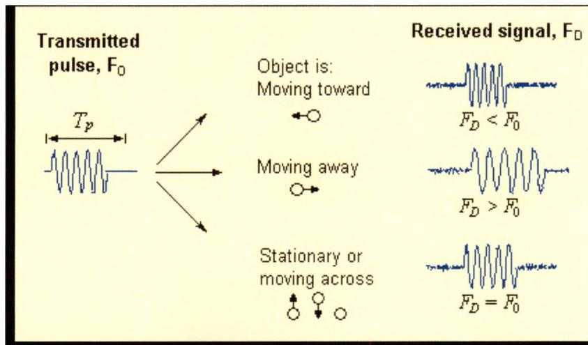
Figure 4. Illustration of the Doppler principal which shows how the transmitted pulse is shifted as an object is either moving away, towards, or stationary relative to the source (Sontek 2007).
