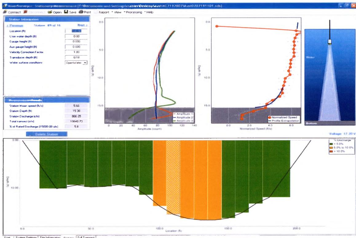
Figure 9. Output from the SonTek Stationary ADCP software illustrating the river channel separated into 20 to 25 sections in the lower image, with velocity profile and beam amplitude plots in the upper half (SonTek 2007).
