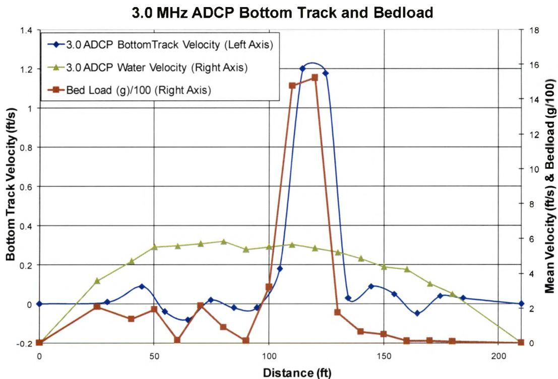
Figure 16. Chart showing how bottom track velocities, water velocities, and bed load varied throughout the cross-section during the 3.0 MHz ADCP measurement.
