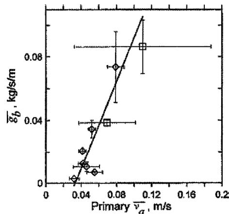
Figure 8. Bed load versus ADCP measured bed velocity plot from the Rennie et al. (2002) study.
