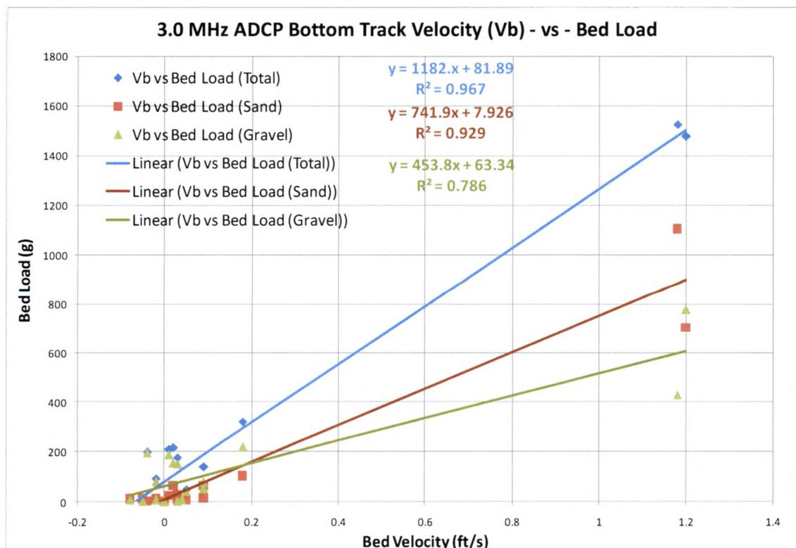
Figure 19. Linear regression lines demonstrating the relationships between the sand and gravel components of bed load captured during the 3.0 MHz ADCP measurement relative to bottom track velocity.
