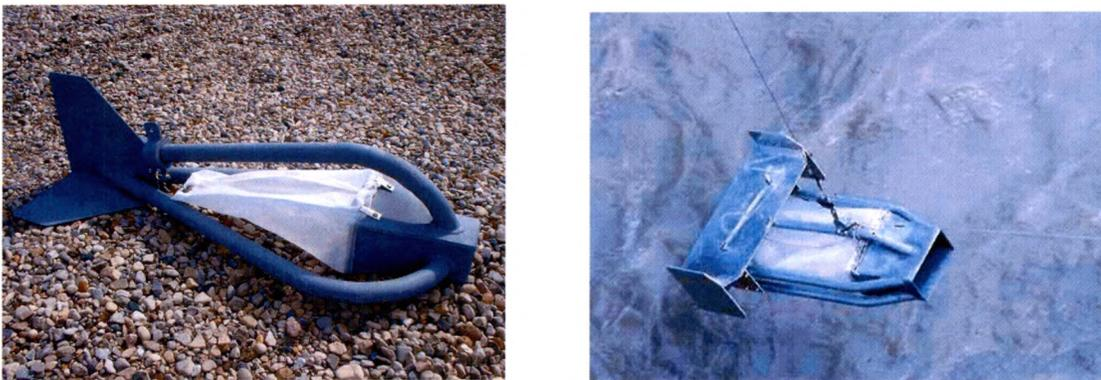
Figure 3. Pictures of the 195 pound model 8075 cable-suspended Helley-Smith (Left), and the 210 pound model 404-030 US-TR2 cable-suspended Toutle (Right) bed load sediment samplers (Rickly 2007).
