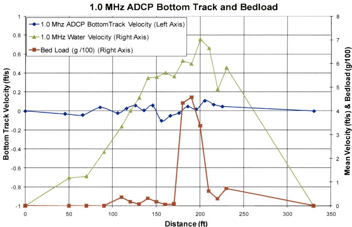
Figure 15. Chart showing how bottom track velocities, water velocities, and bed load varied throughout the cross-section during the 1.0 MHz ADCP measurement.
