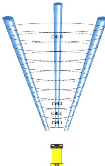
Figure 6. ADCP with a three beam setup, showing cell geometry (SonTek 2007).
