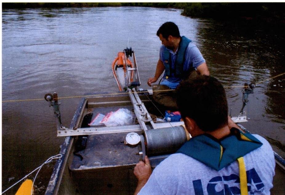
Figure 14. 16 ft boat and Helley-Smith sediment sampler setup with tagline during a measurement.
