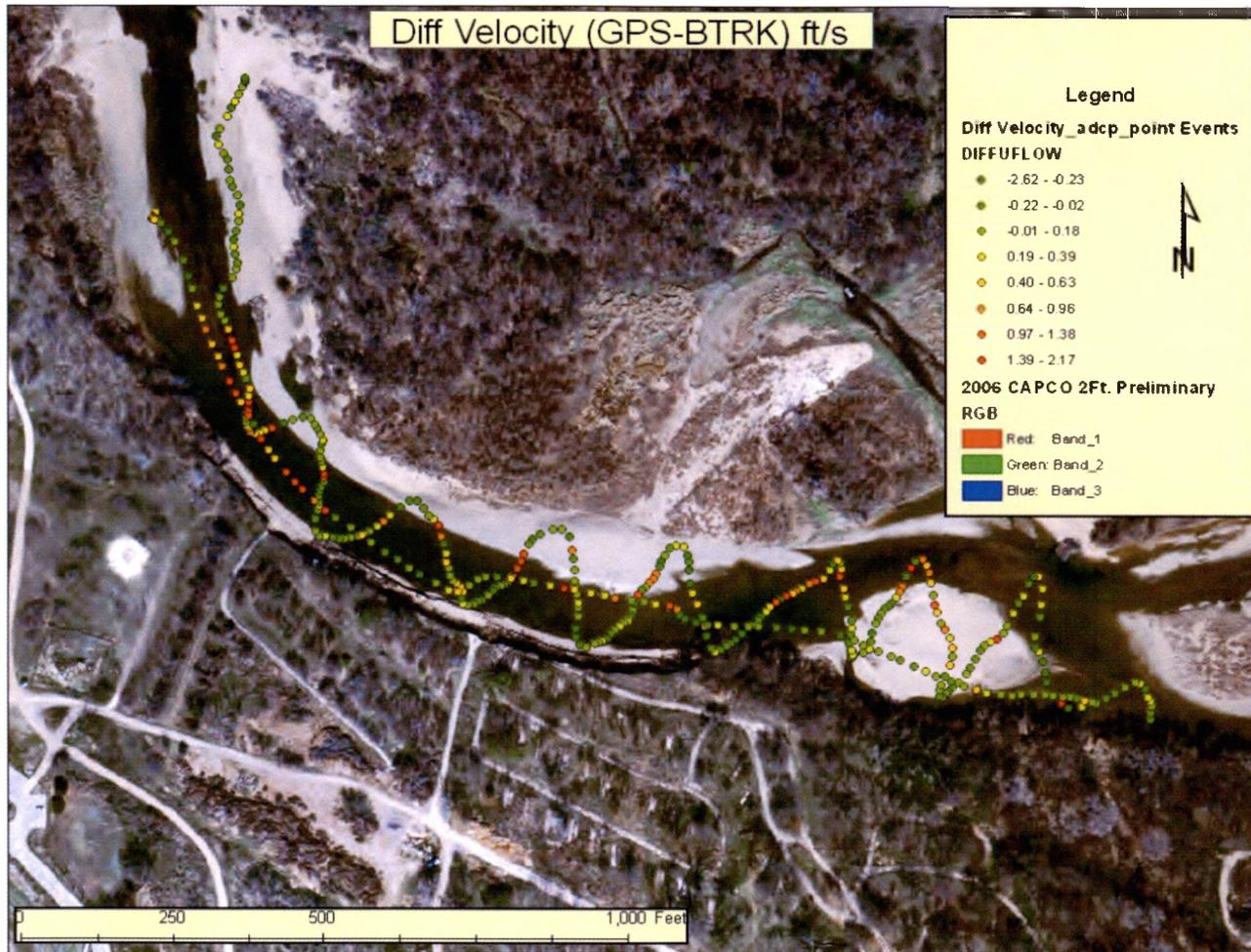
Figure 11. Aerial photo of the study site showing the ADCP path and bed load velocities (ft/s) using the Rennie et al. (2002) method.
