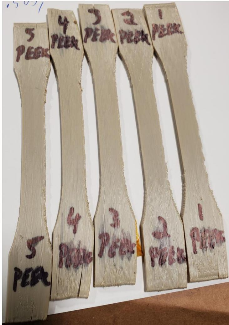
*Figure 166. PEEK on Edge (XZ) Tensile Specimens before Testing*
