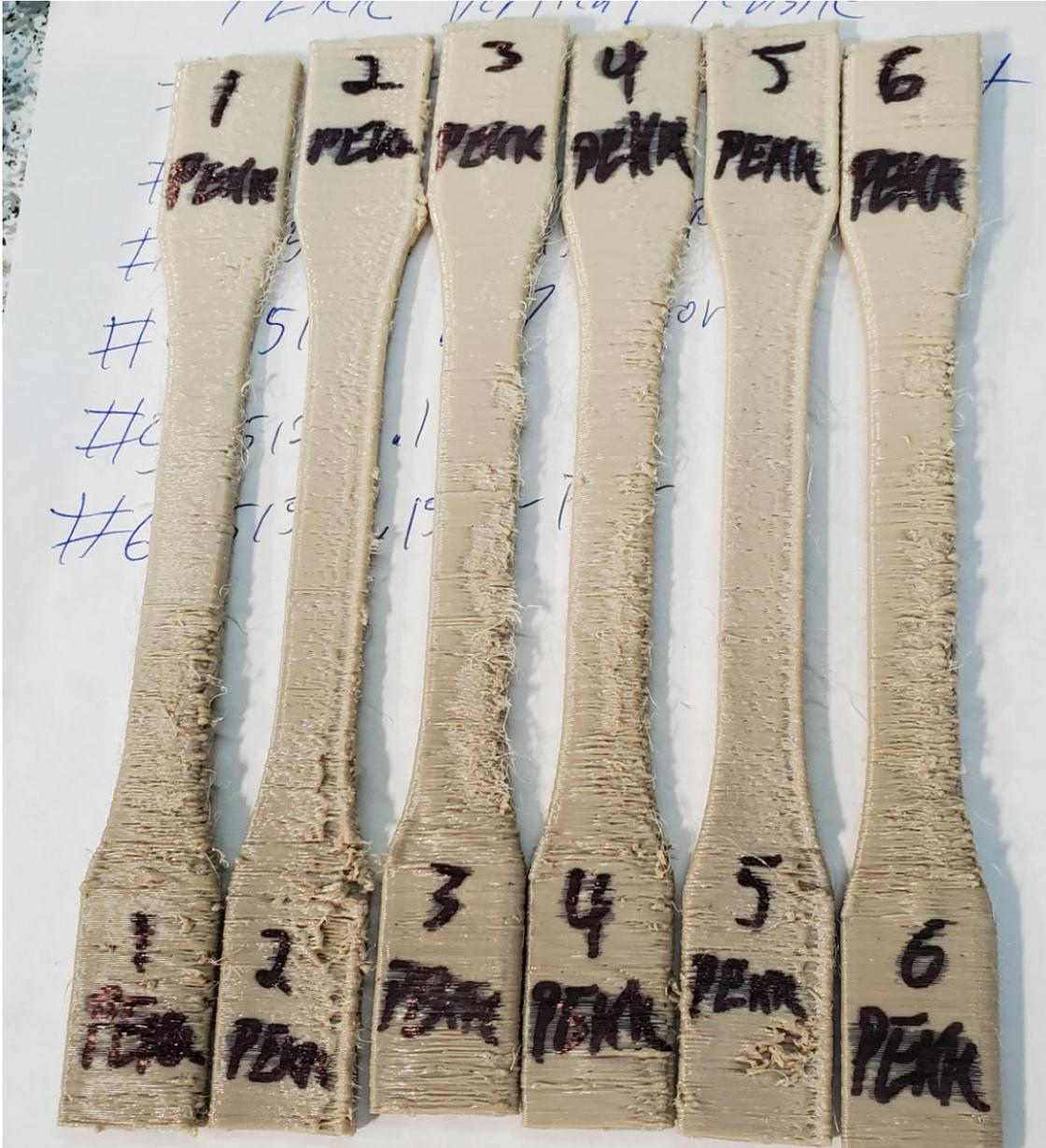
*Figure 112. PEKK Upright (ZX) Tensile Specimens before Testing*
