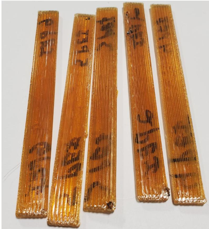
*Figure 148. PEI Ultem 1010 Flat (XY) Flexural Specimens before Testing*
