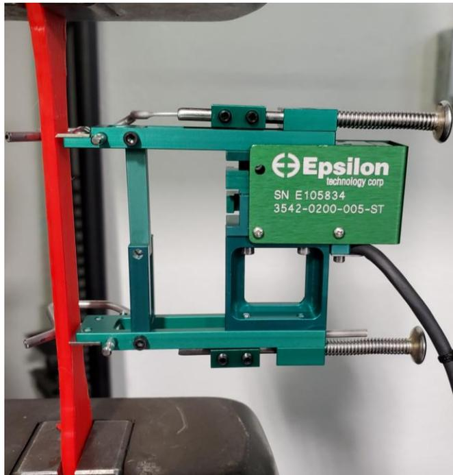
*Figure 60. Axial extensometer model 3542 from Epsilon that was used to Measure the Tensile Strain*
