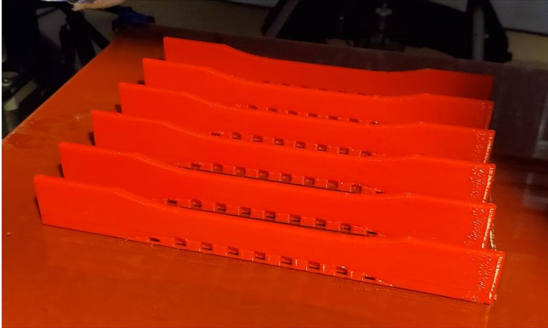
***Figure 33. Printed PLA Tensile Specimens on the Edge (XZ)***
