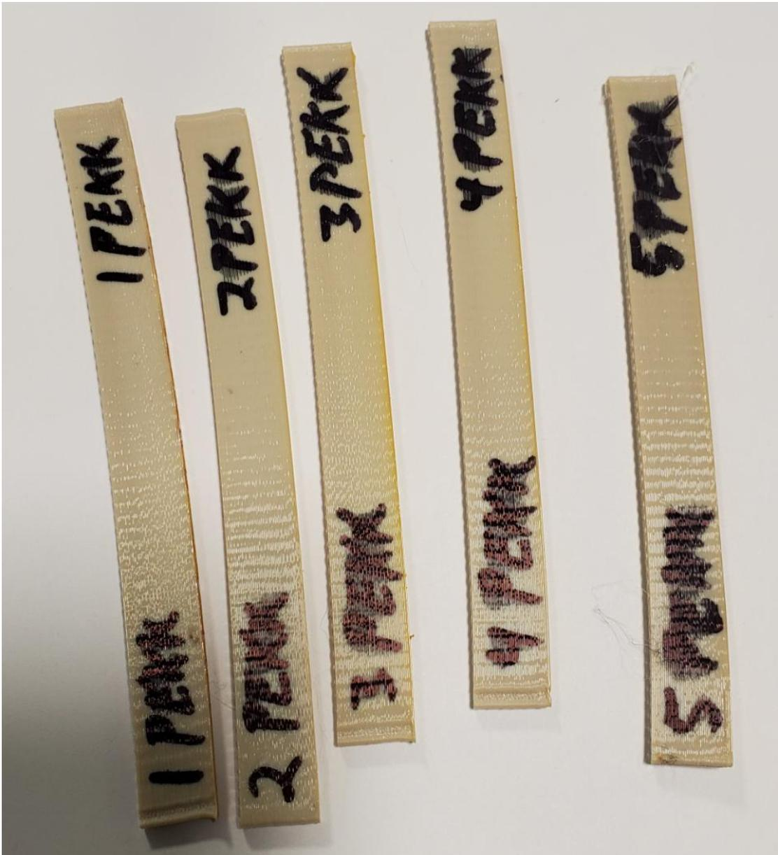
*Figure 122. PEKK on Edge (XZ) Flexural Specimens before Testing*
