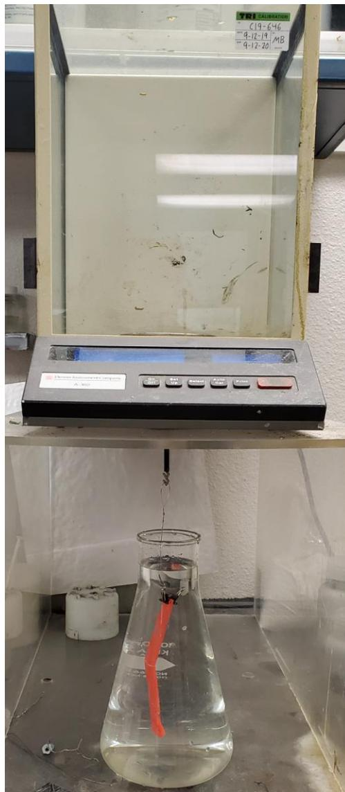
**Figure 182. Measuring the Weight in Water to Calculate Density**
