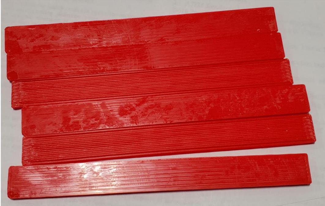
*Figure 86. PLA Flat (XY) Flexural Specimens*
