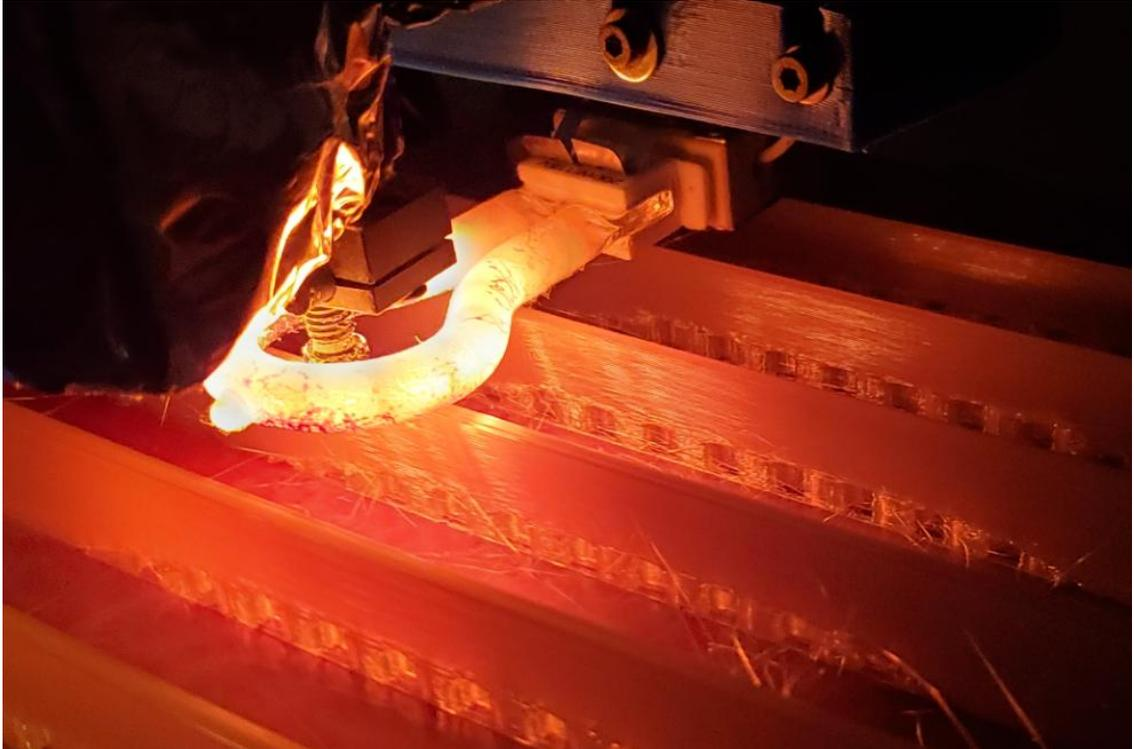
*Figure 39. Printing PEKK Tensile Specimens on the Edge (XZ) Image 2*
