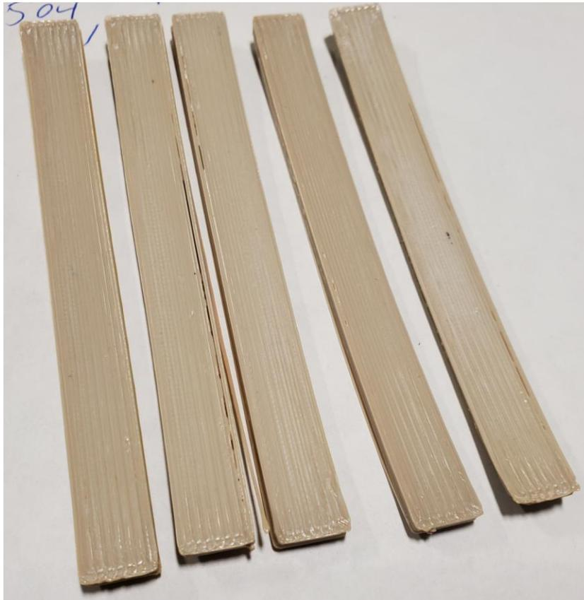
***Figure 173. PEEK Flat (XY) Flexural Test Specimens before Testing***
