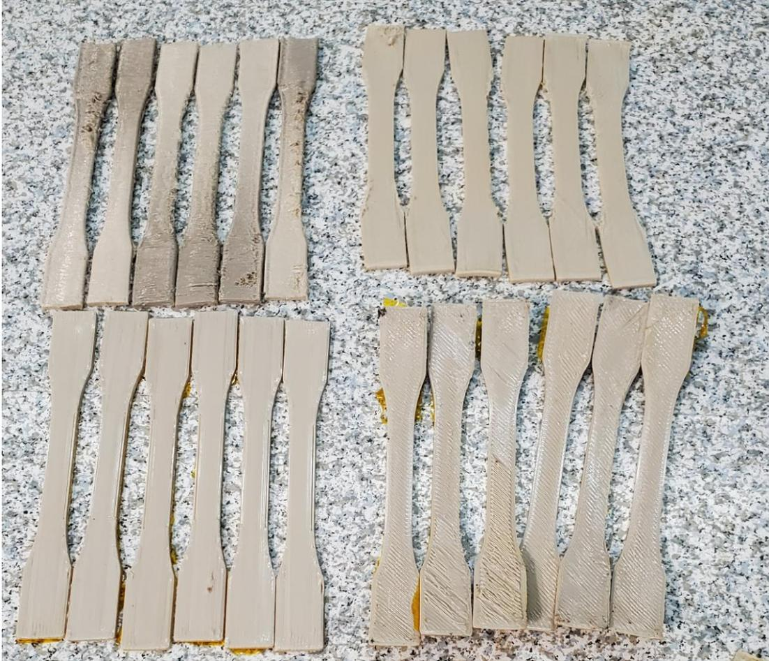
*Figure 101. PEKK Tensile Specimens*
