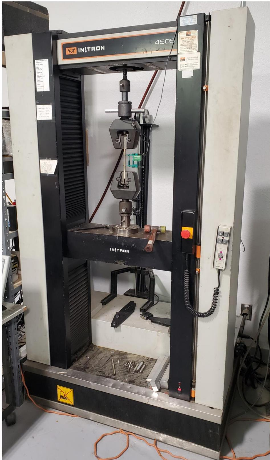
*Figure 59. 4505 Series Instron Test Frame used for Tensile and Flexural Testing.*
