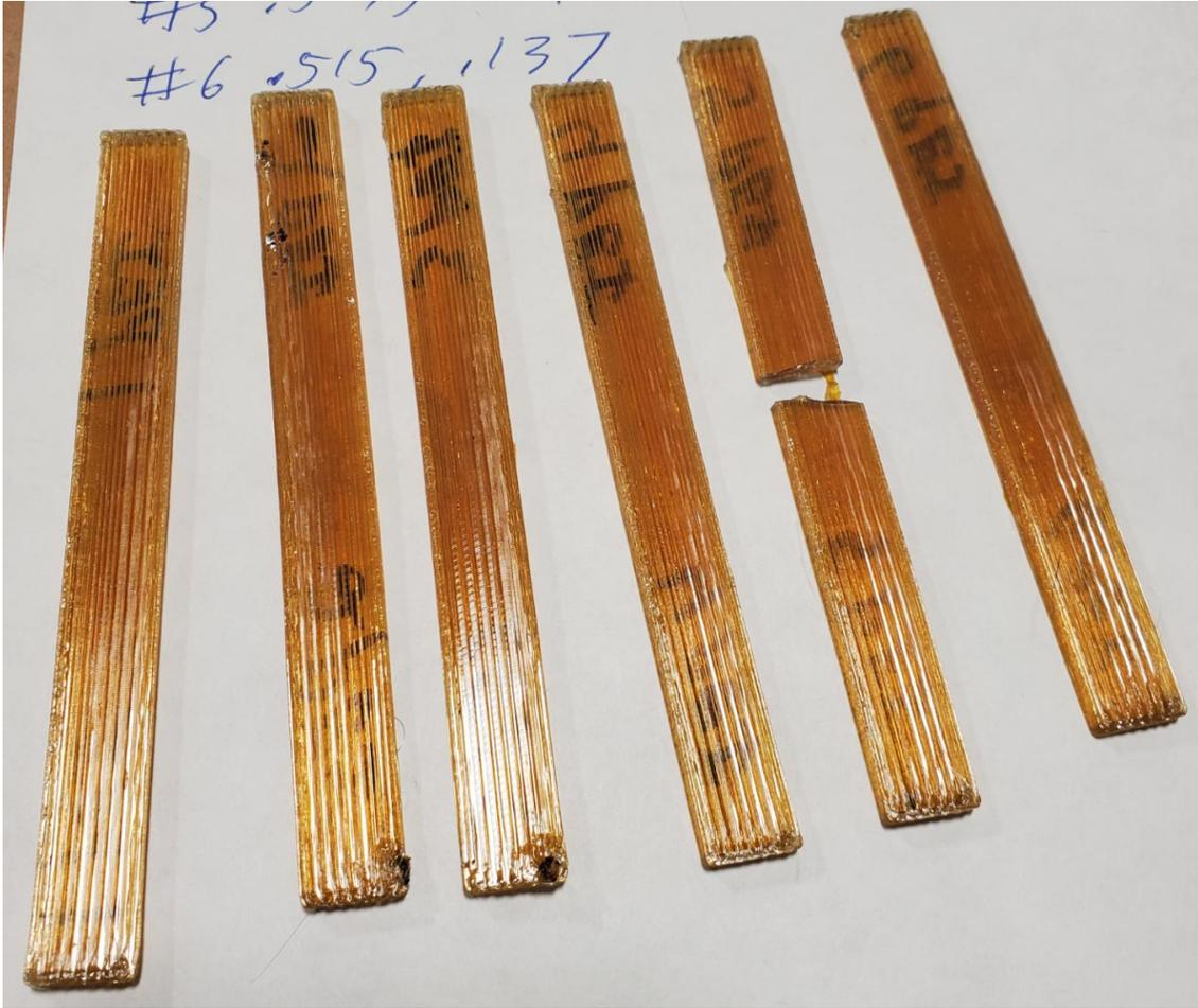
*Figure 149. PEI Ultem 1010 Flat (XY) Flexural Specimens after Testing*
