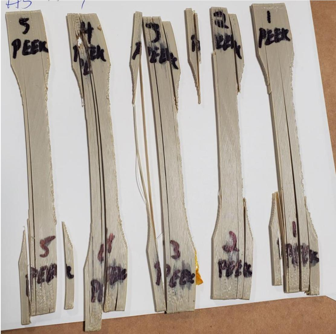
Figure 167. PEEK on Edge (XZ) Tensile Specimens after Testing
