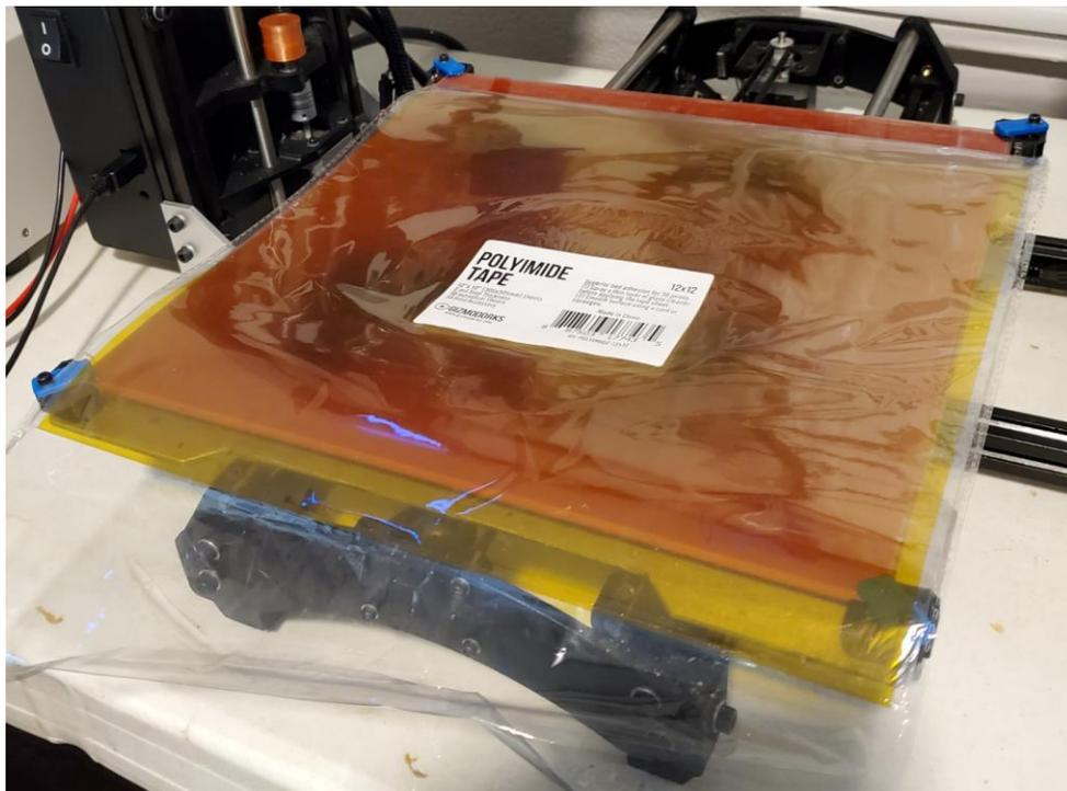
*Figure 28. Kapton Polyimide Tape to Stick Parts to Print Bed*
