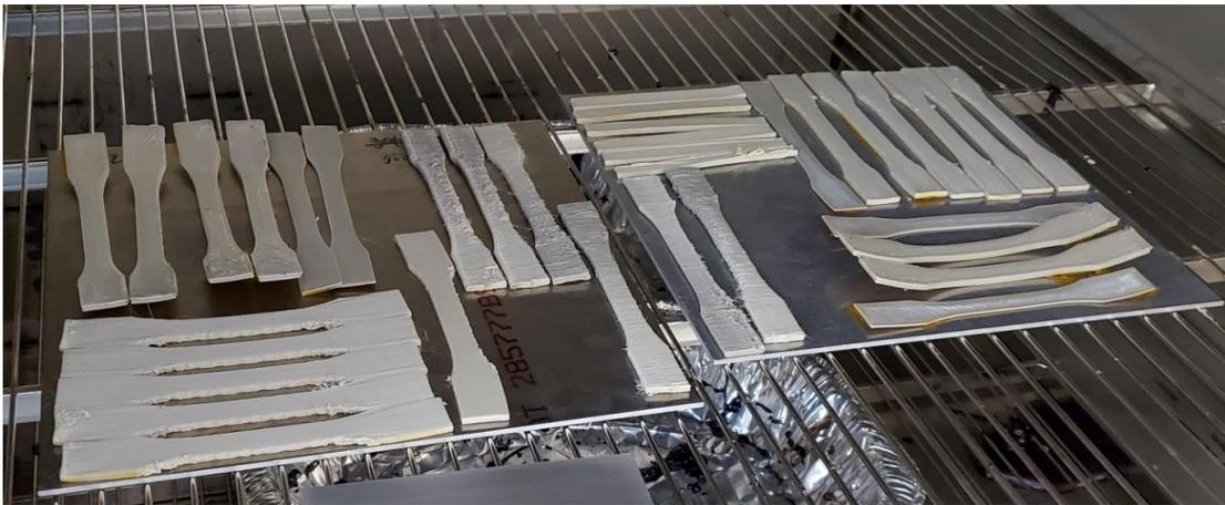
*Figure 100. Annealing PEKK Specimens*
