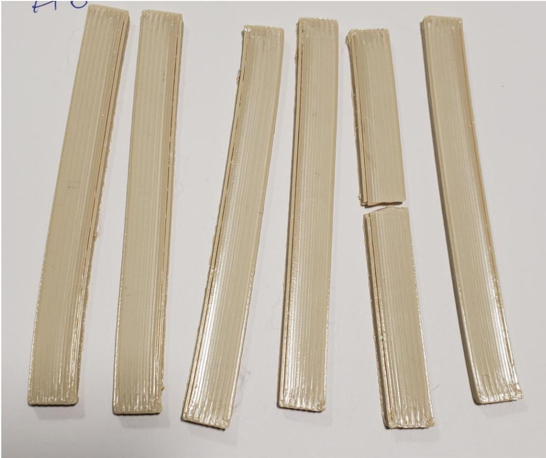
*Figure 120. PEKK Flat (XY) Flexural Specimens after Testing*
