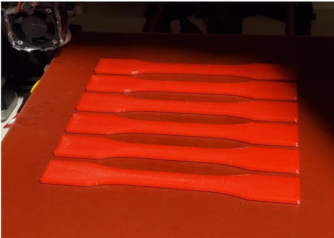
*Figure 32. Printed Flat (XY) PLA Tensile Specimens*
