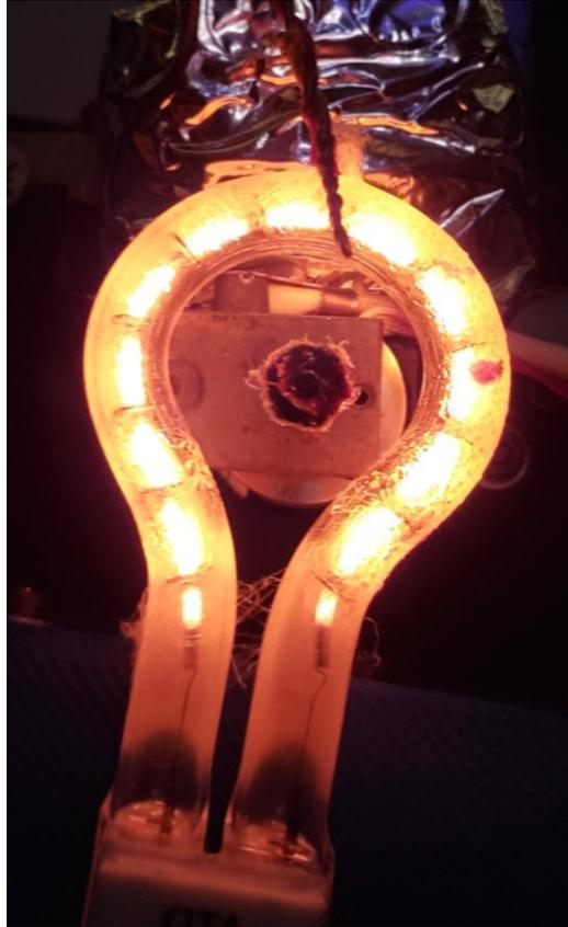
*Figure 11. Looking up at the Infrared Heat Lamp and the Bottom of the Nozzle*
