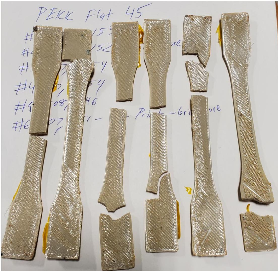
Figure 107. PEKK Flat (XY)  $\pm 45^\circ$  Infill Tensile Specimens after Testing
