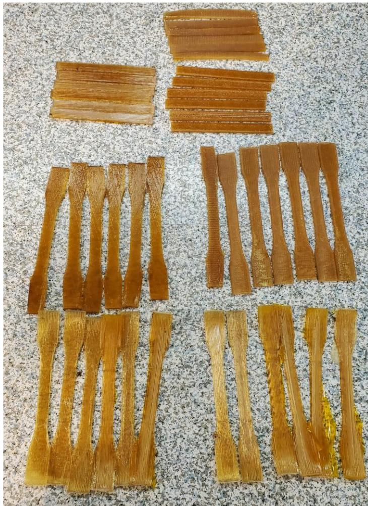
***Figure 133. PEI Tensile and Flexural Test Specimens***
