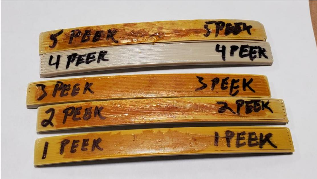
Figure 174. PEEK Flat (XY) Flexural Test Specimens after Testing
