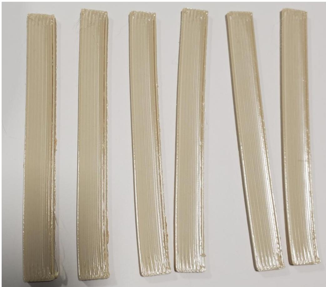
*Figure 119. PEKK Flat (XY) Flexural Specimens before Testing*
