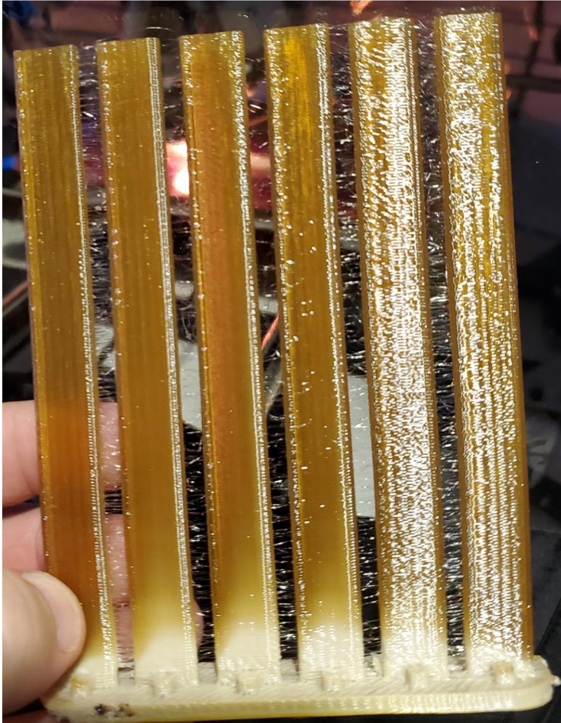
*Figure 45. Printing PEKK Upright (ZX) Flexural Specimens Image 2*
