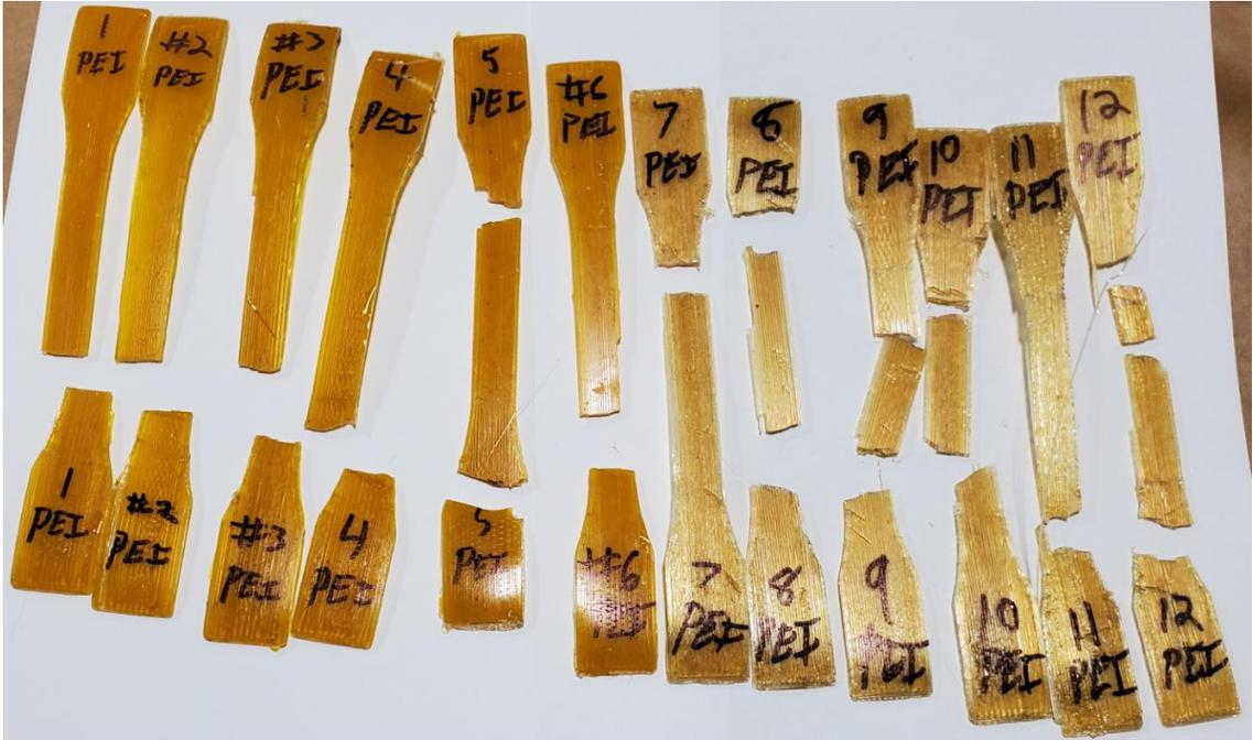
Figure 136. PEI Ultem 1010 Flat (XY) Tensile Specimens after Testing
