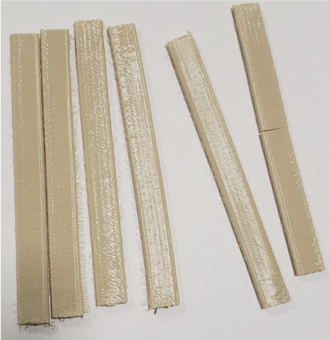
*Figure 125. PEKK Upright (ZX) Flexural Specimens*
