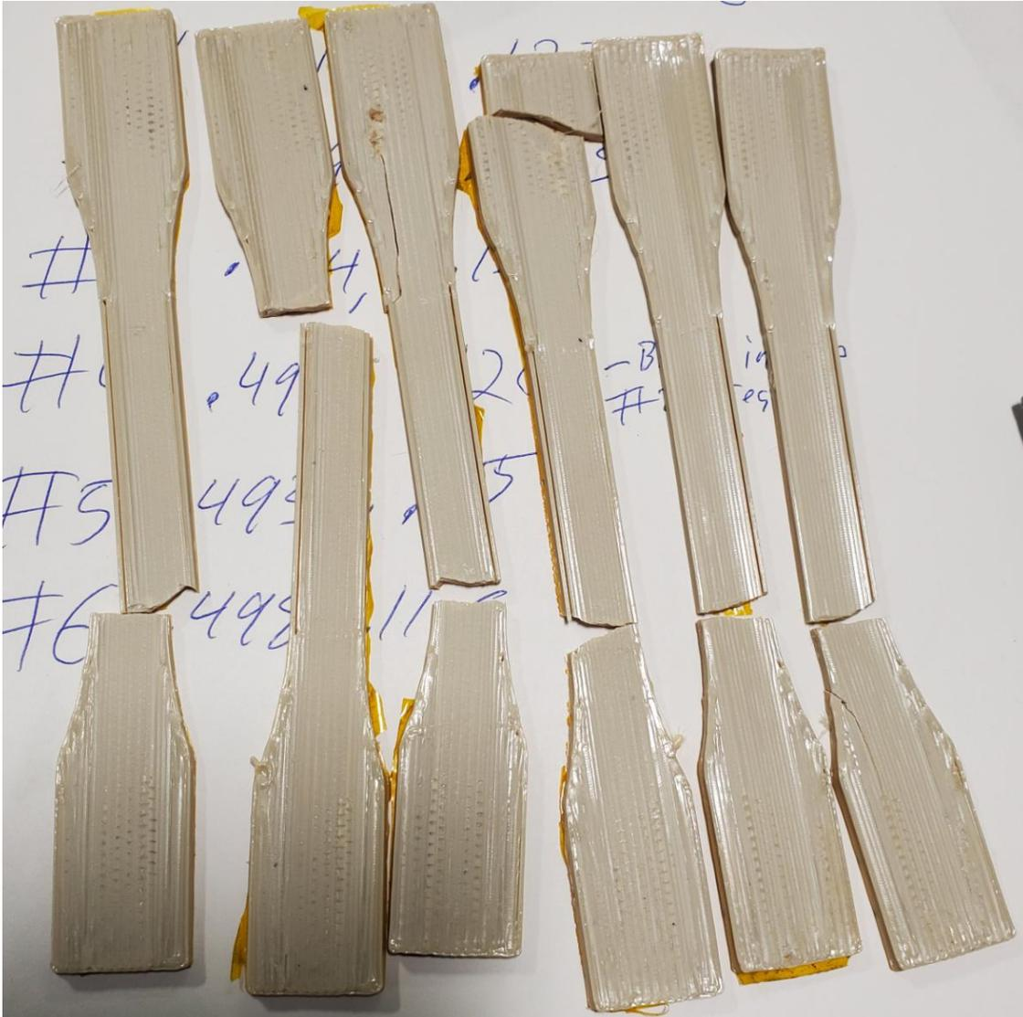
**Figure 104. PEKK Flat (XY) Tensile Specimens after Testing**
