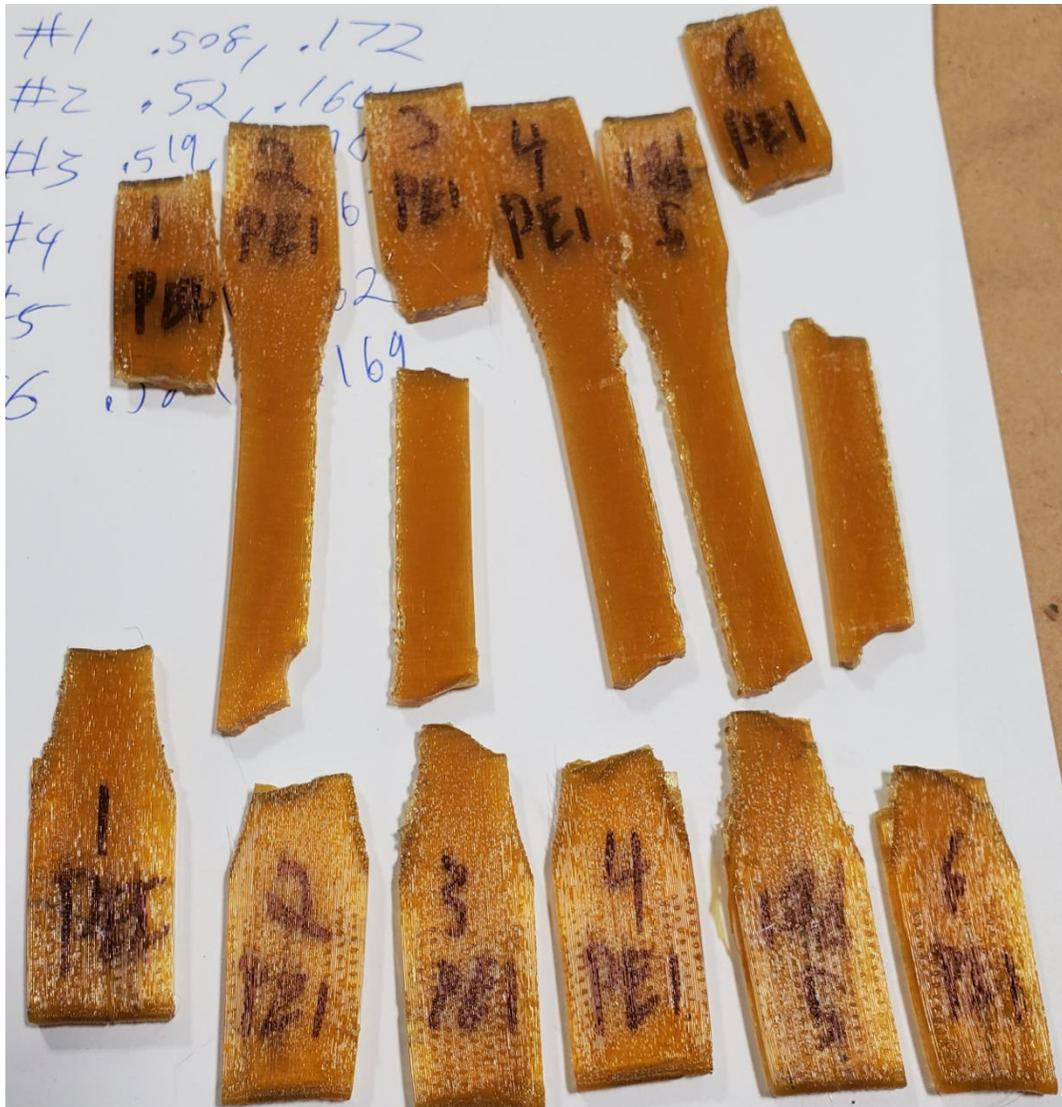
**Figure 139. PEI Ultem 1010 on Edge (XZ) Tensile Specimens after Testing**
