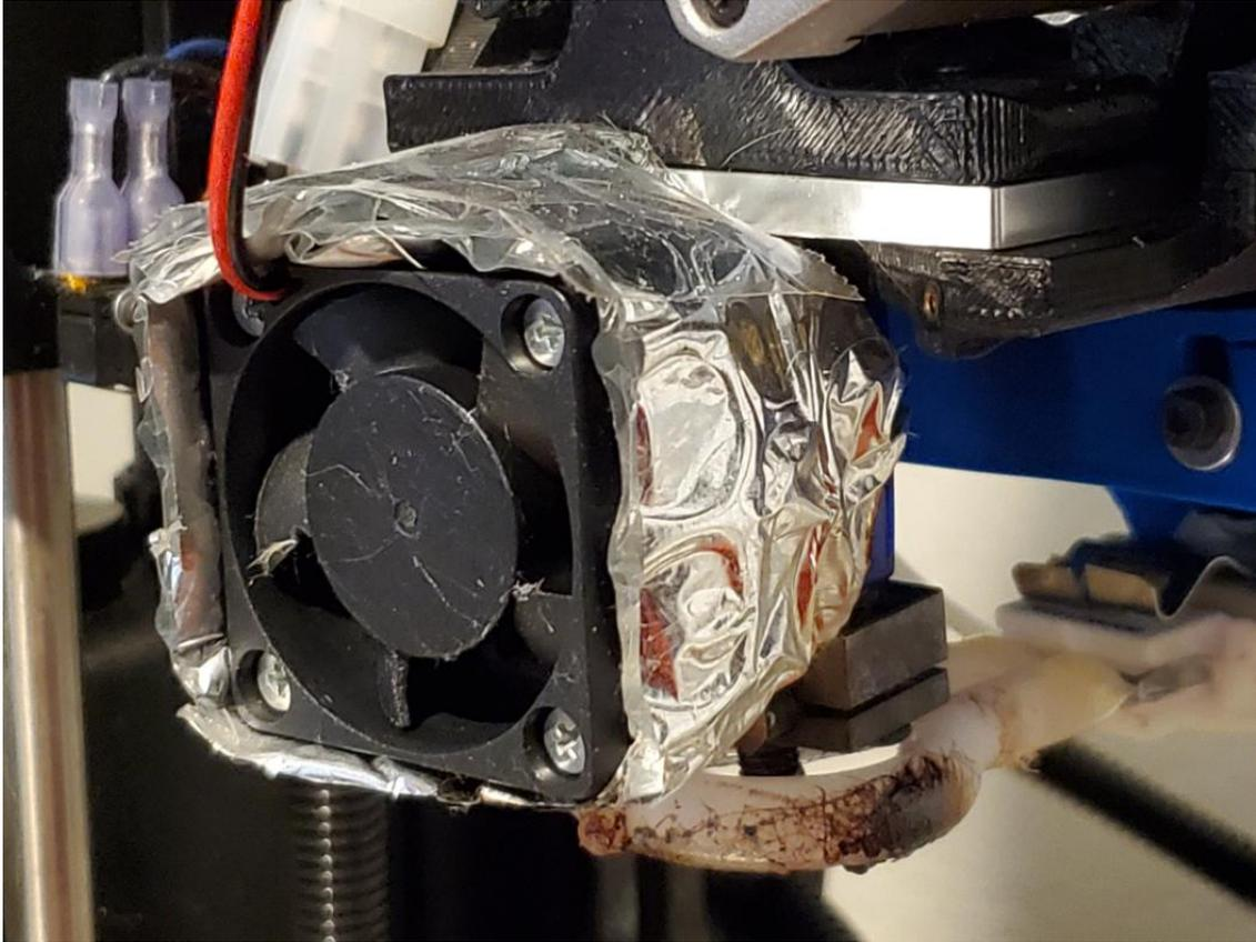
*Figure 6. Hot End Cooling Fan with Insulation to Protect it from the heat from the Infrared Light*
