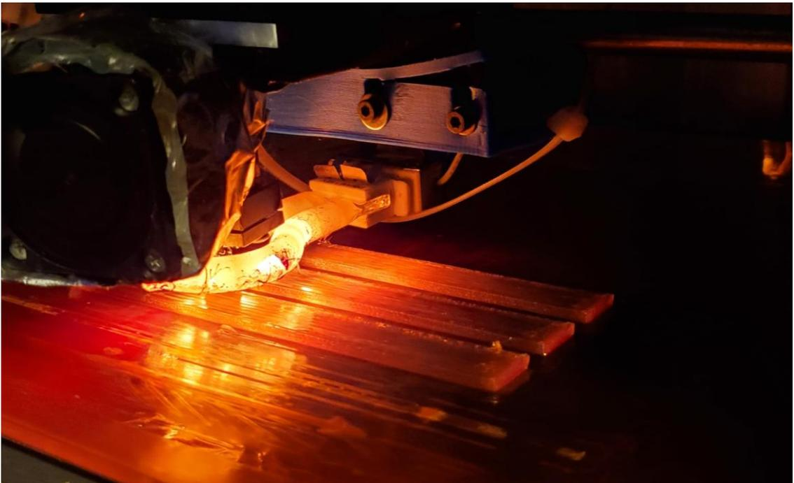
*Figure 50. Printing PEI Flat (XY) Flexural Specimens*
