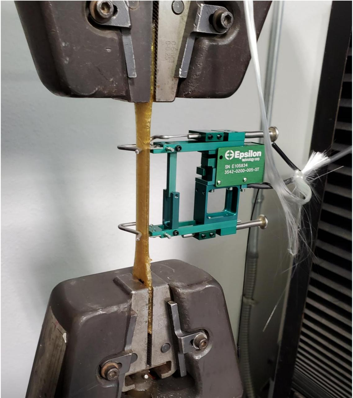
*Figure 134. PEI Tensile Testing*
