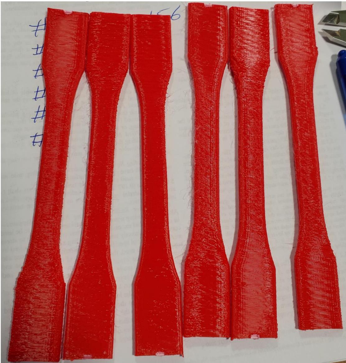
***Figure 79. PLA Upright (ZX) Tensile Specimens Printed with Heat Lamp at 60°C before Testing***
