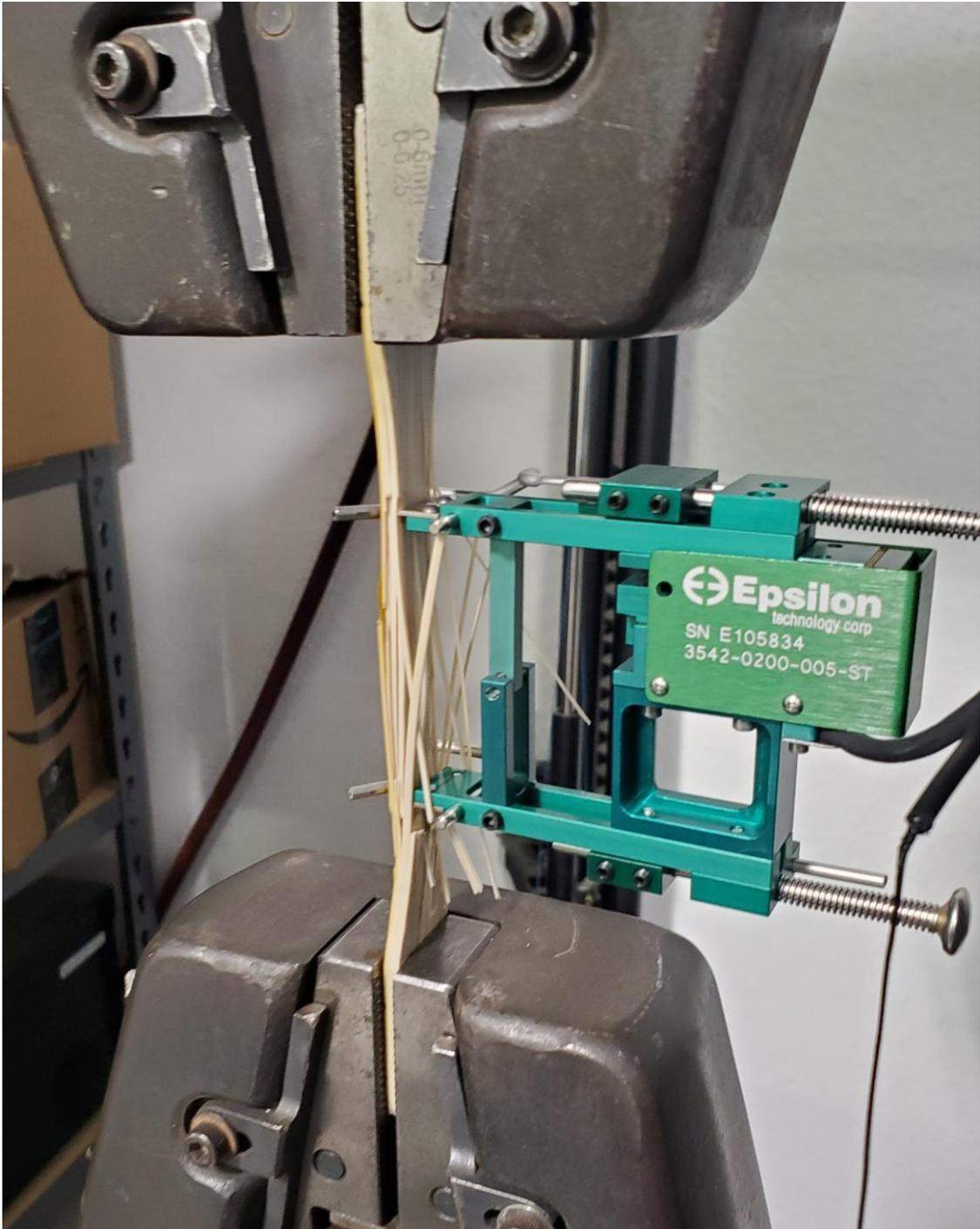
*Figure 163. PEEK Flat (XY) Tensile Specimen after Testing*
