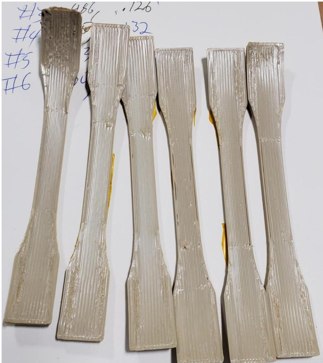
**Figure 162. PEEK Flat (XY) Tensile Specimens before Testing**
