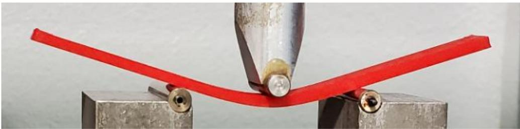
*Figure 62. Flexural Testing Setup*
