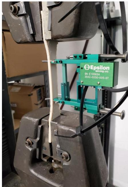
*Figure 102. Testing PEKK Tensile Specimen*
