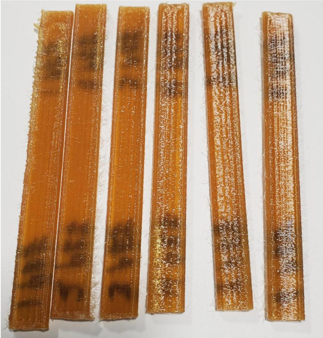
*Figure 153. PEI Ultem 1010 Upright (ZX) Flexural Specimens before Testing*
