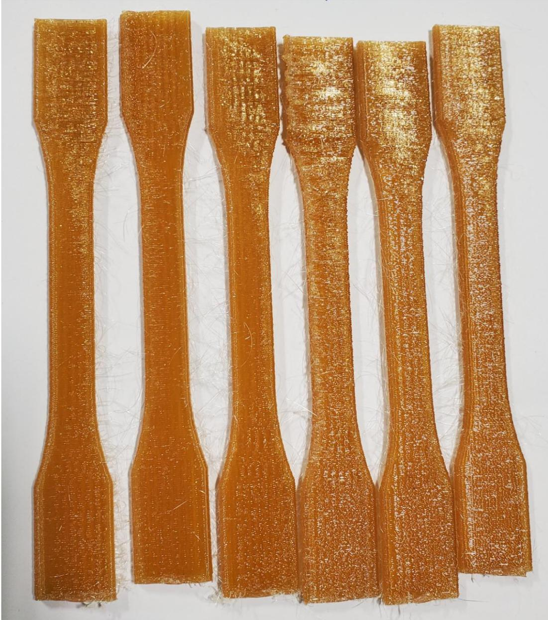
***Figure 141. PEI Ultem 1010 Upright (ZX) Tensile Specimens before Testing***
