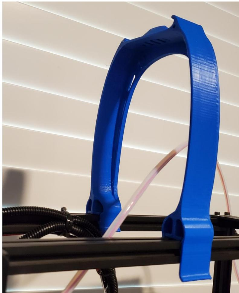
*Figure 20. Installed Mounting Bracket for Enclosure*
