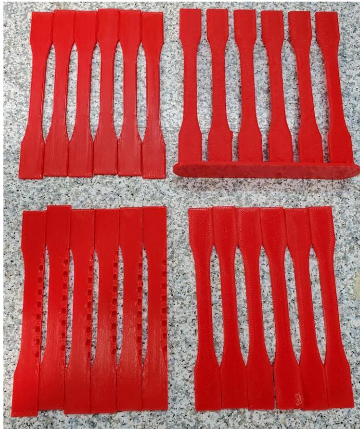
*Figure 63. PLA Tensile Test Specimens, Flat (XY), Upright (ZX), on Edge (XZ), and Flat  $\pm 45^\circ$  Infill (XY)*
