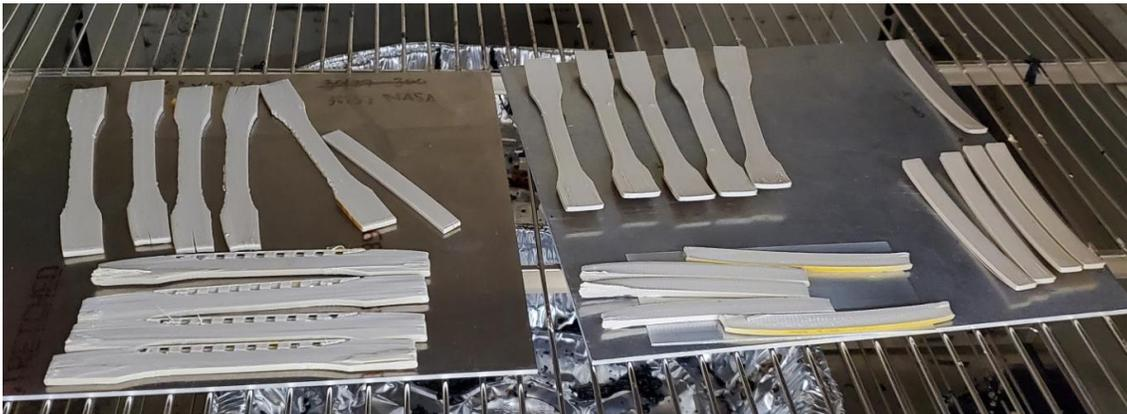
*Figure 161. PEEK Test Specimen Annealing*
