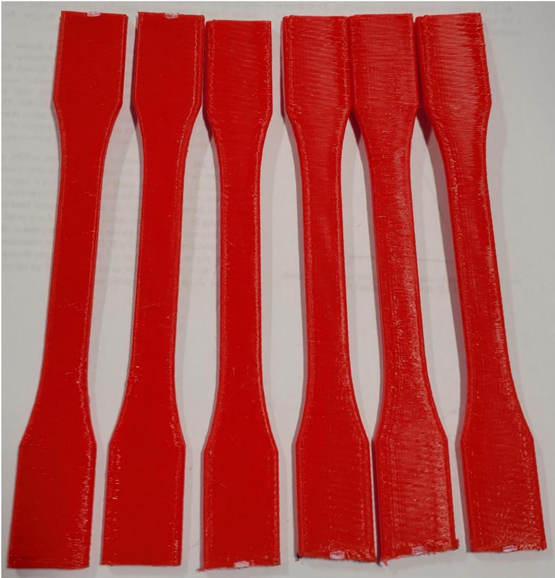
***Figure 76. PLA Upright (ZX) Tensile Specimens Printed at Room Temperature before Testing***
