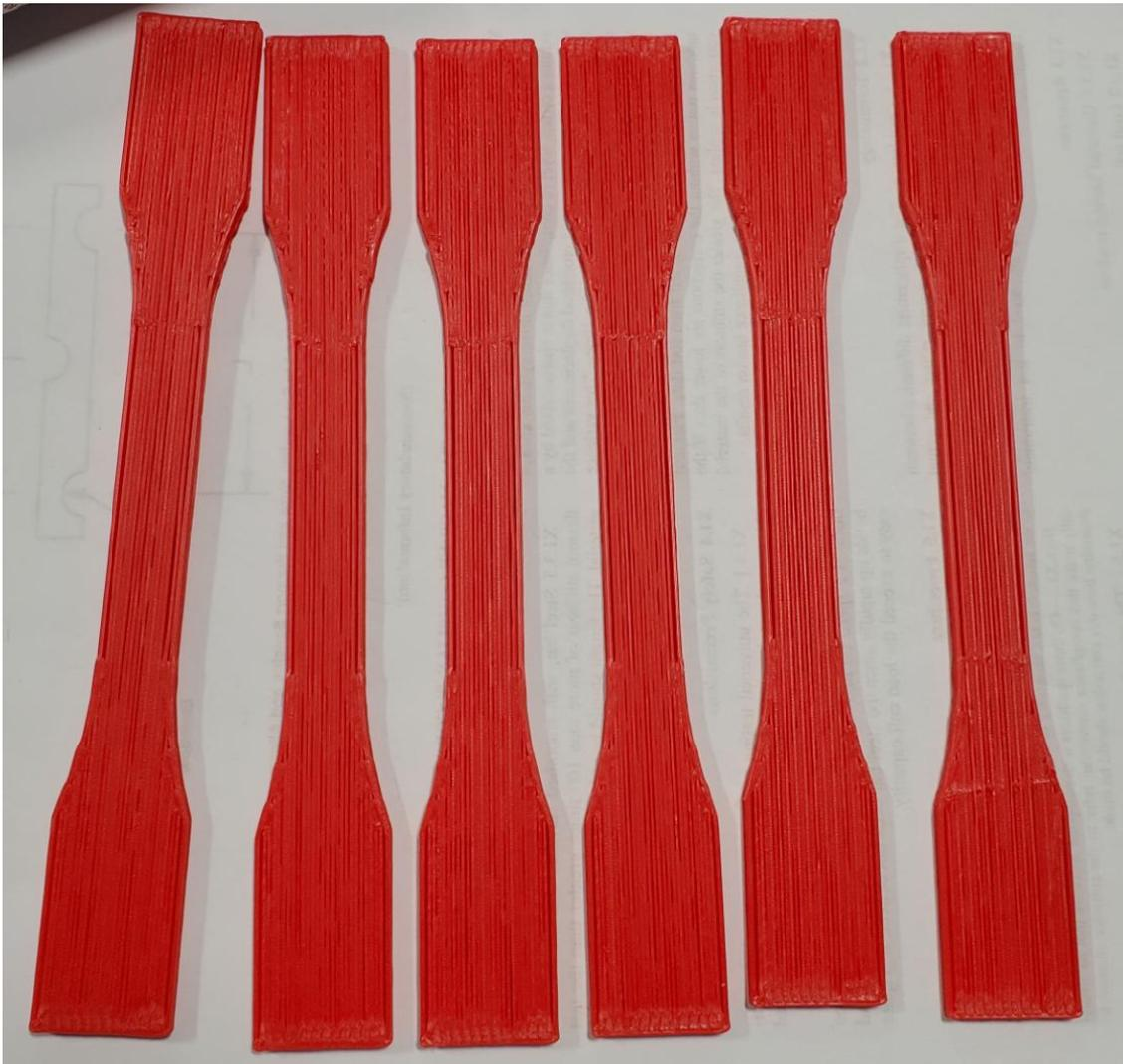
***Figure 64. PLA Flat (XY) Tensile Specimens***
