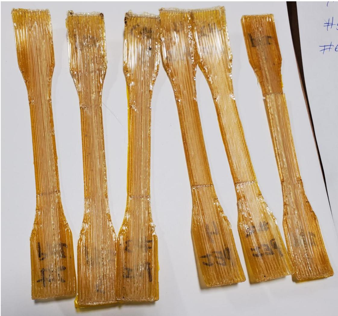
*Figure 135. PEI Ultem 1010 Flat (XY) Tensile Specimens before Testing*
