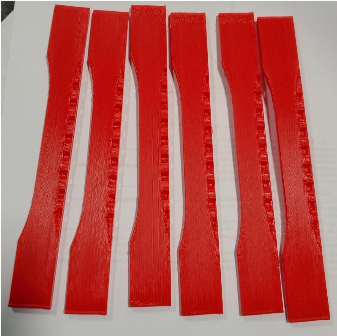
***Figure 71. PLA on Edge (XZ) Tensile Specimens before Testing and Removing the Printing Supports***
