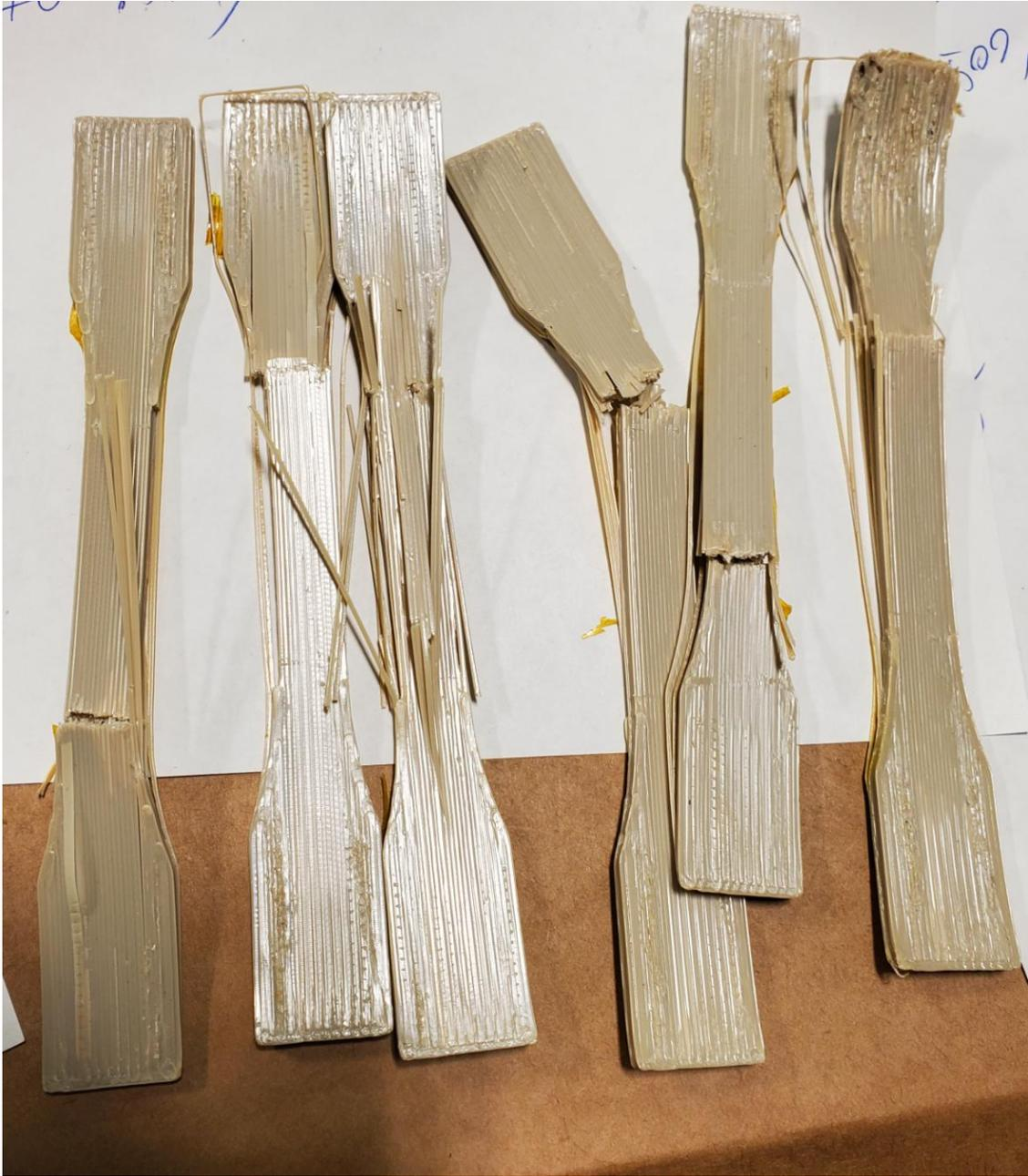
*Figure 164. PEEK Flat (XY) Tensile Specimens after Testing*
