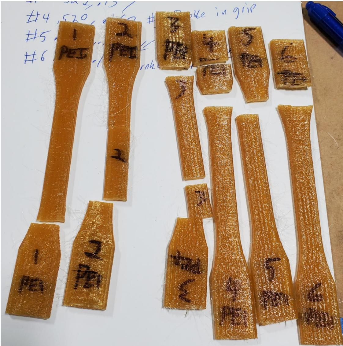
**Figure 142. PEI Ultem 1010 Upright (ZX) Tensile Specimens after Testing**
