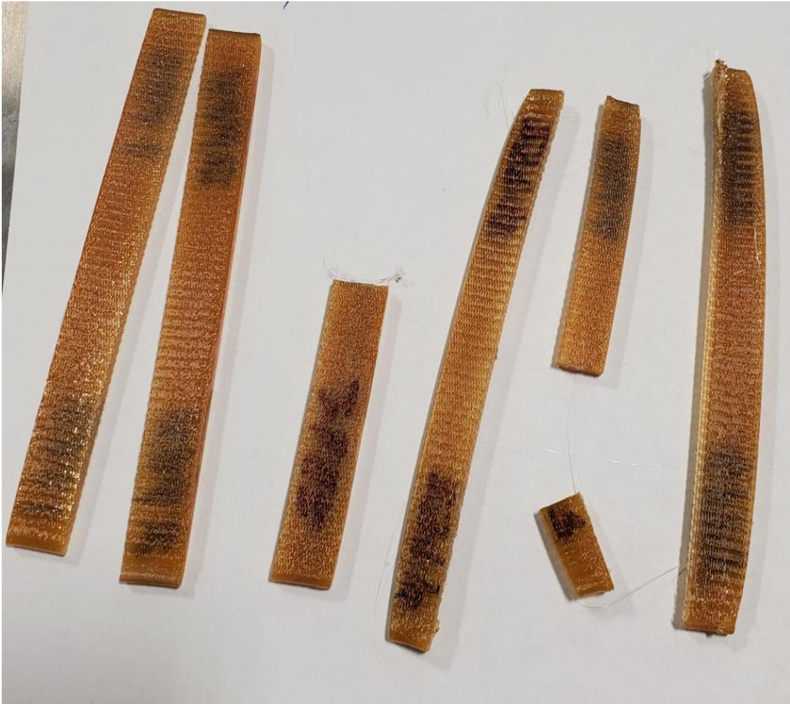
*Figure 151. PEI Ultem 1010 on Edge (XZ) Flexural Specimens*
