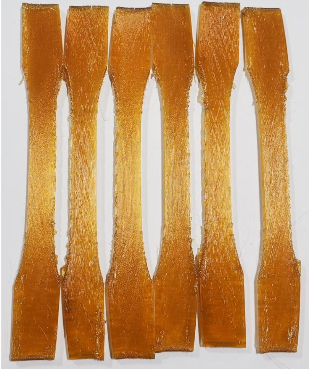
*Figure 138. PEI Ultem 1010 on Edge (XZ) Tensile Specimens before Testing*
