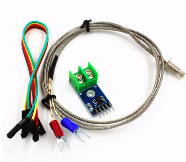
Figure 7.7: MAX6675 temperature sensor used to build the CPS testbed.
