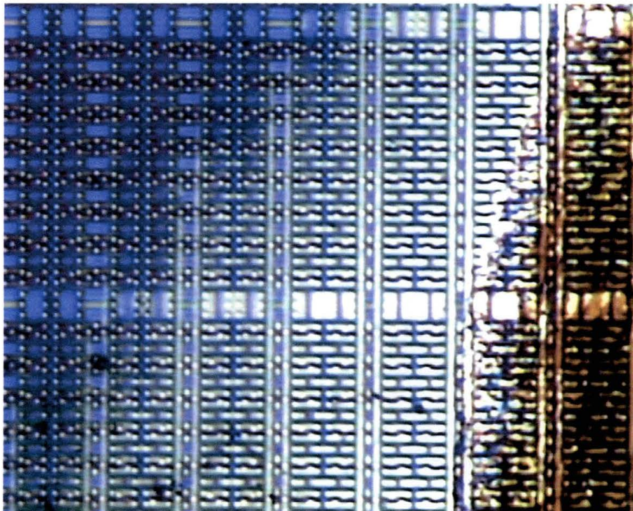
Figure 4.18 Polishing front removing metal 1 as it
