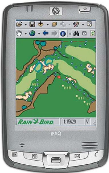
**Figure 21. Golf Irrigation Mobile Controller (Rainbird 2010)**
