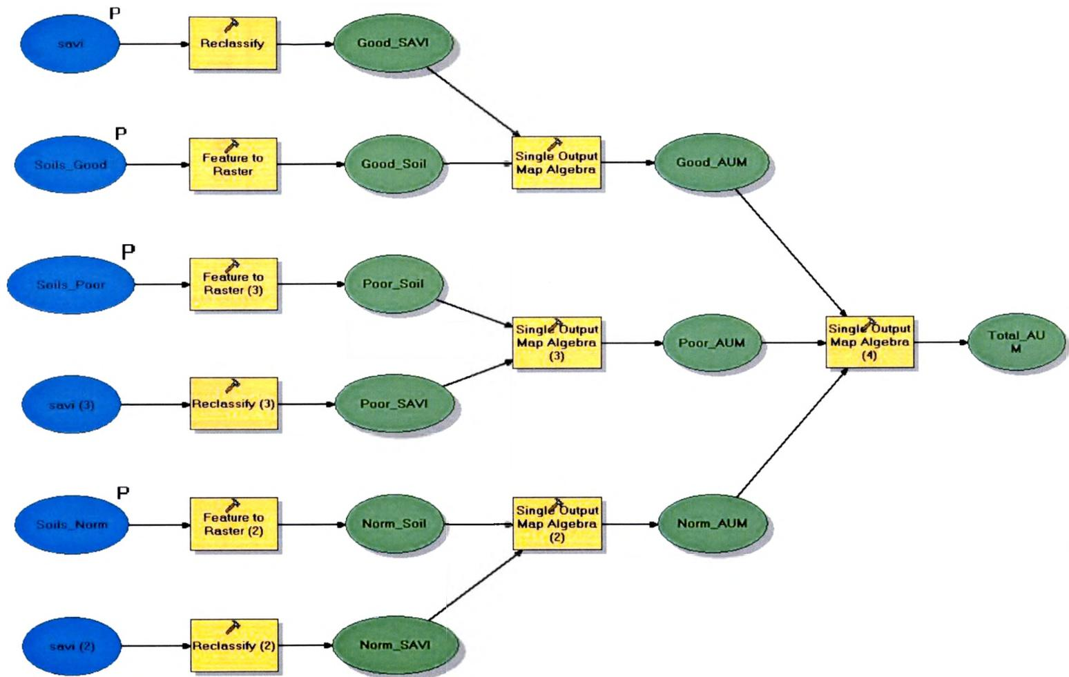
Figure 6. AUM model in ArcGIS 9 model builder
