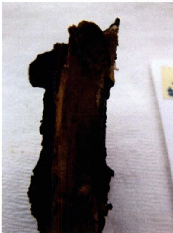
*(Figure 71) Internal surface of rib from Dry-Chemical remains showing the jagged fracture edge observed during laboratory analysis.*
