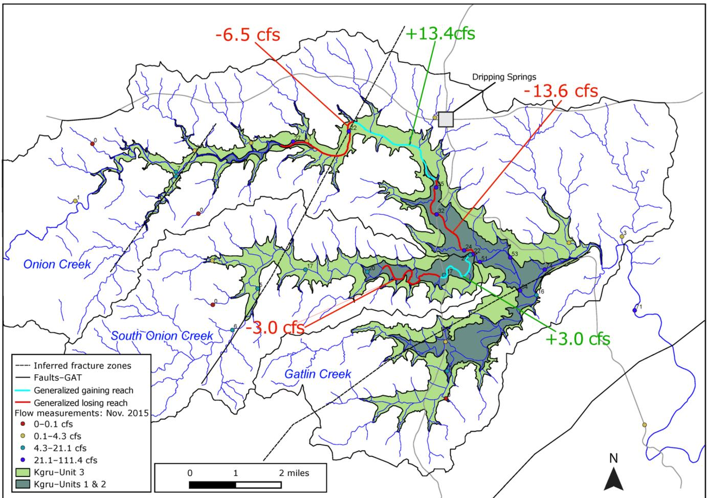
Figure 11. Geologic map with November 2015 gain/loss data from Hunt et al. (2016) overlaid. Prominent losing stream reaches occur in areas where unit 3 has been fully incised.
