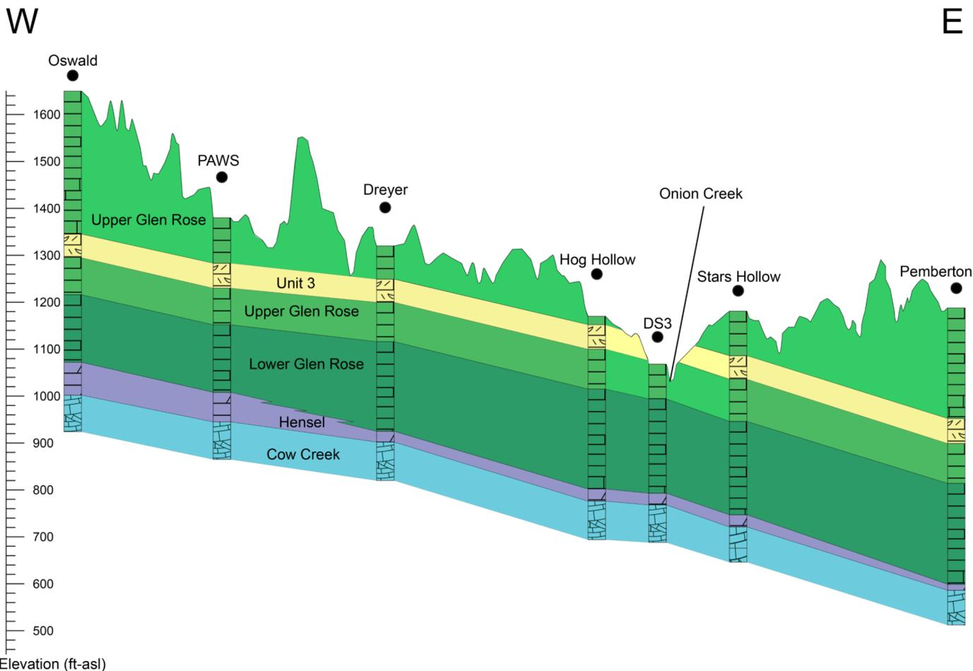
**Figure 9. Structural cross-section A–A'.** Areas where unit 3 has been fully incised are shown in map view in [Figure 10](#) (dark green).
