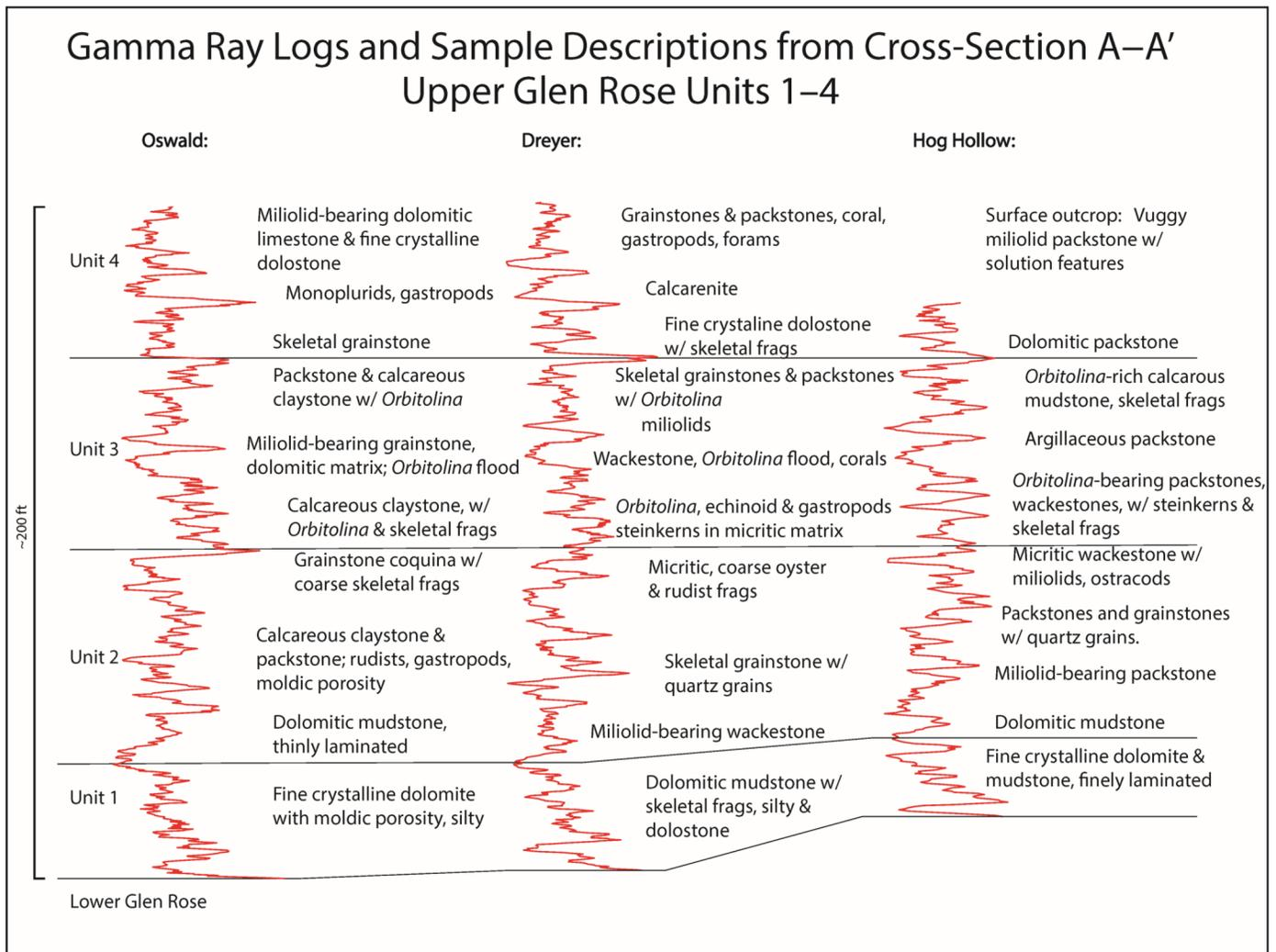
Figure 4. Subsurface correlation of gamma ray logs.
