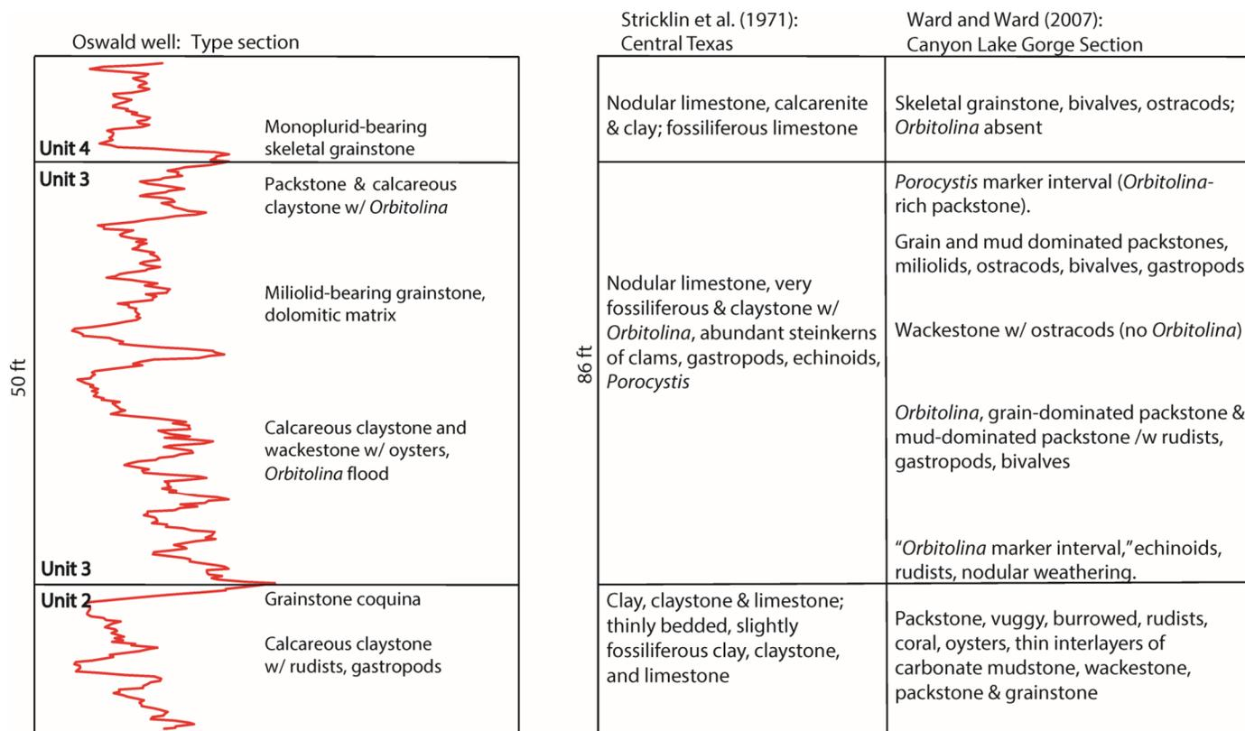
Figure 3. Oswald well type subsurface section with gamma ray log (red line) correlated to previous surface sections by Ward and Ward (2007) and Stricklin et al. (1971).
