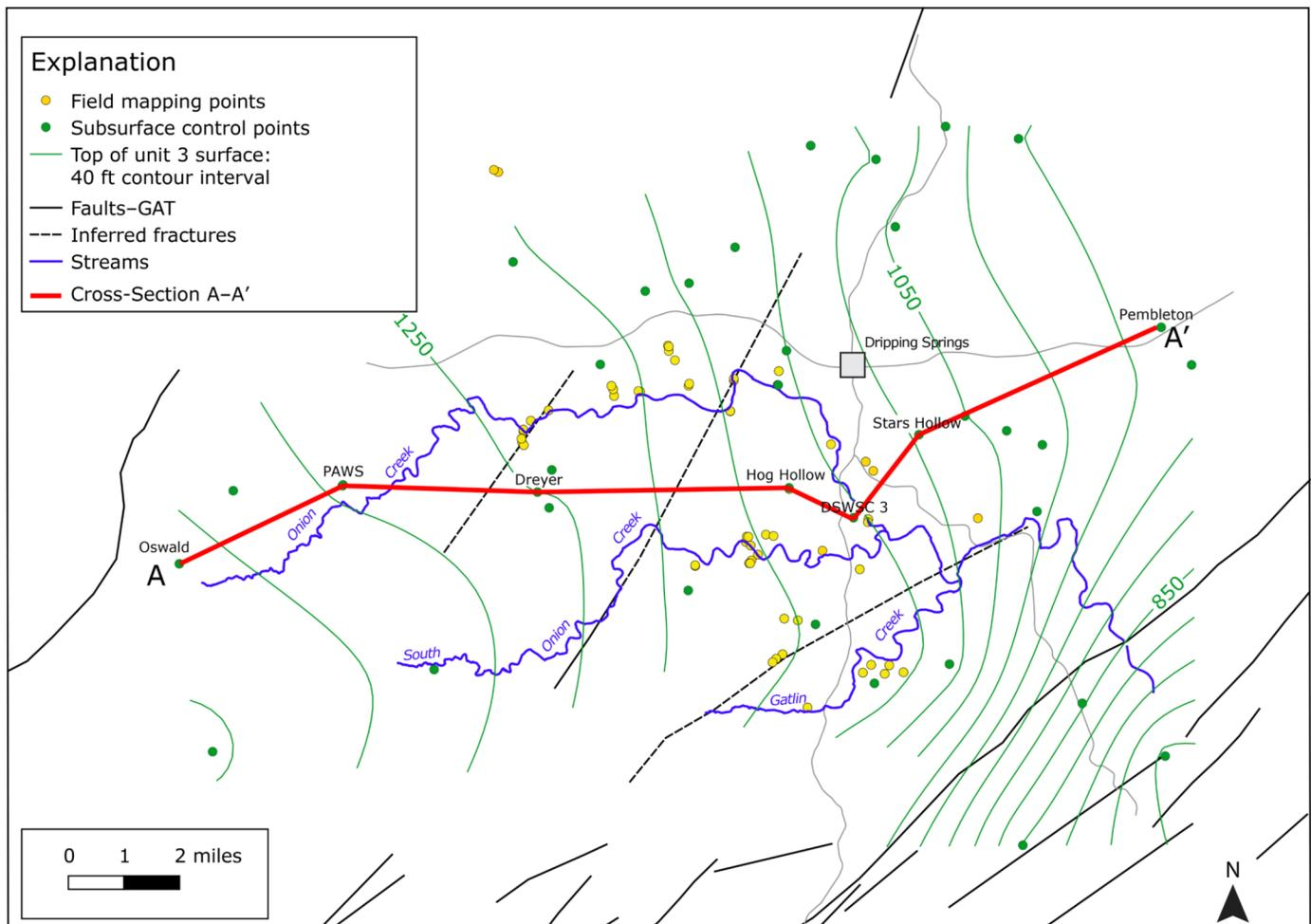
Figure 8. Structure contour map at the top of unit 3. Line A-A' denotes the path of the structural cross section presented in Figure 9.
