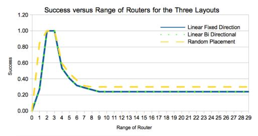
**Figure 8. Example of the Increasing Range Graph.** This figure shows the results for the range experiment with the three different kinds of layouts, each with a fixed number of rooms.
