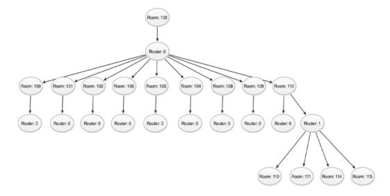
Figure 4. Example of NUWAP's navigation tree. Shows an example of the possible path decisions, which are created as the NUWAP algorithm works. This structure is also known as a tree.
