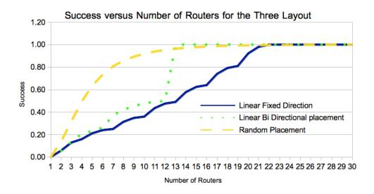
Figure 9. Example of the Increasing Density of Router's Graph. This figure shows the results for the density experiment with the three different kinds of layouts, each with a fixed range.
