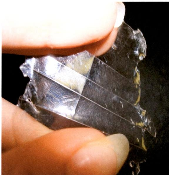
**Figure 12.** Polyimide film passes “crease test.”
