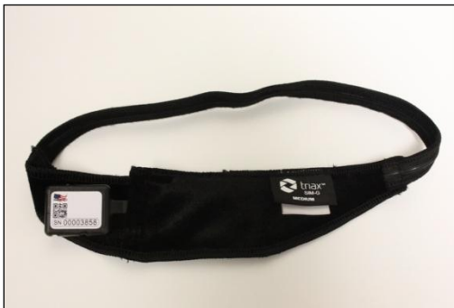
Figure 3. Back view Triax SIM-G sensor placement in custom headband
