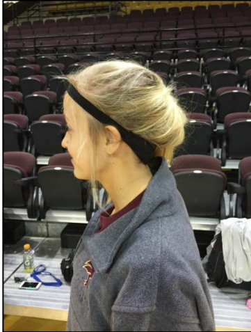
Figure 5. Correct Triax SIM-G headband placement side view
